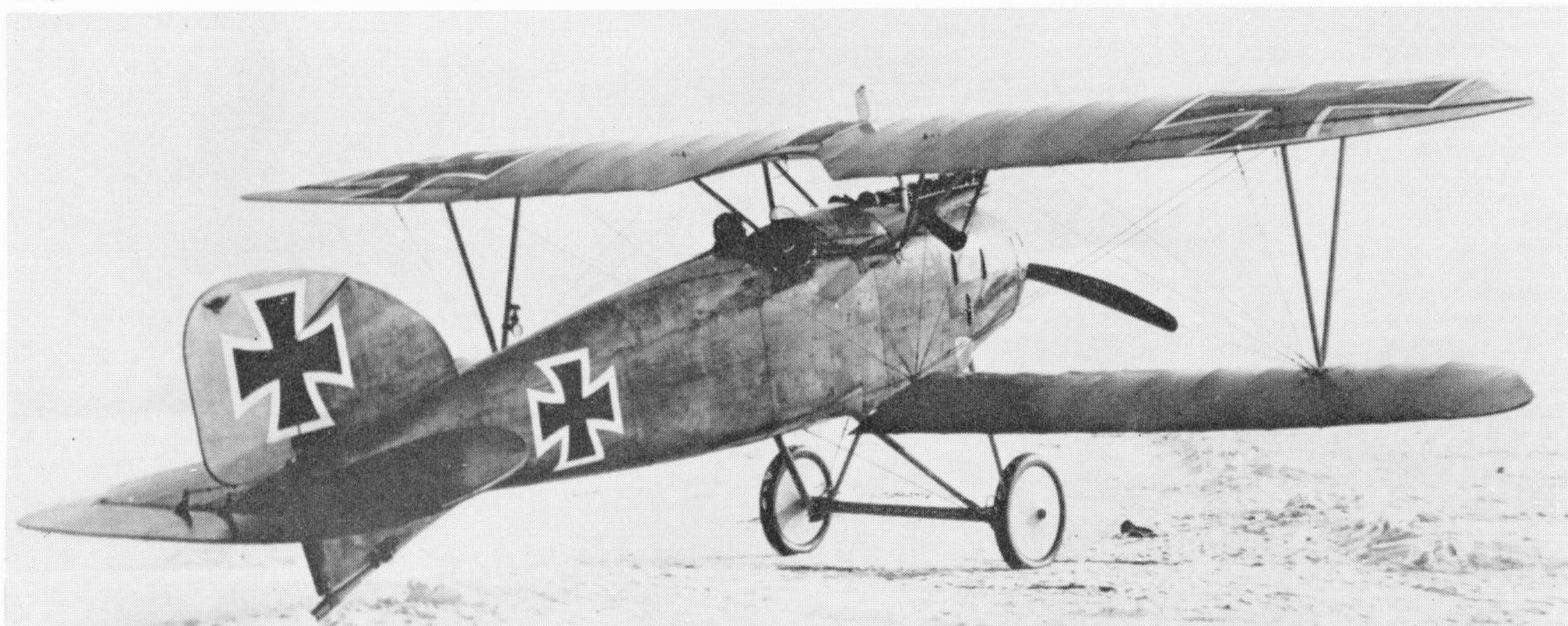
Crisply etched against the winter sky and snow covered airfield the graceful lines of the D III are well shown in this view. This is an early "ex-works" machine with centrally located radiator. (Photo: Egon Krueger)
