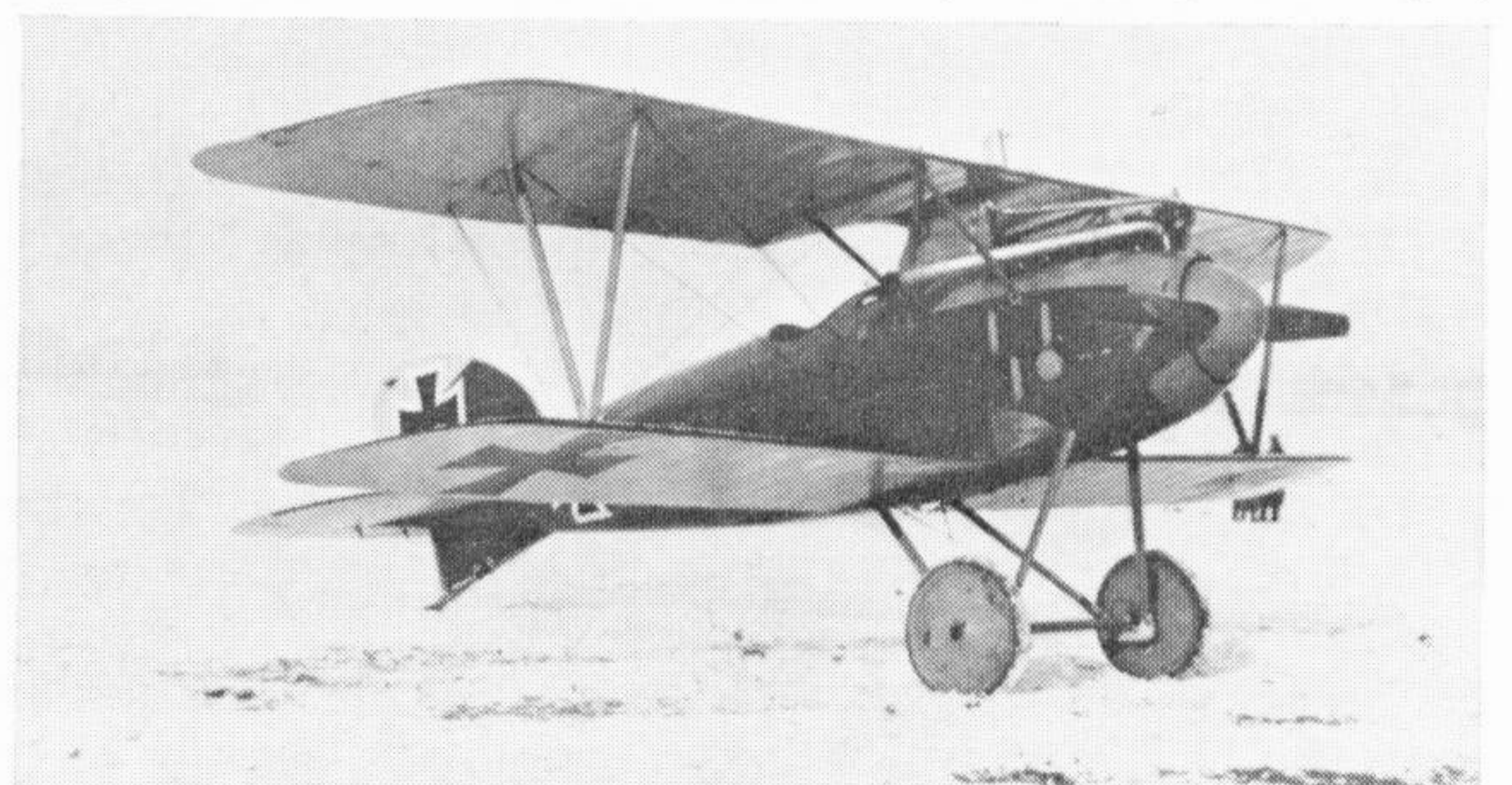
Again an early D III with centrally placed radiator: the machine belonged to Jasta 5. (Photo: Egon Krueger)
