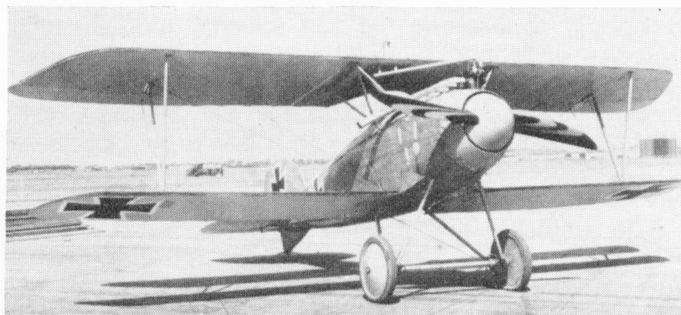
Late production Albatros D III with D V type rudder. The contrast of the aircrew laminations is clearly shown.
