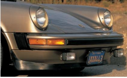
U.S. models with impact bumpers had an extra indicator lens in each side of the front bumper molding. This Weissach model also shows off its additional driving lights below the bumper.
