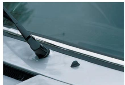
The wipers on the 911 had changed for 1968 so that they always parked in front of the driver, whether the car was left-hand or right-hand drive. Since then, the 911 designers have not been able to change the wiper arrangement significantly through the entire life of the model because of the cost of retooling.
