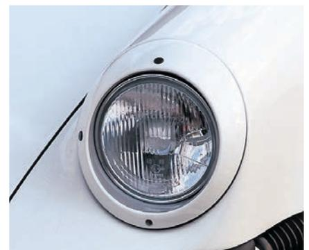
By 1986 the sealed-beam Hella headlamps fitted to U.S. cars were available with the more powerful H4 filaments.
