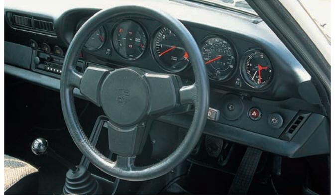
The instrument panel of the SC was little changed from the European Carrera 3.0. Points to note are the 380-millimeter steering wheel (which obscured important sections of the speedometer) and the rocker switch for the headlamp washers sited between the speedometer and the clock.
