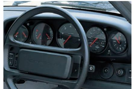
The instruments were totally updated for the new models (above). The figures and indicator needles were now backlit at night, and the oil combination gauge now contained an array of warning lights. This car does not have the air bag steering wheel. The instruments continued to be developed (below), and by 1992 the clock even carried its own complement of warning lights. The speedometer contained a shift indicator on Tiptronic models.
