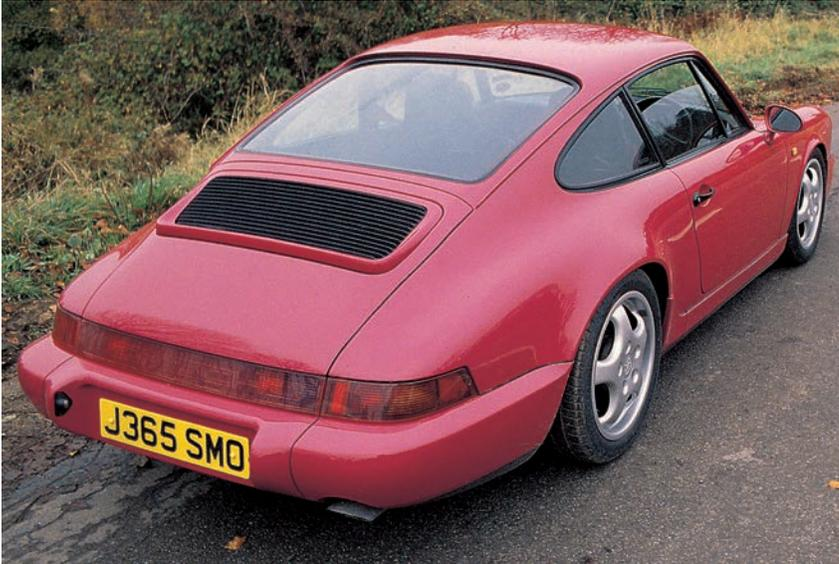
The Carrera 2 RS arrived in late 1991. With no concessions to touring comfort, this car was modified to perform. The suspension was lowered 40 millimeters from standard, instantly giving the car a purposeful stance.
