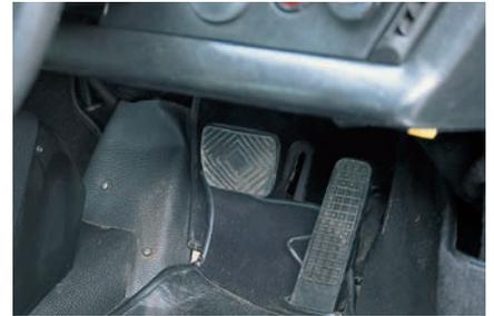
By 1979, when this car was built, the two-pedal Sportomatic transmission was available only on special order. This novel but halfway house automatic shift was deleted the following year.
