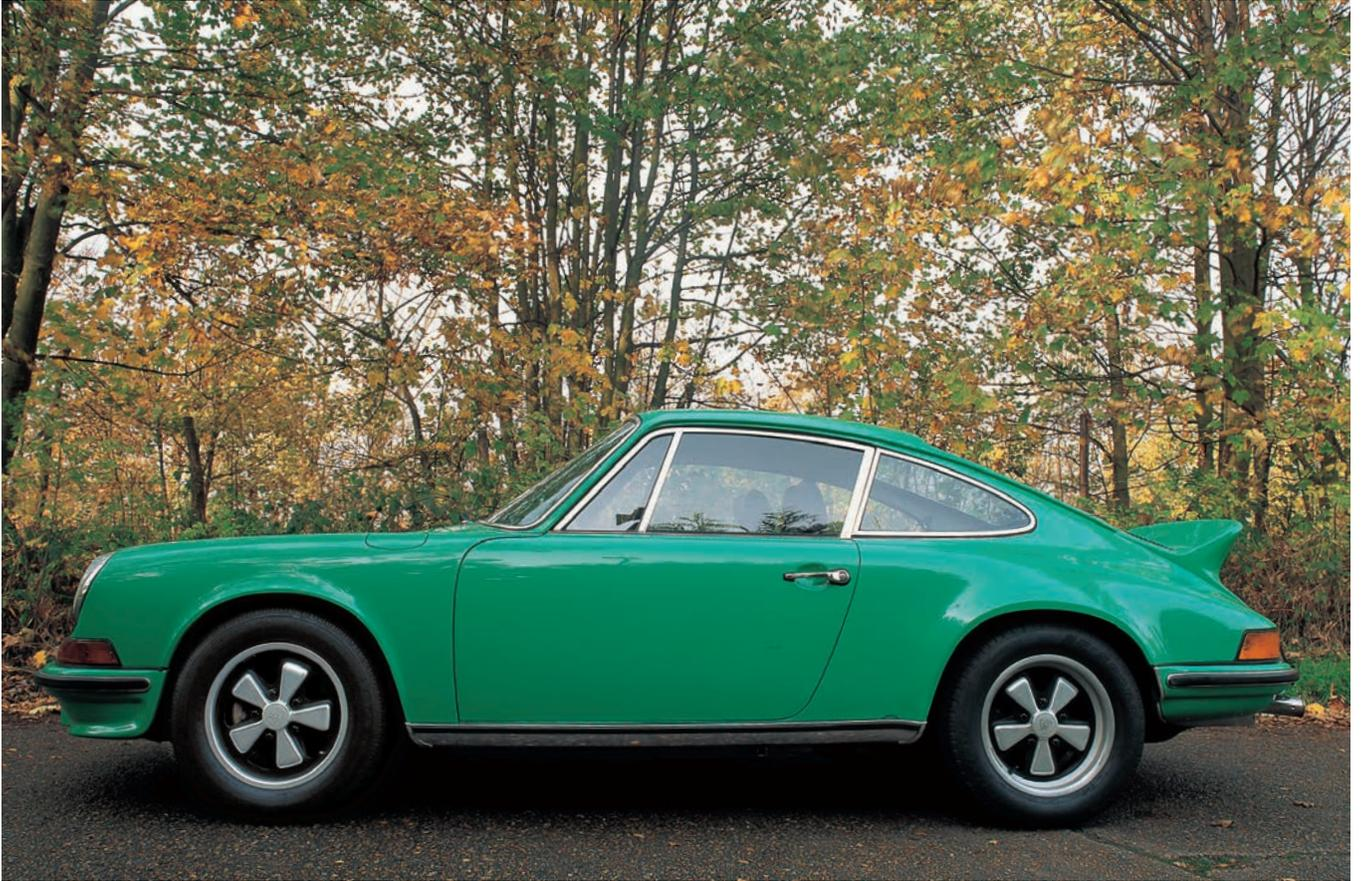
Pointing to the 911's aerodynamic future, the Carrera RS was the first model to sprout a rear spoiler, although the ducktail was actually an option.
