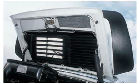
The dual functions of the tea-tray grille can be seen with the engine lid raised: The air-to-air intercooler connected into the engine intake manifold is on the left, while the air conditioning condenser on the right is mounted directly to the grille itself.
