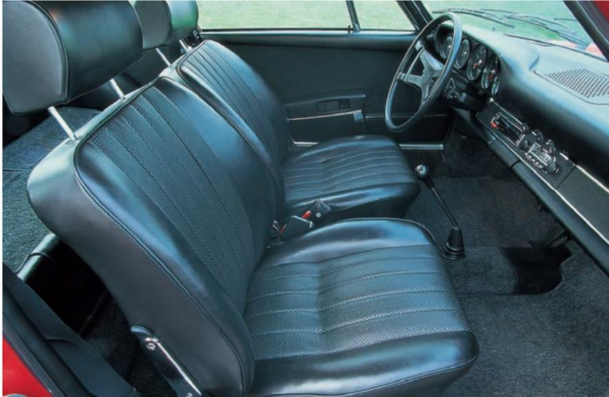
The interior of a 2.2 911 was now far removed from the early models. For the 1969 model year the lower dash had been revised to include more effective heating and ventilation controls. The ashtray was moved to the central area, the glovebox lid was further revised, and the speaker grille was now removable. From 1969, too, the seats could be tilted forward by operating a lever at the top of the seat back support, instead of down at the hinge point.
