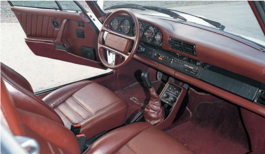
The smart Burgundy interior of this 1986 U.S. Turbo features that year's ventilation improvements, with larger face and side window vents and a new switchgear presentation.
