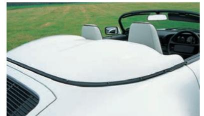
The Speedster’s large fiberglass hood cover molding hinges backward and remains in place all the time, precluding the fitting of rear seats.
