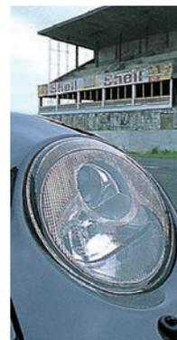
Poly-ellipsoid headlamps gave the 911 an altogether different appearance by day and by night. The reflector, rather than the glass lens, produced the required light distribution. The whole lamp unit can be removed by moving a lever inside the luggage compartment.
