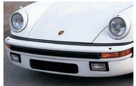
This 1986 Turbo has a replacement front air dam, complete with opening for a supplementary oil cooler and integrated mountings for driving lights.
