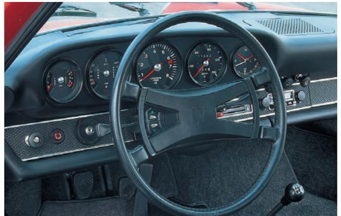
The instrument panel on a 1971 T, showing only detail changes: the hazard warning flasher button, introduced in 1970, is on the left-hand lower dash, and there are improved switches with large rubber surrounds. The labeling behind the steering wheel indicates headlamp flash and turn signal operation but is completely obscured from the driver!
