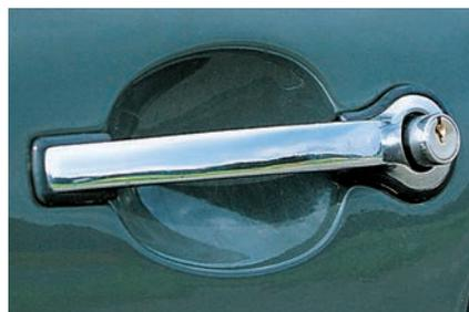
The first 911s used a simple push-button external door handle. The tooling for this door handle was changed for the 1967 model year, the later version having slightly more radius in the curvature around the button. A new handle, which protected the button and prevented the door from being accidentally opened, was introduced for 1968.
