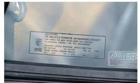
This factory label shows that the 911SC was comfortably within Californian emissions limits for hydrocarbons, carbon monoxide, and oxides of nitrogen.
