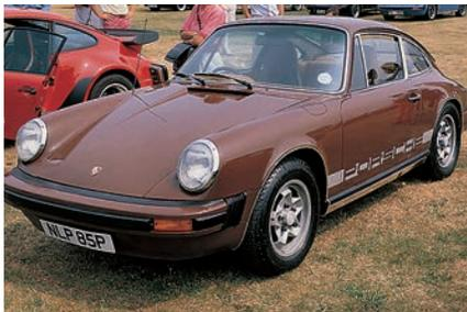
This 1976 U.K.-specification 2.7 911 shows off the ATS cookie-cutter wheels that had first appeared on the 1973 911E. The electrically operated driver's door mirror was new for the 1976 model year.
