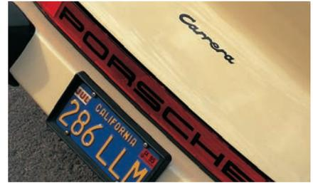
The new bumpers were neat one-piece aluminum extrusions front and rear. The rear aspect of the 911 was further changed by the addition of a full-width reflector strip between the light clusters. Possibly too flashy on some cars, it worked well on the 911. The Carrera logo had always been reserved for limited-edition high-performance models.
