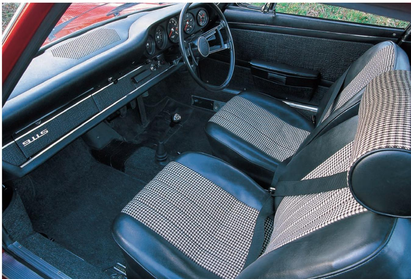
The 911 began life with a velour interior carpet, which later became the more luxurious option for the higher-spec cars like the E and S. From 1967, a cheaper material termed Perlon (with an appearance like felt) was introduced for the basic models (the 911 and the later 911 T). Until approximately the start of the 1968 model year, you could have any carpet color as long as it was dark gray.
