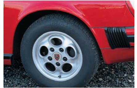
Telephone dial wheels were one feature of Porsche's attempt to update the Carrera 3.2's appearance without excessive cost. Another external difference was that the front driving lights became more integrated into the shape of the front spoiler.
