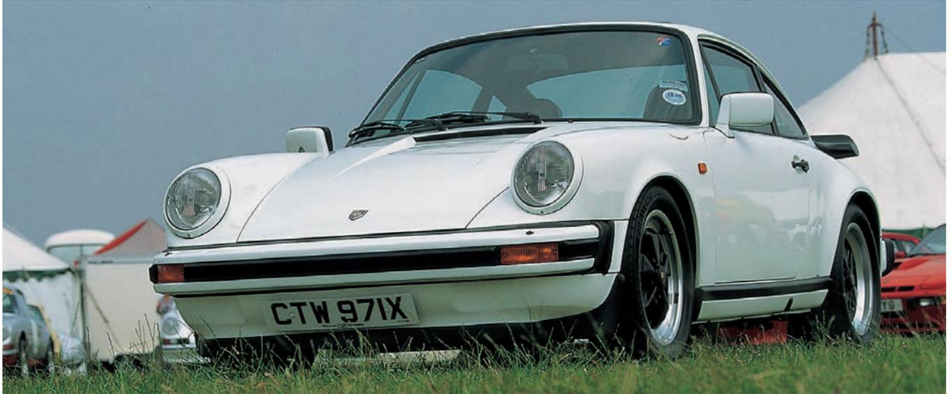
Bilstein dampers gave a firmer ride, and special Fuchs wheels with Platinum Metallic centers were used irrespective of body color. These wheels were fitted with Pirelli CN36 tires of sizes 185/70VR15 front and 215/60VR15 rear, on 6-inch and 7-inch rims, respectively. Other decorations included a passenger door mirror, electric sunroof, foglights below the front bumper, and an electric aerial with speakers fitted in the doors and on the rear shelf.
