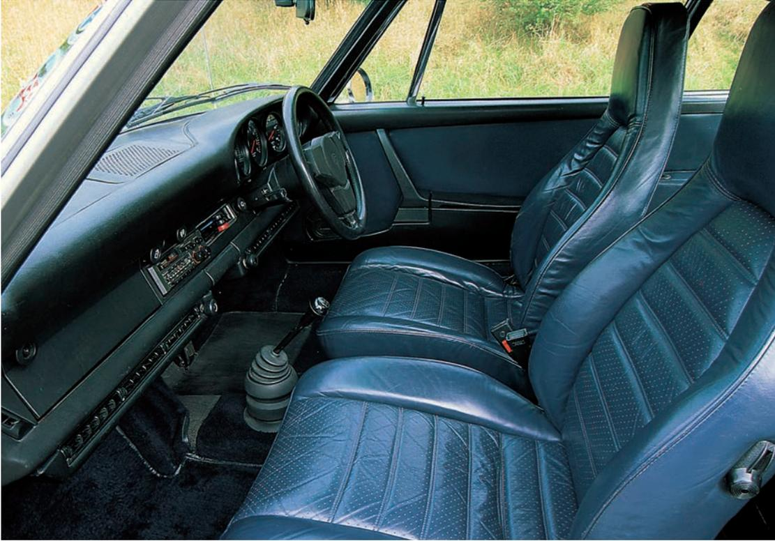
There were new seats for 1974, featuring more thigh support and integral head restraints. Although rear passengers found it more difficult to see ahead, getting in the back was easier because the releases on the seat backs were more accessible. When air conditioning was fitted, as here, the outlets ran across the lower dash area, integrating well with the existing design but reducing knee room.
