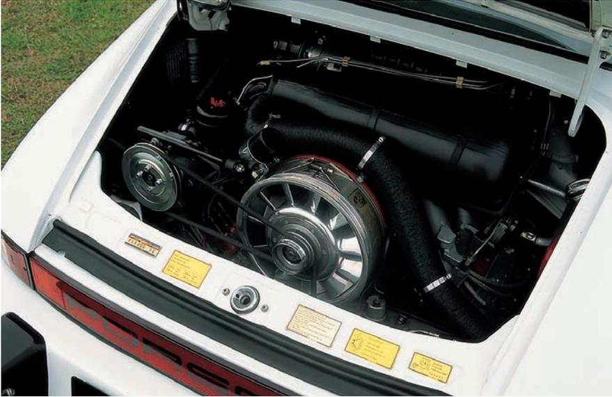
Rest-of-the-World models retained the air-injection pump, seen here on the left of this 1982 engine compartment. The air filter for the pump can be seen behind it, with a red wing nut on top. After a brief period when a five-blade cooling fan had been used, the SC returned to an 11-blade version. This fan and many of the fittings around the engine have been highly polished, to good effect.
