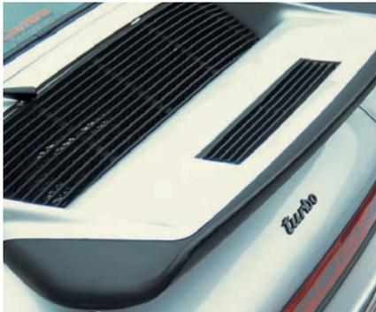
The whaletail spoiler was derived from the design used on the 1973–1974 3-litre RS. The 1975 model has a small secondary engine cooling grille, a style that was used only for one year.
