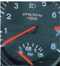
The Turbo's power was nothing special at low revs, but then it arrived all in a rush, that little needle flicking around the dial as the car surged forward. The boost gauge did not become standard on Turbos until the 1977 model year.
