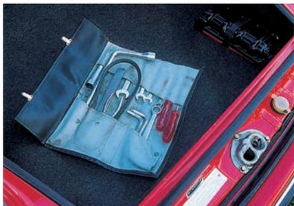
The 1968 S had a soft-grain finish to its tool bag, but from 1969 the tool bag vinyl changed to a basketweave. The chassis number plate is seen to the left of the latch, with the windshield washer filler on the right. The battery at top right has the correct rubber strap and plastic cover.
