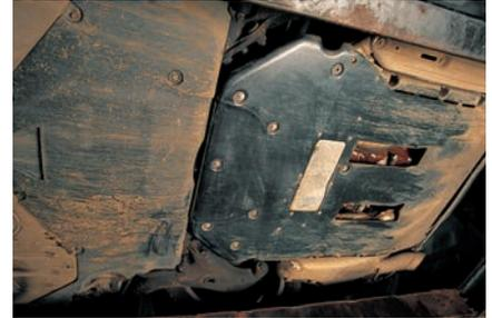
Great attention was paid to the aerodynamics of the Carrera 4. A full-length undertray to the rear of the engine not only helped airflow but also contributed to lower noise levels. Note the NACA duct below the gearbox area.
