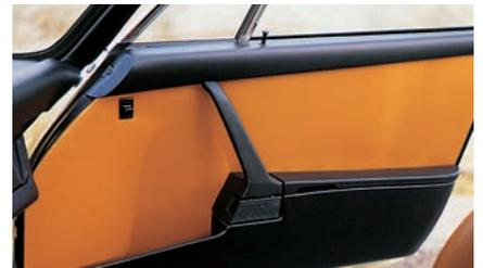
The door trim on the 1974 models received another revision. The rear compartment was now deeper and had a conventionally hinged top lid to replace the elastic bungee sprung "clamshell" of the previous design.
