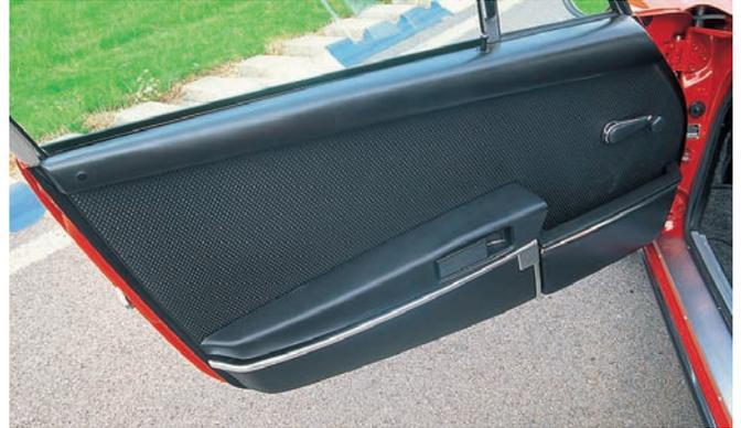
New door trims were introduced for the 2.2 models. Their features were rigid storage pockets (the rear one hinged outward) and a recessed door handle lever—much safer than the previous push-button release.
