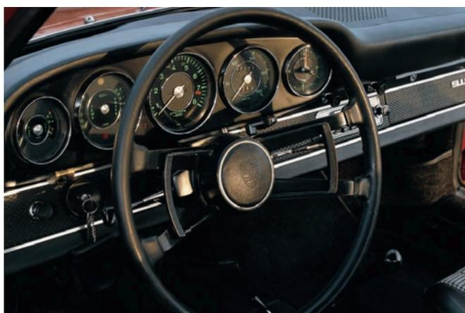
The dashboard began to change for the 1967 model year. The S was given a leather-rimmed steering wheel and basketweave vinyl trim on the lower dash area, but the green instrument markings remained. Note also the new glove compartment lid with "square" 911S lettering.
