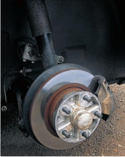
The front suspension of this 1965 car shows the MacPherson strut and, behind it, the actuating lever for the 13-millimeter anti-roll bar—an early attempt to stiffen the front and delay the onset of oversteer. Brake discs were solid and at the front used the M-type cast-iron caliper.
