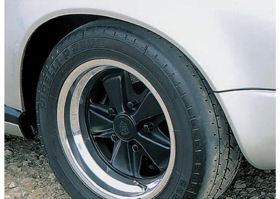
By 1975, the Fuchs forged-alloy wheel had become the required fitting. From the early narrow examples, changes had centered on increasing the wheel width and improving the finish of the rim. The RS had introduced different front/rear wheel sizes, and this practice was carried over to the later 2.7 Carreras. This is a rear 7Jx15 wheel with a nonstandard 225/50 tire.
