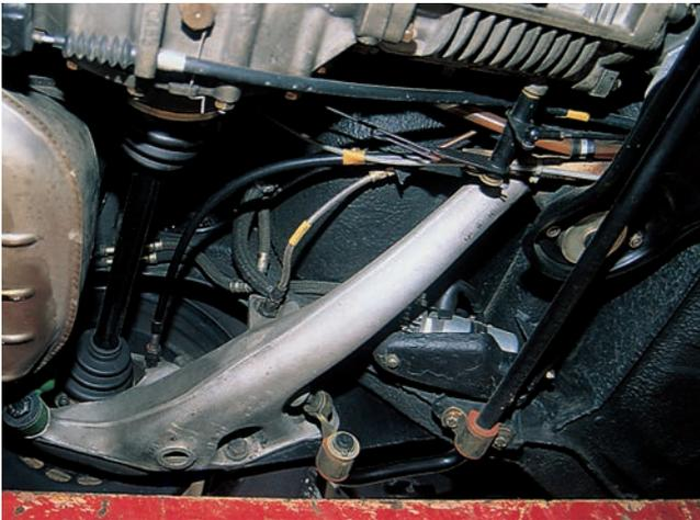
This underside view shows the forged semi-trailing arms (with embossed build date) that replaced the more flexible fabricated steel units in 1974. Other points of interest are the glimpse of the green Bilstein gas shock absorber, the fuel pump tucked away behind and above it, and the delicate mounting for the anti-roll bar.
