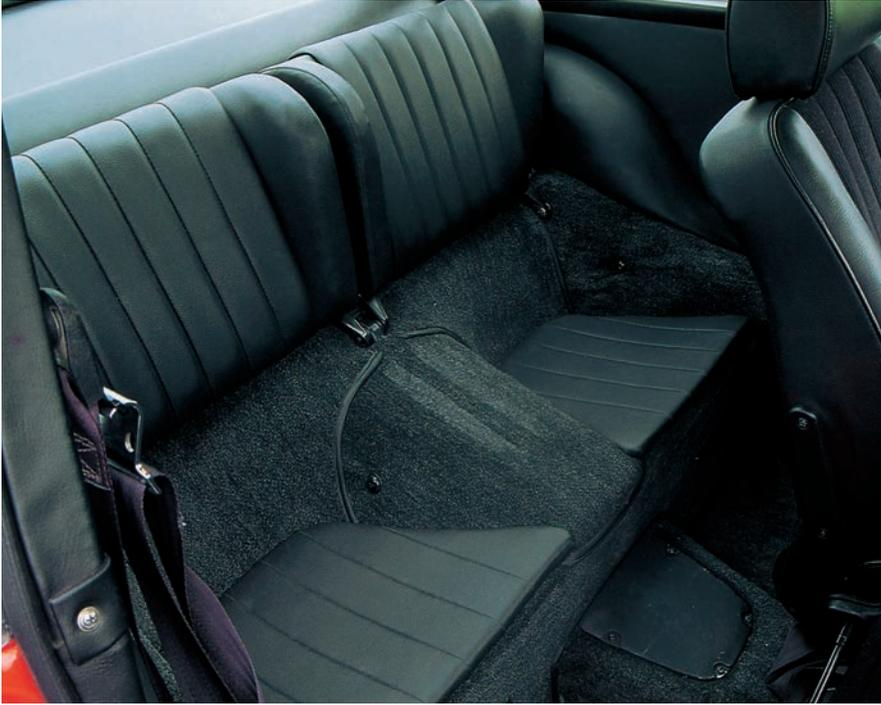
The interior of the 2.4E reflects a fashion in the 1970s for minimal chromework. An interesting point is the blank cover plate on the central tunnel. On early models (to 1967) a petrol heater was standard, but then became an option on left-hand-drive cars until 1973. Intake air for this device would have been drawn through an open grille mounted in this position.
