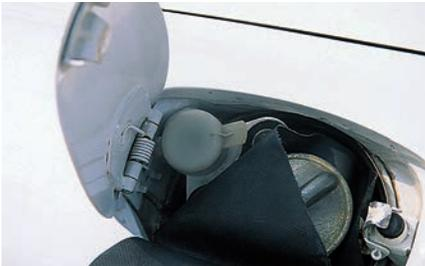
The fuel filler flap has hardly changed throughout the life of the 911. The canvas flap shields the paintwork from drips, while the washer bottle filler is to the left.
