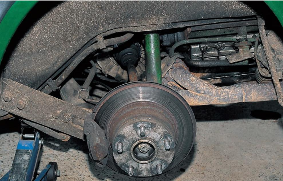
A mud-splattered 1975 Turbo rear end shows off its Bilstein shock absorber and the engine's lower valve covers newly strengthened by added ribbing. The brake calipers look far too humble for the performance of the car. The Turbo did not receive suitably powerful brakes until the 1978 model year.
