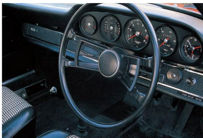
The markings of the dials changed from green to white for the 1968 model year, and chrome trim virtually disappeared from the dashboard. Interesting details include the large switch under the clock for the optional sunroof and the heavy grain lower dash that was also new for the 1968 model year.
