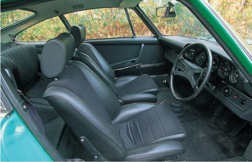
The interior of the M472 was equipped to the level of the production S model. Note the sports seats and the large gear lever boot—a new feature for 1973.
