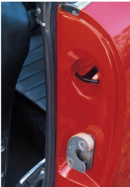
The engine lid release on the 911 is to be found on the left-hand B pillar. This feature is not so convenient for right-hand drive.
