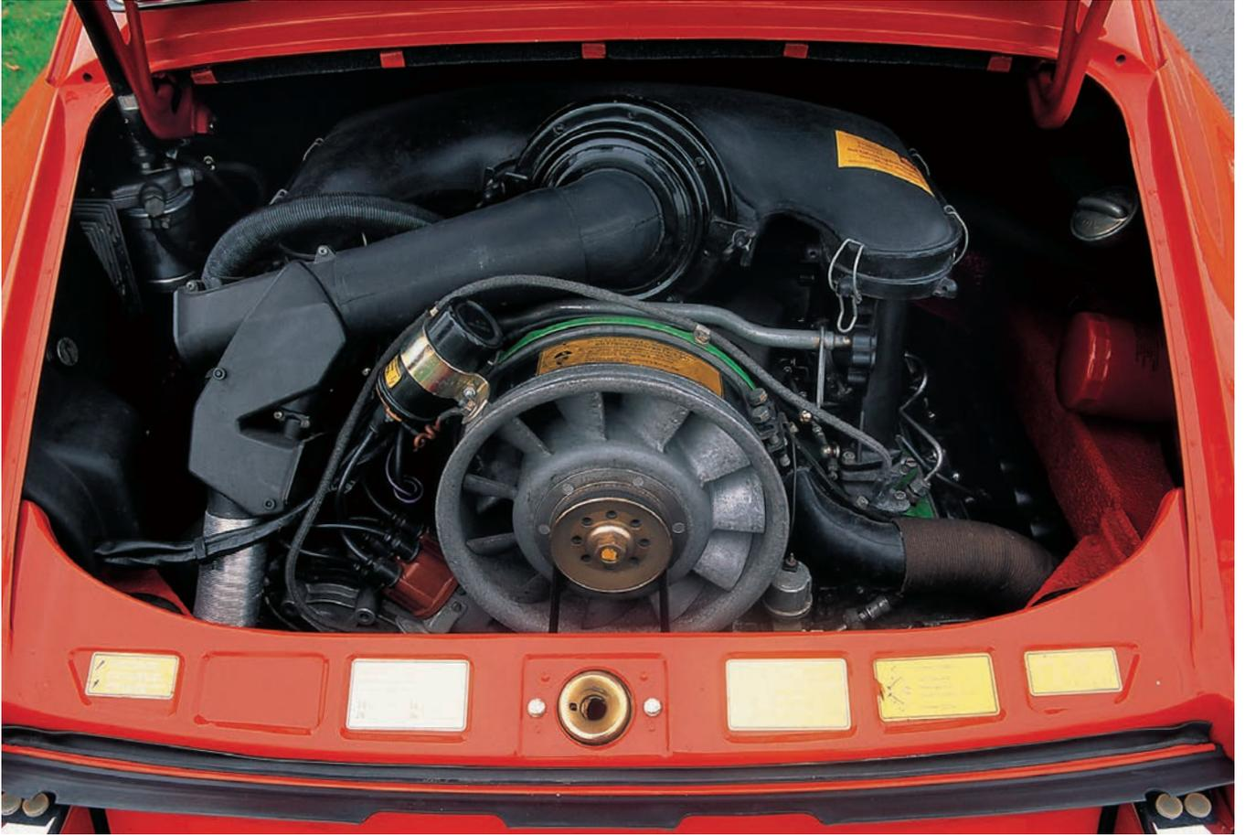
For the 2.4 models the engine air intake ducting was revised to incorporate a cold-start flap, with the opening moved from the right-hand to the left-hand side of the engine compartment. When the engine was cold, the flap prevented ambient air entering the intake ducting, and warm air was drawn from around the left-hand heat exchanger.
