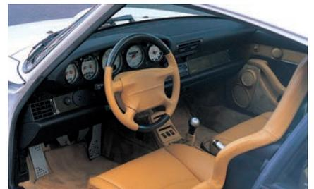
This U.S. model Turbo S interior was a product of the factory’s Exclusive customizing program. Special features include the carbon-fiber trim panels, Exclusive steering wheel, matching leather-trimmed Recaro bucket seats, drilled pedals, and reverse-painted instruments.
