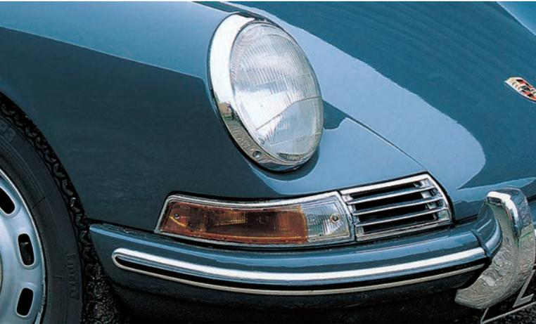
The earliest style of horn grille was made of chrome-plated brass and mounted with four screws (above), but a cheaper design for the 1967 model year was secured by only two screws (below). Both cars have the European-specification Bosch asymmetric (nonsealed-beam) headlights used until the end of the 1967 model year, but the bumper styles differ because the later car, without over-riders, has the wide rubber insert that was a new feature of the S.
