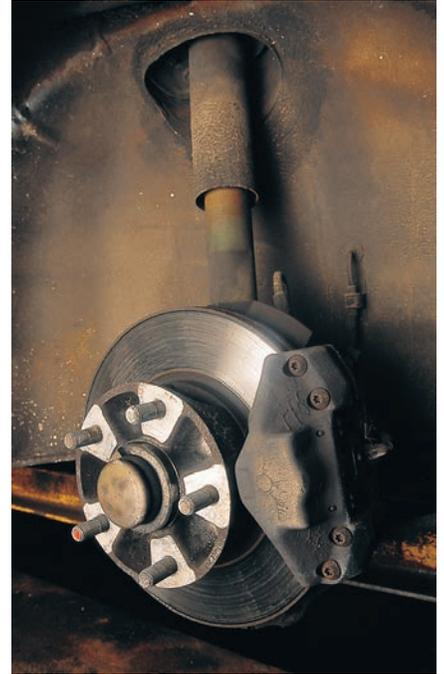
Club Sports had (green) Bilstein gas dampers as standard. All Carrera 3.2s were given larger versions of the familiar A-type cast-iron calipers and the brake discs were thicker (at 24 millimeters) than those on the SC.
