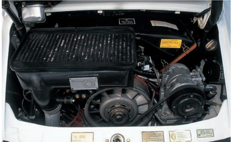
The busy engine compartment of a 1986 U.S. Turbo: The horizontal radiator is the air-to-air intercooler, placed after the turbocharger in the high-pressure duct to the intake plenum. The intercooler reduces the temperature of the charge air and noticeably improves engine power as a result.
