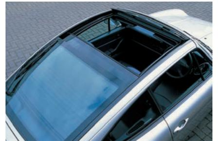
The Targa's roof was thermally insulated and filtered ultra-violet light. The elegance of the design is evident, particularly in the absence of the old rain gutters of the coupe and the new form of the rear side window. The opening glass slid back under the rear window at the touch of a switch to provide open-air motoring. The panel in front of the sliding roof opened forward to prevent wind buffeting inside the car.
