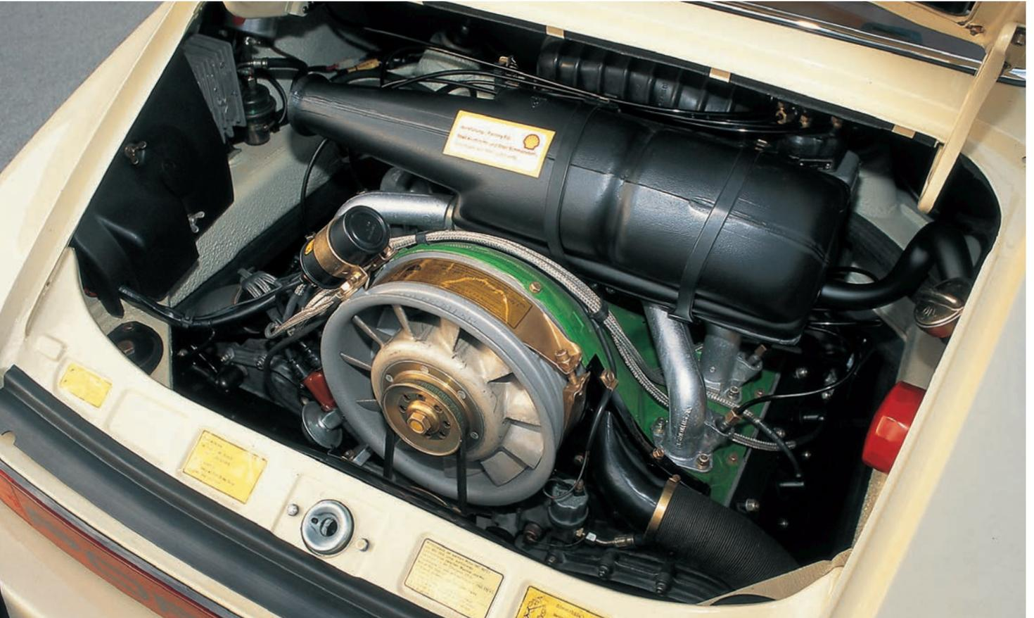
While European 1974 Carreras used the engine from the previous year's RS, U.S. models adopted that market's S engine and Bosch K-Jetronic injection. With just 175-brake horsepower, the U.S. Carreras were at a significant power disadvantage against the 210-brake horsepower Carreras offered in most other markets.
