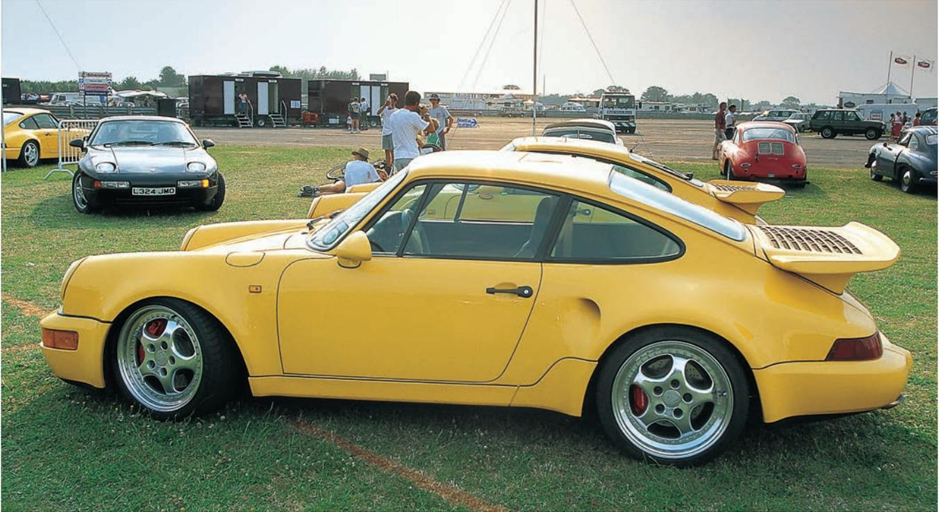
The 1987 Turbo Slant-Nose derived its front profile from the 935 racer, but pop-up headlamps were added. Early customized Slant-Nose cars lacked pop-up headlamps, having the lights mounted below the bumper line.
