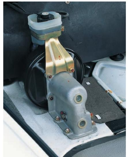
The addition of a brake servo was a significant improvement for the 911 SC. Its effect was most noticeable around town when the discs were cold. The bulk of the assembly seriously reduced the usefulness of the luggage compartment.
