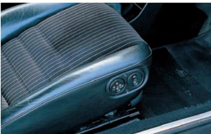
The seats on the Carrera 3.2 have electric adjustment for height, cushion angle, and recline, with this control panel set on the side of the cushion.
