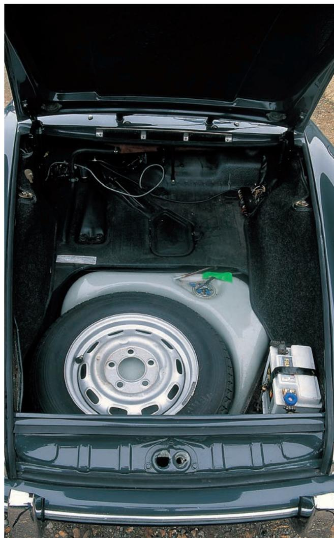
The luggage compartment, seen here on a 1965 model with the central piece of carpet removed, housed the spare wheel and the fuel tank, both of which were recessed between the front wheels to allow a useful volume on top for personal belongings. Note the fuse block fitted at the top right. The battery is attached by a later fitting, the original rubber strap and plastic cover no doubt having disappeared long ago.
