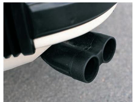
Twin exhaust tailpipes were first seen on the 1983 Turbos when the wastegate exhaust was taken directly to atmosphere.
