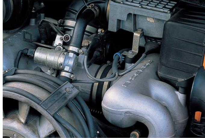
Digital Motor Electronics came to the 911 for the 1984 model year, improving performance and reducing fuel consumption by 10 percent.
