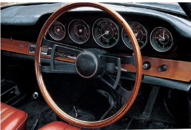
Right from the start, the dashboard featured the 911 trademark of five dials reducing in size either side of a central rev counter. The colors of the wood veneer (used for the 1965–66 model years) and the green features on the dials (1965–67 model years) complement each other and are accented by chrome bezels.
