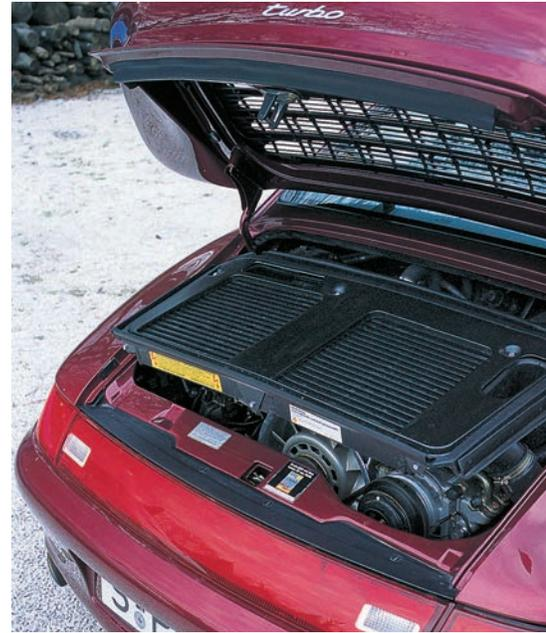
There is an engine under there somewhere! Twin air-to-air intercoolers dominated the engine compartment of the Turbo.
