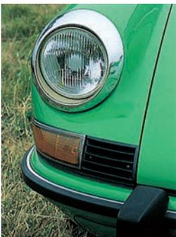
This T has the more pronounced chromed headlamp flange that goes with the sealed-beam units fitted to U.S. cars. These headlamps were unpopular, as shown by this car having the more powerful Lucas H4 units retrofitted. Also visible is the large elastomer over-rider used only in 1973.
