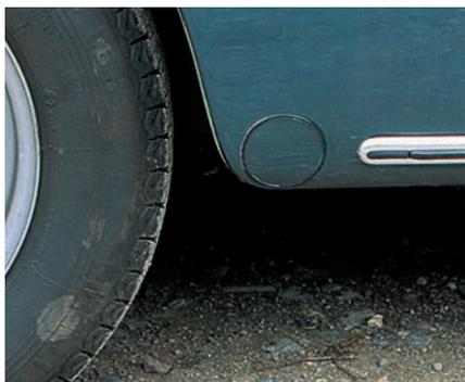
The earliest 911s had pencil-thin rubbing strips on the sills, and the circular cover that gives access to the rear torsion bar was completely exposed.
