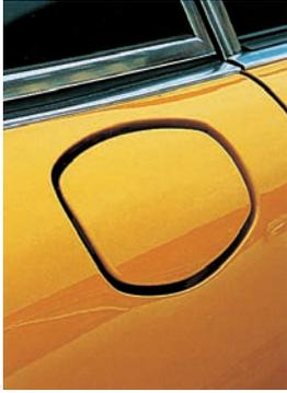
A 1972 model 2.4 can be identified by the oil filler flap on the right-hand rear wing—where it remained for only one year. Placing the oil tank within the wheelbase helped the handling, but this arrangement proved to be impractical because filling station attendants sometimes put petrol in the oil tank.
