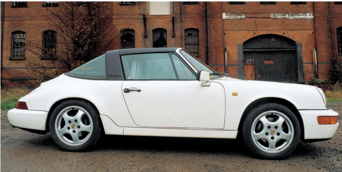
Ian King's Carrera 4 Targa shows the new design of front bumper and side skirt, with a much more squared-off lower edge to the 911's classic curves. This car is fitted with five-spoke Cup Design wheels.
