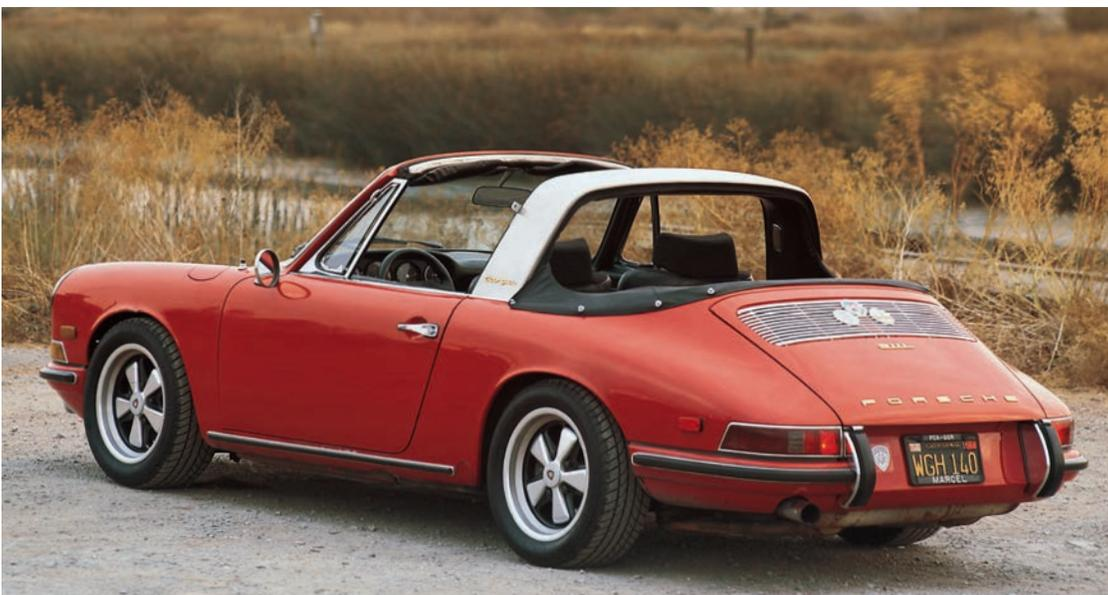
This detail of a 1968 Targa shows the "soft-window" rear screen stowed and the tonneau in place. The position of the interior light in the roll-over hoop and the gold-anodized Targa script can be seen.
