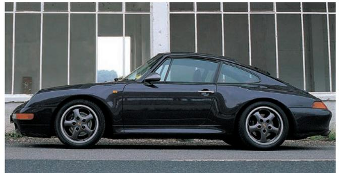
This is a 1997 Carrera S, which combined the Turbo chassis and rear-wheel-drive transmission to produce a supremely confident package.
