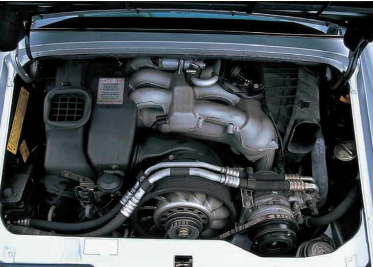
The 3.6-liter engine gained another 22-brake horsepower. Despite weighing an extra 20 kilograms, the 993 delivered better all-round performance than the 964. The improved 1996 models (left) used a Varioram induction system and larger valves to produce 285-brake horsepower from the last full-scale production version of the air-cooled boxer "six."
