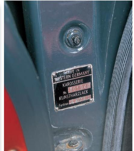
The chassis number on early models is found on the left-hand door pillar. Also shown on the plate is the paint code (Farbton) 6401, Slate Gray.
