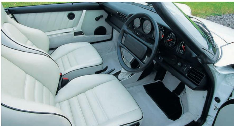
This Speedster interior shows manual window winders and the smaller sun visors used to suit the lower windscreen.
