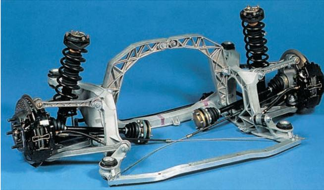
Porsche's lightweight-stable-agile (LSA) design provided the 993 with new multi-link rear suspension—a major change under the surface.
