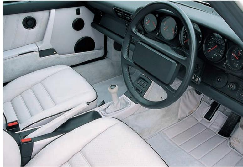
Apart from new trim choices and door loudspeakers, the only significant change in this Carrera 4's interior architecture compared with the old Carrera 3.2 is the higher central tunnel necessary for the four-wheel-drive system.
