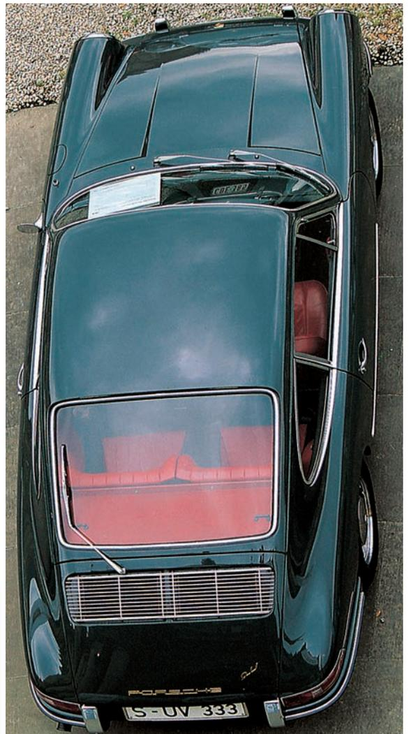
The clean lines of the Porsche factory’s own 1964 911 coupe. The first 911s had minimal flaring to their wings, giving the cars a clean aerodynamic shape. Evident in this view is the Durant driver’s door mirror of 356 vintage.
