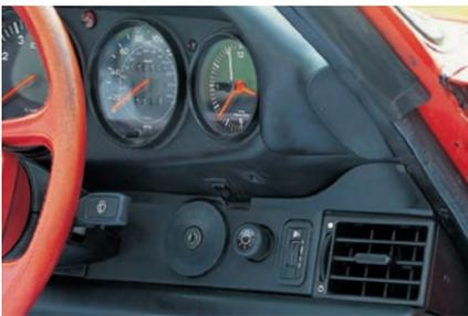
The ventilation system was improved again for the 1986 model year, with larger face level and side window vents. The headlamp level adjustment was introduced for 1987. The nonstandard slot next to the sunroof rocker switch is the keyhole for an aftermarket engine immobilizer.
