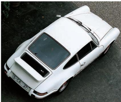
Just more than half of the 109 3-liter Carrera RS models built were roadgoing variants (below). This version used the heavier production bodysell and featured a new whaletail rear spoiler. The M471 Sport model (above) is notable for its elementary equipment specification in the pursuit of performance.
