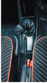
control next to the handbrake. In the absence of electric seat adjustment, the manual levers fore and aft movement are also grouped near the handbrake. Note the shift pattern of the C50 gearbox.
