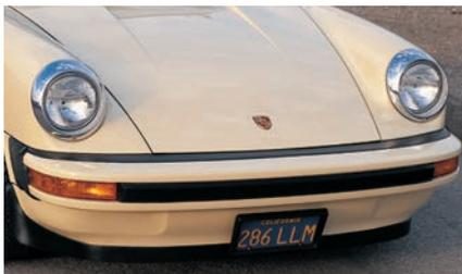
By a superbly clever mix of design and function, Porsche's stylists turned a potentially disfiguring legal requirement for energy-absorbing bumpers into an image-enhancing feature. Just visible here is the flexible lip extension to the new front spoiler, an important detail that improved the aerodynamic balance of the car when the rear ducktail was fitted.
