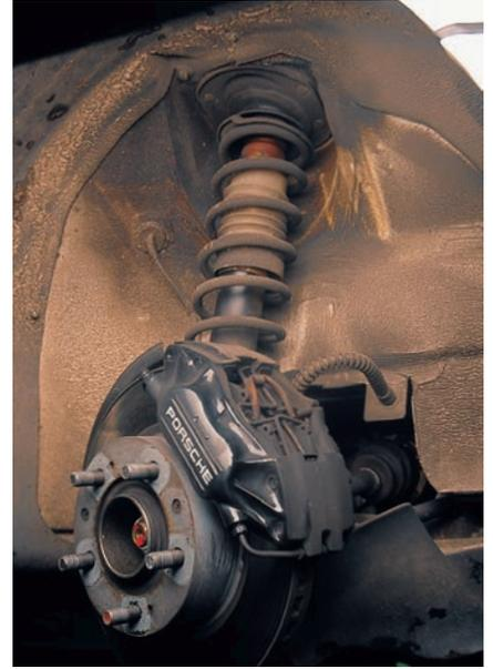
The front suspension discarded the 911's time-honored torsion bars and adopted conventional coil springs over the shock absorbers. A significant redesign of the front chassis was necessary to accommodate four-wheel drive.
