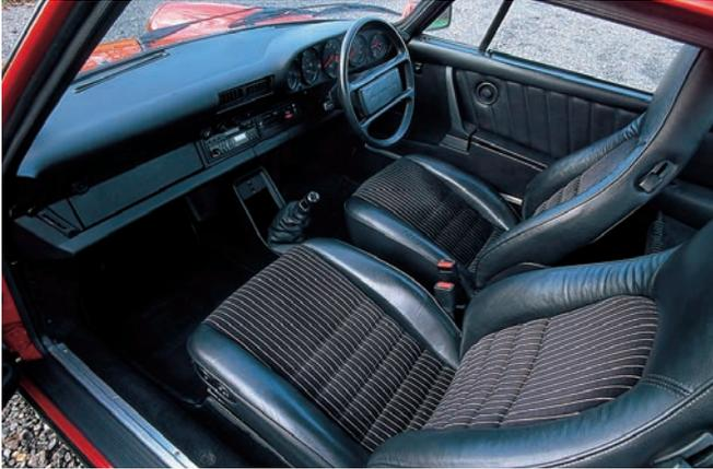
The pinstripe style is one of Porsche's best interiors, being both practical and smart. New features for the 1985 model year, one year after the Carrera 3.2's introduction, included a four-spoke steering wheel, taller seat backrests, and seat release catches on both sides of the backrests.
