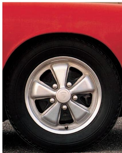
The classic Fuchs forged-alloy wheel was introduced on the 1967 model year 911S, but the narrow rim width of 4.5 inches dismayed *Car and Driver* magazine. Note the restrained use of black paint on these early wheels and the elegance of the non-spoilered front profile.
