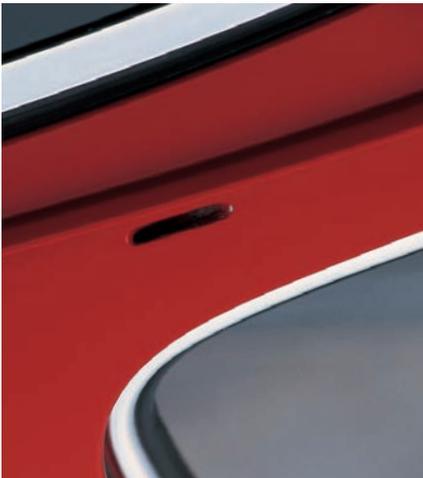
A feature of O- and A-program model 5 with a sunroof fitted at the factory was drain slots in the roof adjacent to the rear window.
