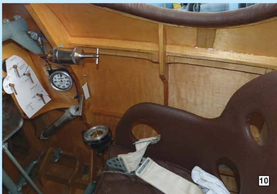
7. Looking forward is the control column and ammunition magazine. The instrument at the top of the photograph is the tachometer pressurising pump. The instrument next to the switch board is the fuel gauge
