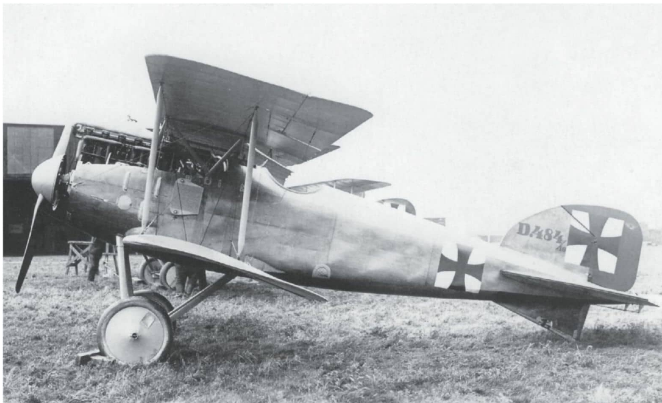
Above: An interesting photograph of Albatros D.II 484/16 with its metal nose panel and cowling missing. 484/16 was one of the first shared batch of D.Is and D.IIs ordered in early July 1916
