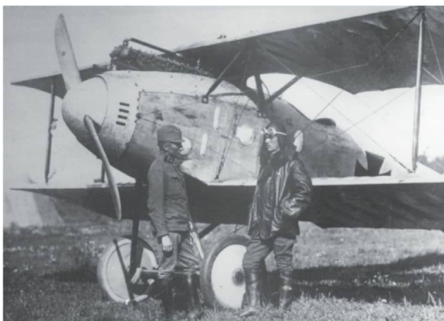
Left: Albatros D.II (OEF) 53.14 in the field. Note the milled pattern of the natural metal cowlings. The four vents visible on the nose panel appear to be unique to 53.14. It's not known if the pattern is repeated on the starboard side
