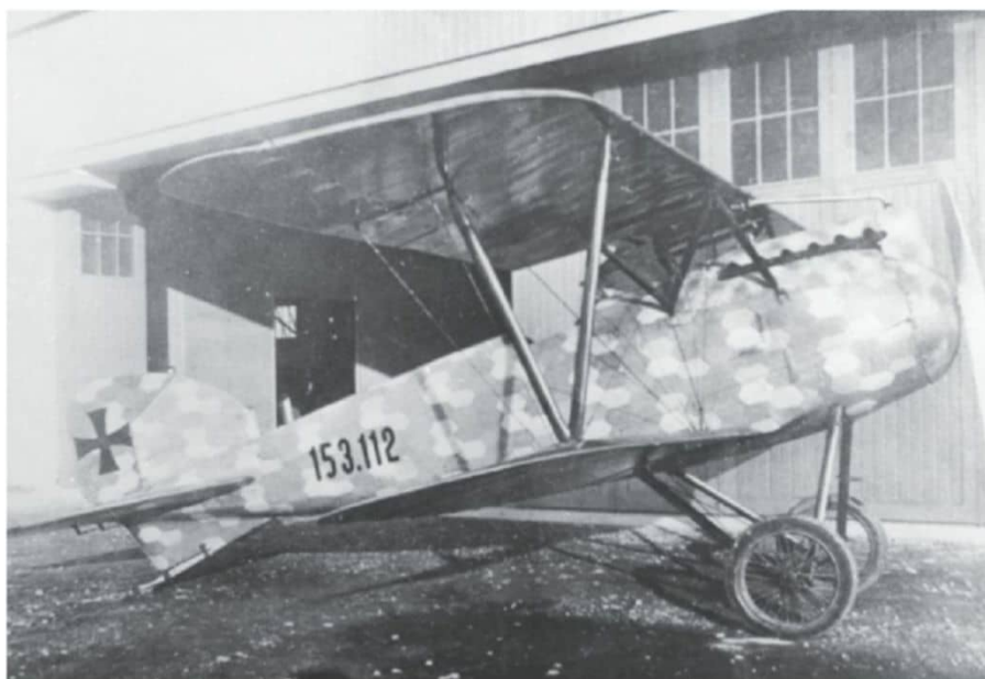
Left: Albatros D.III (OEF) 153.112 was the first OEF production Albatros to have a rounded nose. The aircraft also has an interesting experimental hexagon camouflage pattern which would have been hand painted
