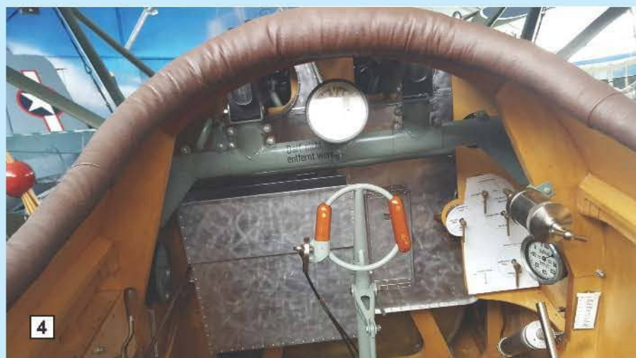
2. Looking down at towards the base of the control column. At the top of the picture is the rudder bar. The cables attached to the control column on the right work the elevator
