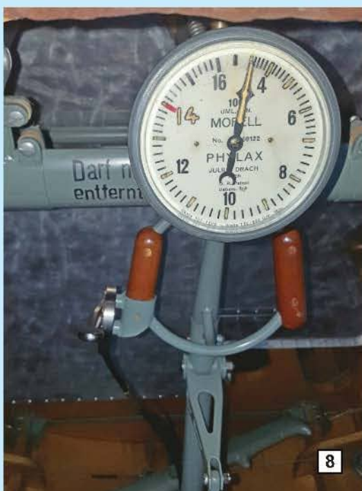
6. A nice shot clearly showing the control column and rudder bar. Note the circular shape of the hand grip that was present on the early Albatros D-types. This would evolve to become more angular in later Albatroses
