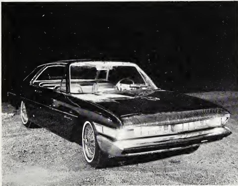
Details of the Sceptre prototype. Note side lighting, cut-down hood/deck assemblies, low frontal profile, flush side contours, 'slide rule' speedometer and adjustable instrument pods, chrome-mylar upholstery, transverse taillights.
