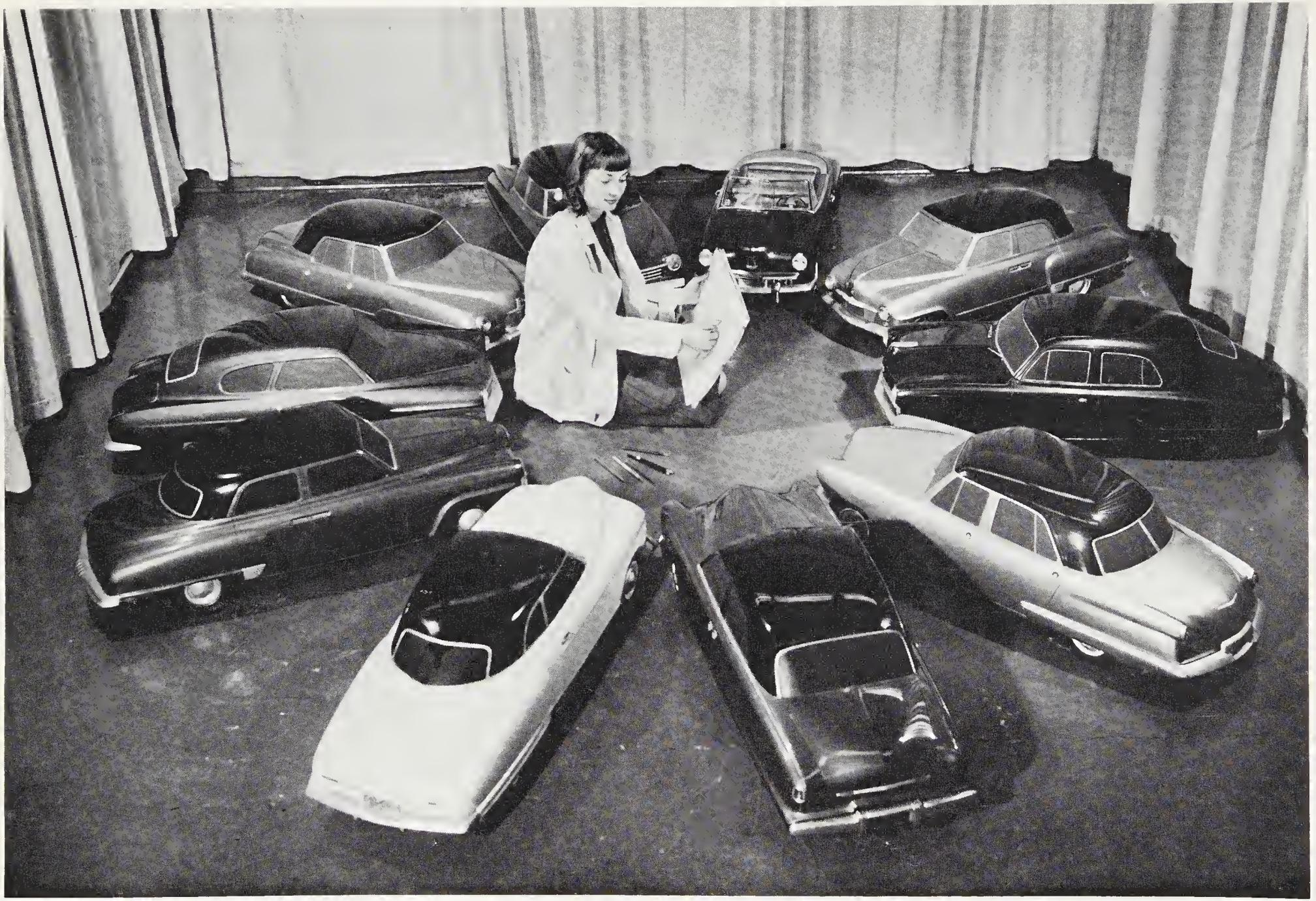
Quarter-scale plastic models, some designed as suggestions for 1947. Bob Koto designed two in foreground. Koto says most of these were actually wider than the Exner design, save the convertible, the car to the right of it, and the cars in the foreground, which were Exner-model modifications.
