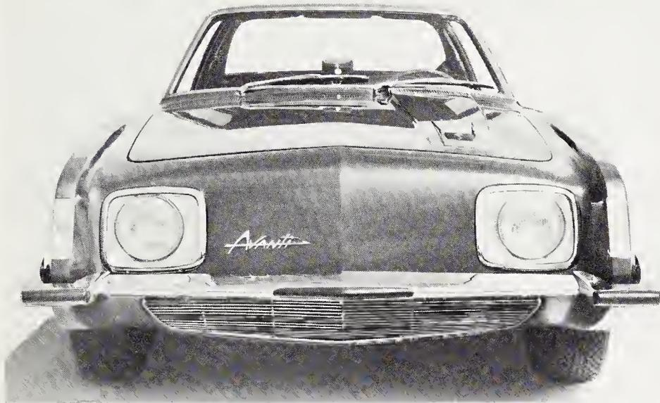
New radiator grille appeared in August 1963 with square-bezel head lamps, but some round-head-lamp models were also fitted with the grille.
