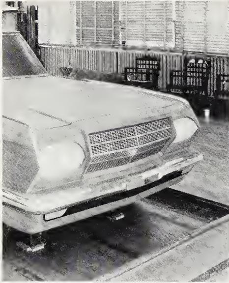
Halogen or glass-covered head lamps figured in 1964 plans, but ultimately conventional sealed beam lamps were fitted.
