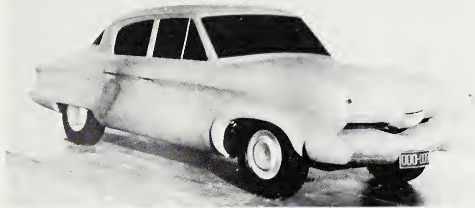
Scale model proposed for 1950 incorporated Loewy spinner, floating wing between fenders. Contoured bumper proved too expensive to produce.
