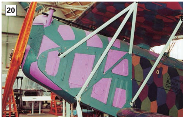
20: Further view of the nose section, showing engine bay louvres and the anchor points, top and bottom, for the cabane struts.
