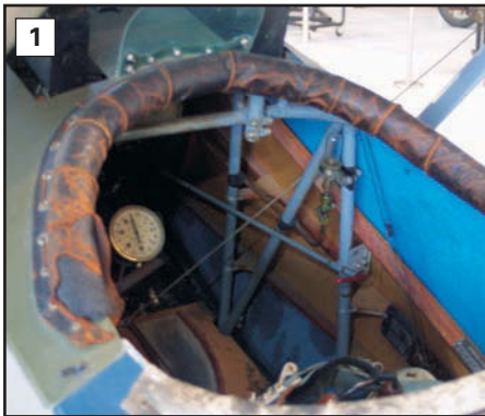
1: Cockpit rim, showing leather coaming and binding.
