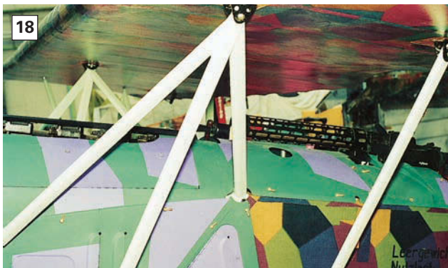
17: Further view of the cabane struts. These look quite slim by the standards of the era.
