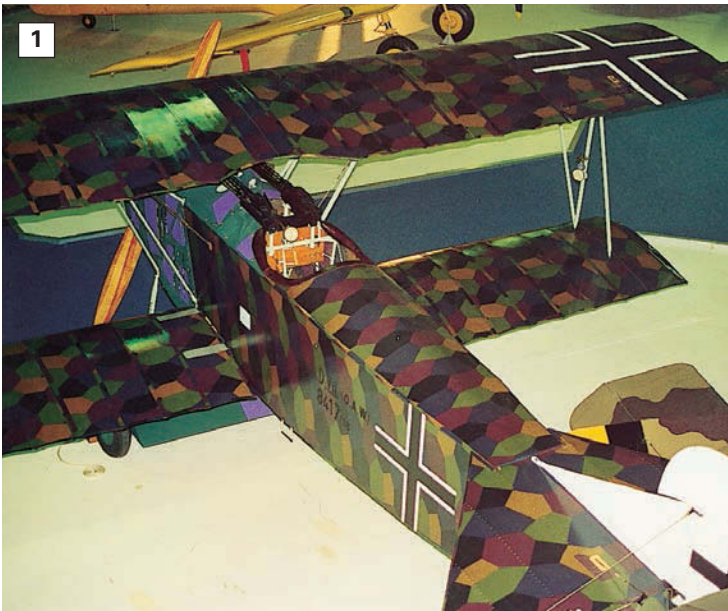
1-6: Some general views of the RAF Museum's machine which features five-colour pattern lozenge camouflage scheme. The 'axle wing' is not lozenge pattern covered.
