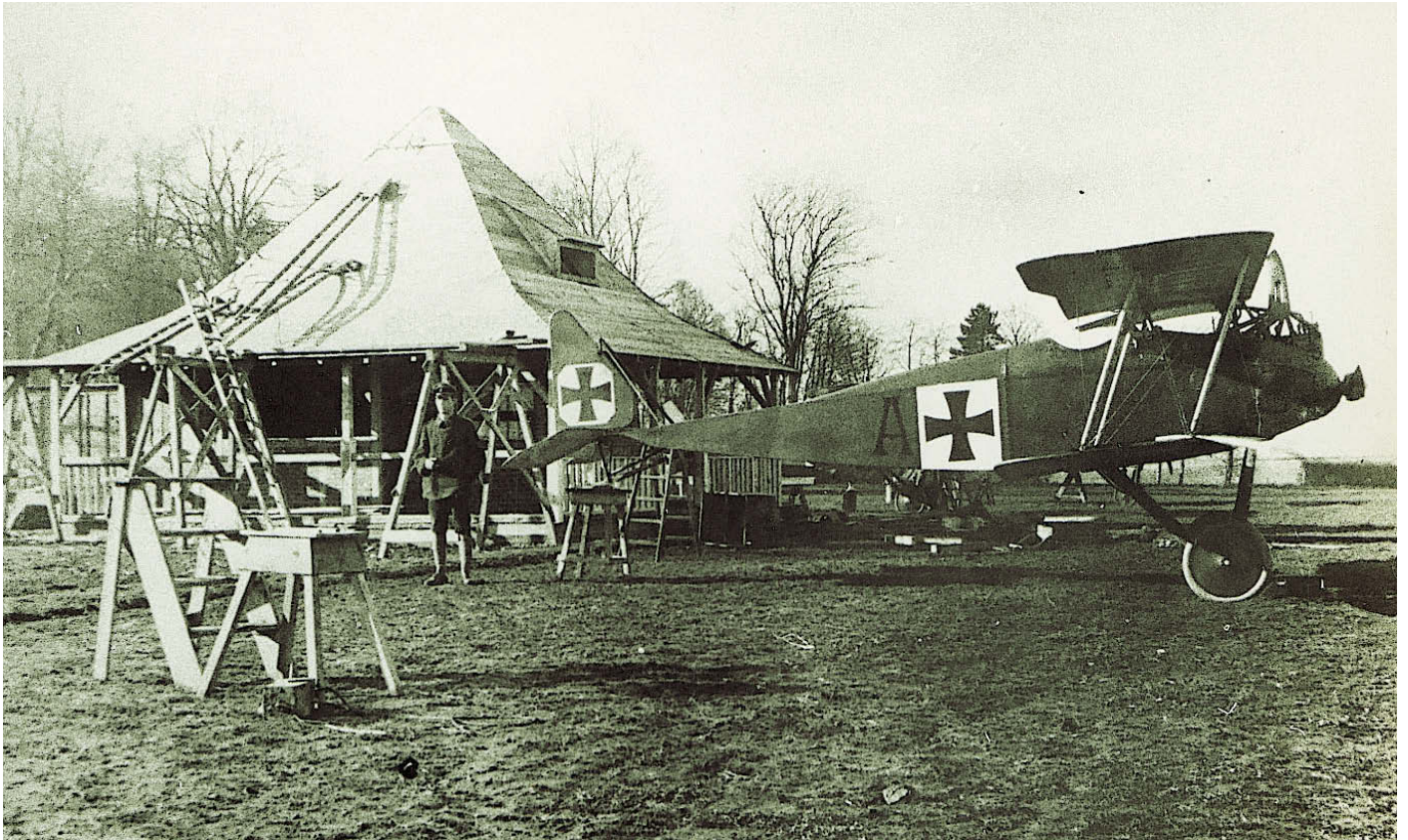
An Argus engined Halberstadt D.III. Note the exhaust stack arrangement, with stack ending above the upper wing.
