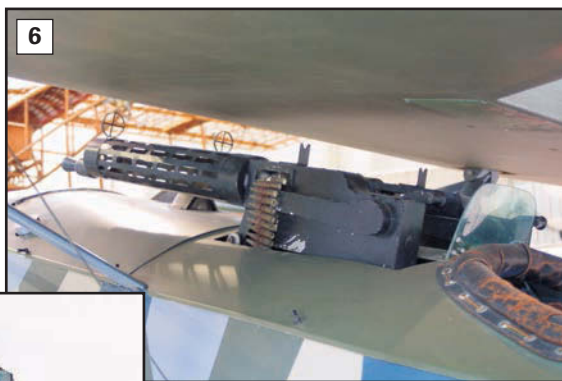
6 & 7: Two views showing the cockpit windscreen and the twin Spandau machine guns.
