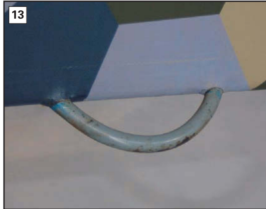
13: Lifting handle at the bottom of the rear fuselage side.
