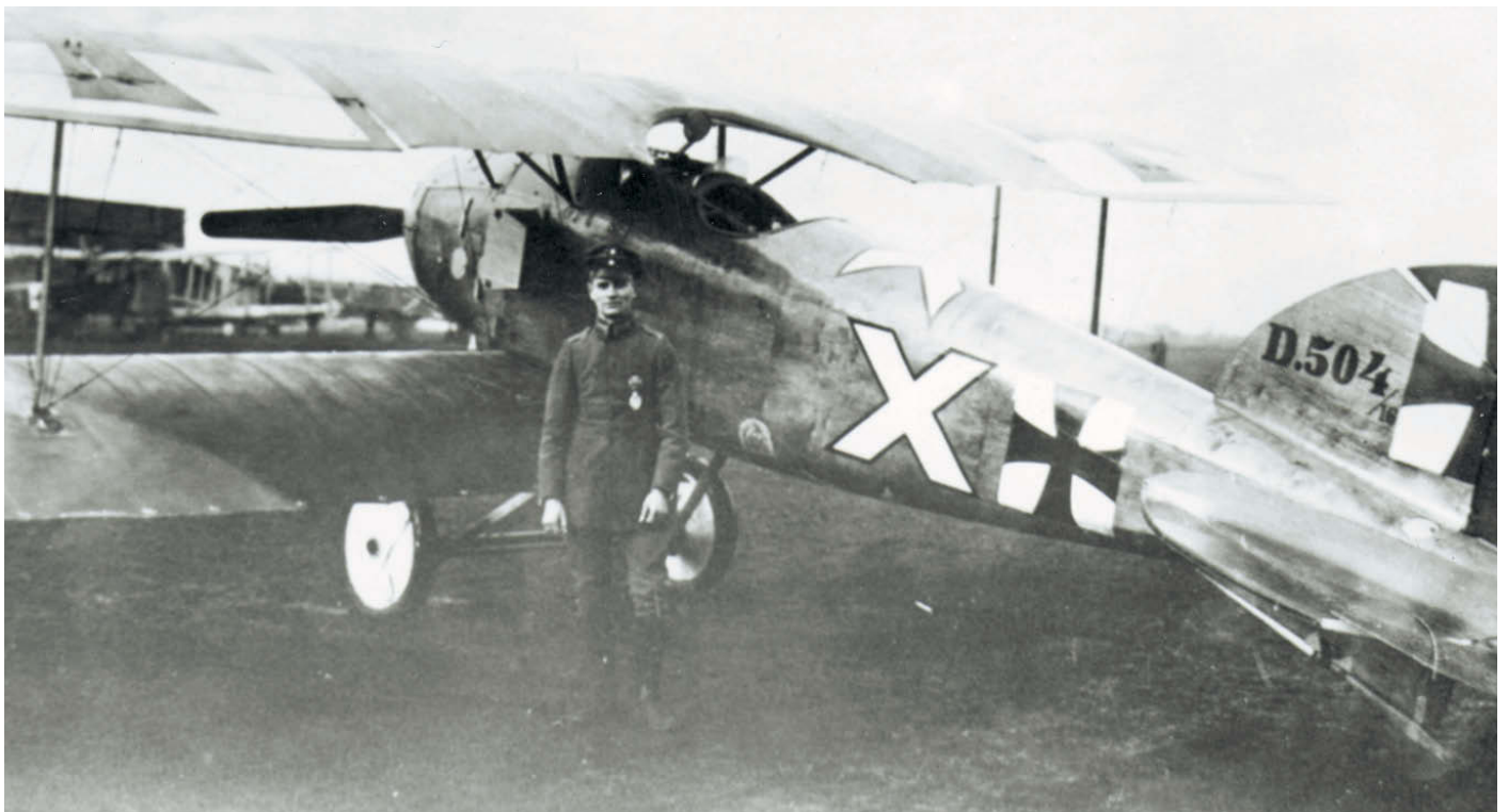
Early aircraft from the first production batch (D.504/16) shows clear-varnished fuselage. National insignia on square white backgrounds, sprayed finish, green and reddish brown. Kampfstaffel 11 in Kampfgeschwader 2, late-1916.
