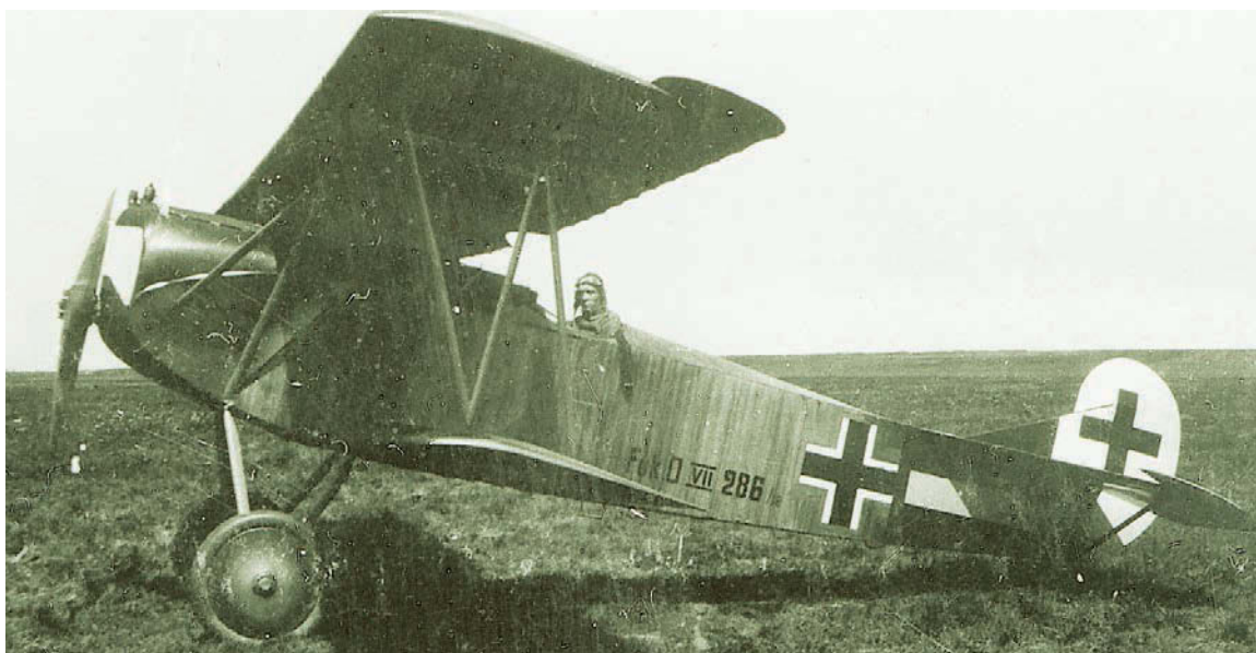
Many WW1 German Air Service pilots held senior N.C.O. ranks. This is VzFW. Willi Gabriel of Jasta II, whose aircraft shows little embellishment beyond a white fin/rudder and horizontal bar below the tailplane. The machine features the streaky finish (vertical on the fuselage) applied to very early D.VII examples.
