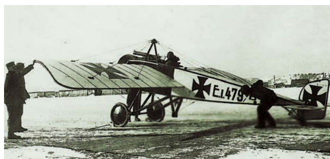
Pfalz E.1 seen at Vilna on the Eastern front, in what appears to be a rather wintry scene. At this stage of WW1, colour schemes were very simple. Wing warp mechanism can be seen behind undercarriage.
