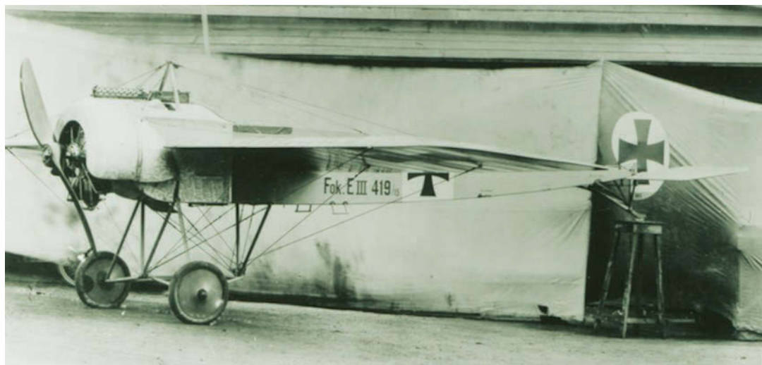
LEFT: A brand new Fokker E.III. The undercarriage struts are also visible here, together with the V-strut anchor for the wing warping mechanism.
