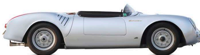
◁ Porsche 550 Coupé 1953 Origin Germany Engine 1,488 cc, flat-four Top speed 124 mph (200 km/h)
