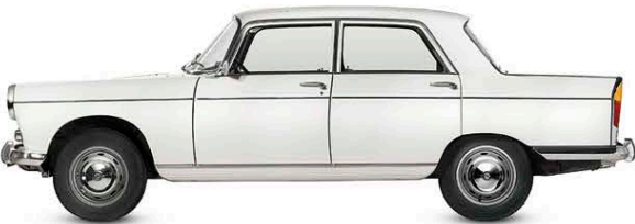
△ Peugeot 404 1960 Origin France Engine 1,618 cc, straight-four Top speed 84 mph (135 km/h)
