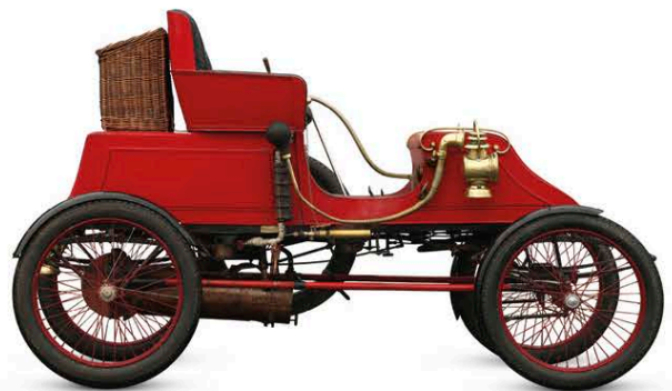
▷ Stanley Runabout 1898 Origin USA Engine 1,692 cc, straight-two steam Top speed 35 mph (56 km/h)
