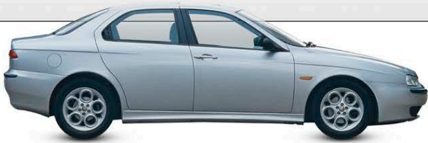
△ Alfa Romeo 156 TS 2.0 1997 Origin Italy Engine 1,970 cc, straight-four Top speed 133 mph (214 km/h) Alfa achieved class-leading styling with this sporting saloon. Features include concealed rear door handles to give it a coupé look.
