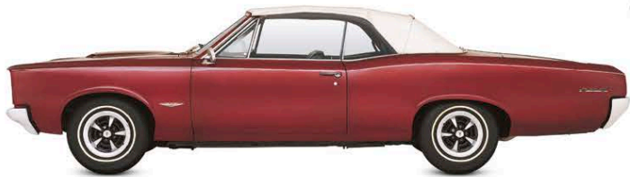
△ Pontiac Tempest GTO 1966 Origin USA Engine 6,375 cc, V8 Top speed 122 mph (196 km/h) The Tempest compact helped make Pontiac the third best-selling US marque of the 1960s and the GTO confirmed its performance credentials: it was a real hot rod.
