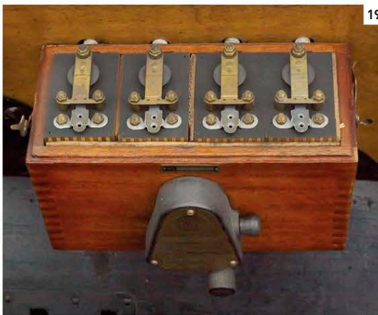
19. Trembler coils for ignition housed in box on dashboard 20. Transmission housing under the floor 21. Bonnet clip 22. Bonnet handle 23. Four-cylinder engine has a capacity of nearly 3 litres
