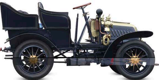
▽ Knox 8HP 1904 Origin USA Engine 2,253 cc, single-cylinder Top speed 28 mph (45 km/h)
