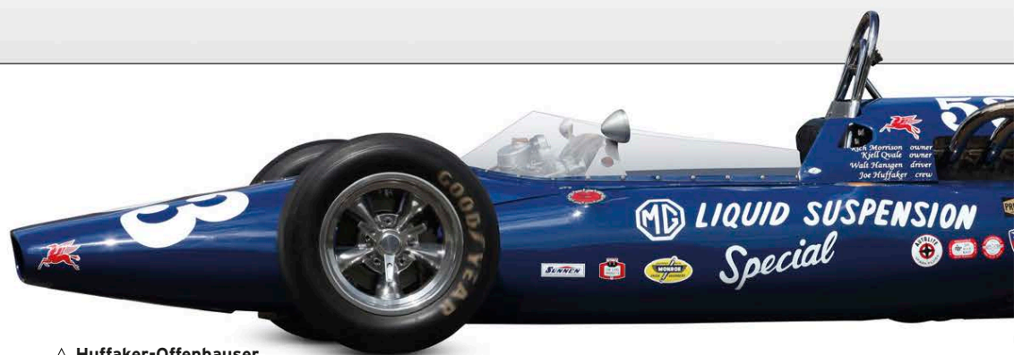
△ Huffaker-Offenhauser Special 1964 Origin USA Engine 4,179 cc, straight-four Top speed 180 mph (290 km/h)
