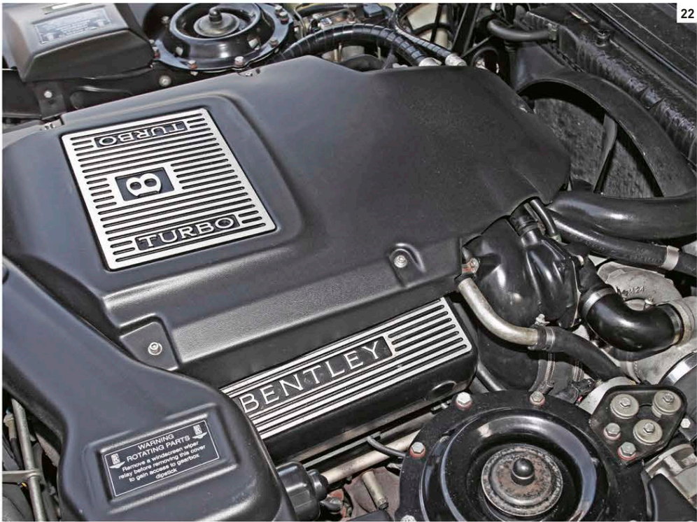
22. Modern shrouding hides 1950s engine design 23. Turbocharger source of Bentley's strong performance 24. Under-bonnet lamp
