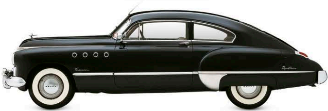
▷ Buick Super 1946 Origin USA Engine 4,064 cc, straight-eight Top speed 82 mph (140 km/h)
