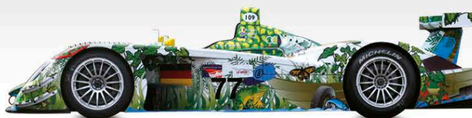
△ Audi R8 2000 Origin Germany Engine 3,600 cc, V8 Top speed 211 mph (339 km/h)
