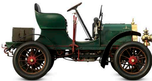
△ Vulcan 10HP 1904 Origin UK Engine 1,500 cc, straight-two Top speed 35 mph (56 km/h)
