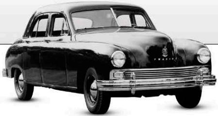
△ Kaiser Frazer F47 1946 Origin USA Engine 3,707 cc, straight-six Top speed 82 mph (132 km/h)
