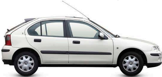
△ Rover 25 VVC 1999 Origin UK Engine 1,796 cc, straight-four Top speed 127 mph (204 km/h) Based on engineering from Honda pre-1994, the 25 was well equipped and good value, with engines from 1.1 to 2.0 litres.
