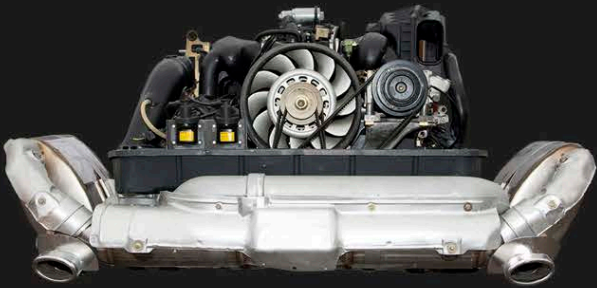
Low profile Although the cylinders and crankcase are obscured in this photo of a 1994 flat-six, the engine's low, wide stance is obvious. This helps the engine fit neatly into the tail of the 911, while the lowered centre of gravity aids roadholding.
