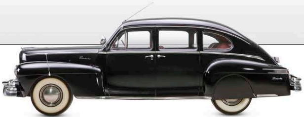
△ Lincoln 1946 Origin USA Engine 4,998 cc, V12 Top speed 92 mph (148 km/h)
