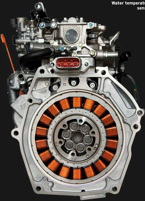
Electric motor Copper coils form part of the Honda Insight's electric motor, which performs three functions: it starts the engine, boosts torque, and provides regenerative braking to recharge the battery pack.
