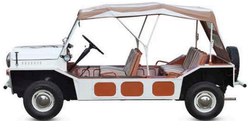
△ Mini Moke 1964 Origin UK Engine 848 cc, straight-four Top speed 84 mph (135 km/h)
