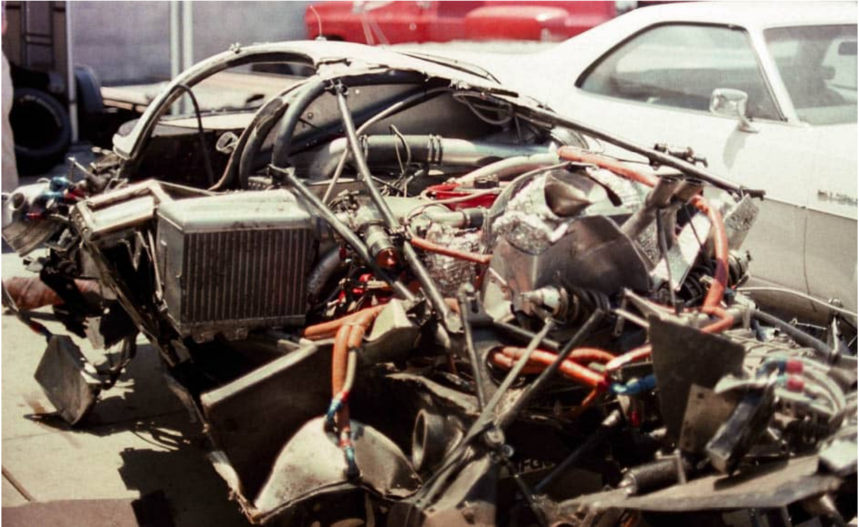
At Jim Busby's workshop: the BFG Team's early 962 sheet-aluminium monocoque, somewhat bent. (JC)
