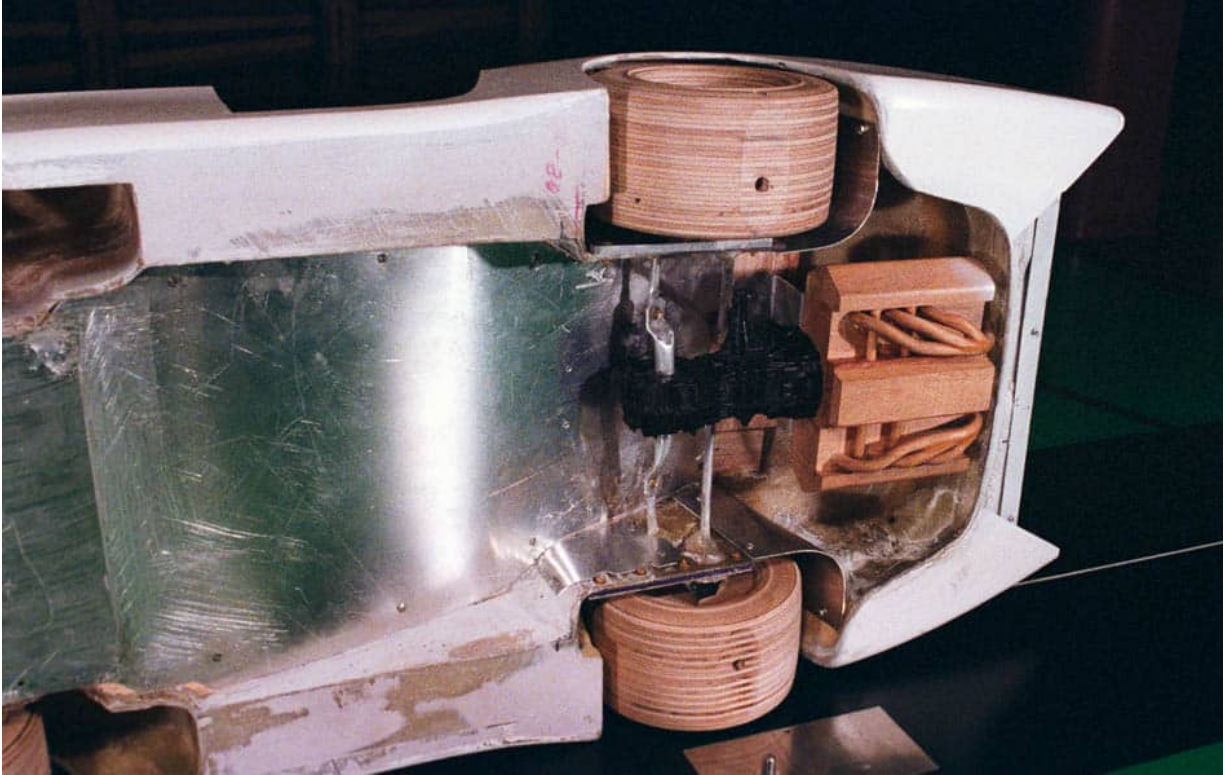
Singer's wind tunnel 935, planned to be the ultimate development of the 935. Here we see the early signs of the shaped floor. (P)
