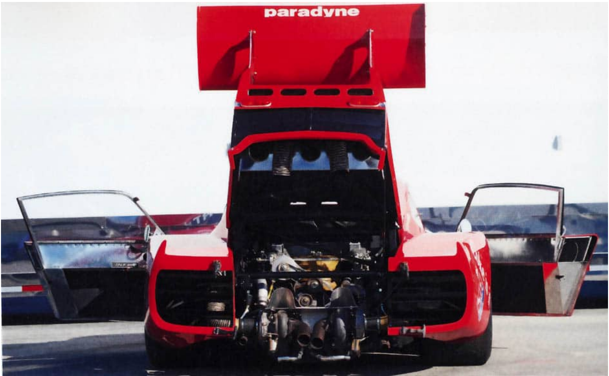
Twin-turbo arrangements on the 836bhp 3.2-litre 930 engine. The car would run well, but was too late in terms of technology to make any significant impression. (DK)
