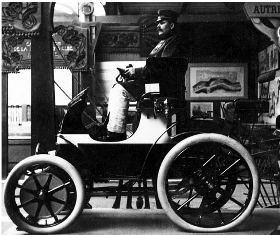
The first front-wheel drive Lohner Porsche vehicle, electrically powered from batteries supplying current to the electric hub motors, displayed at the 1900 Paris World Fair. (P)
