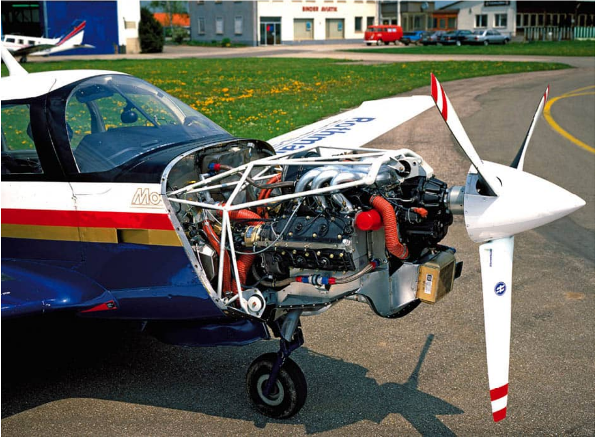
A Mooney M20 aeroplane manufactured by the Mooney Airplane Company. It was powered by a Porsche PFM 3200 six-cylinder horizontally opposed air-cooled aircraft engine, developed by Porsche from the 911 3.2-litre. (P)
