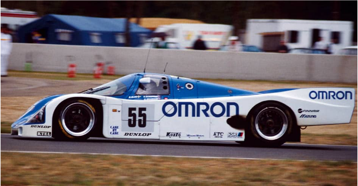
Note the low-downforce Le Mans spec bodywork in comparison with the Suzuka race. (TC)
