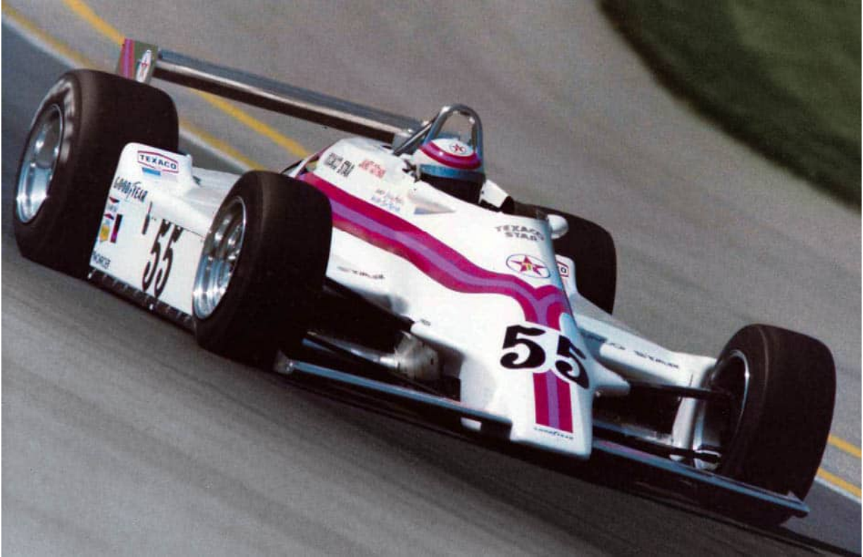
One of the first ground-effect cars to run at Indy. David Bruns (Swift Cars) designed it at Fabcar. (DK)
