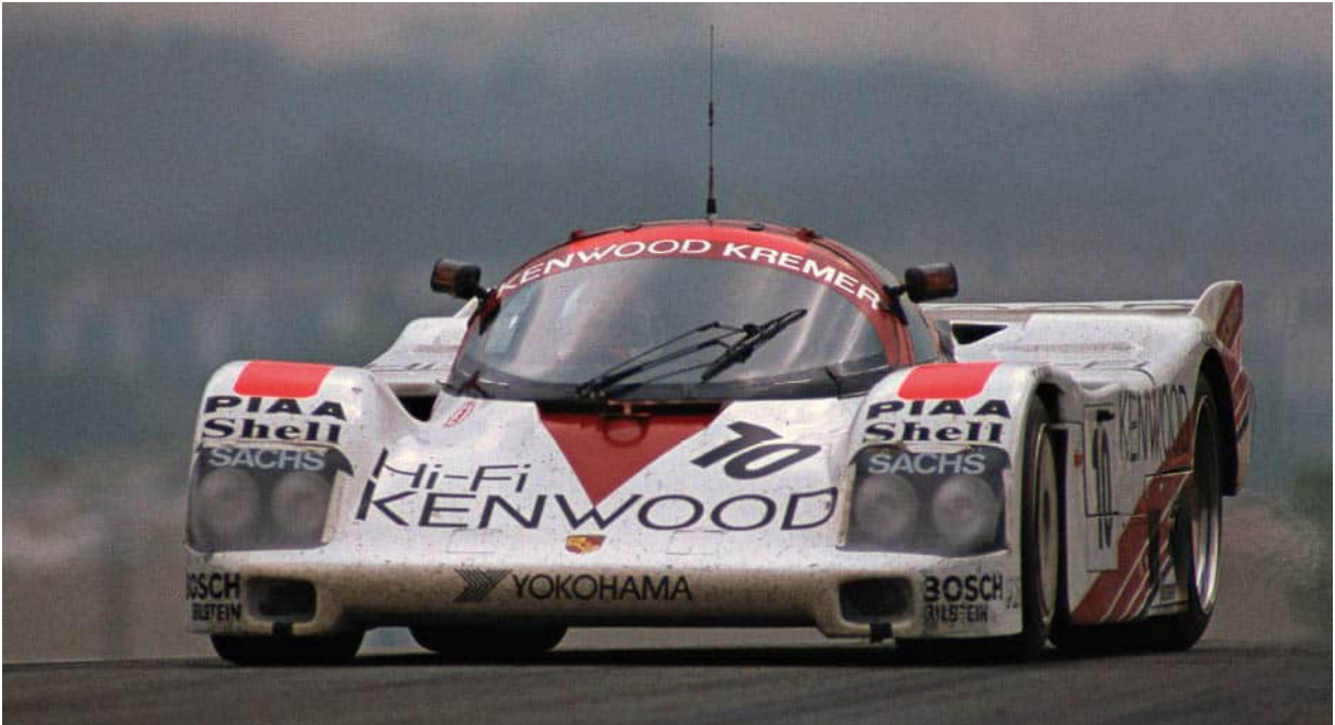
Le Mans 1988: Giacomelli/Takahashi/Okada in the updated CK6, now CK6/88 CK6, a Thompson monocoque honeycomb chassis, the engine being the 935/79 2826cc type, 9th overall in the race. (P)
