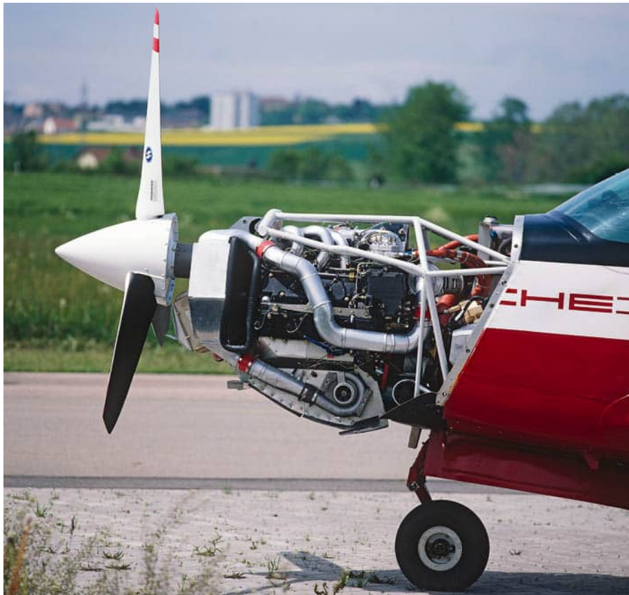
Turbo-powered aircraft engine: the 3200 in 1987, the turbo clearly visible under the engine. (P)
