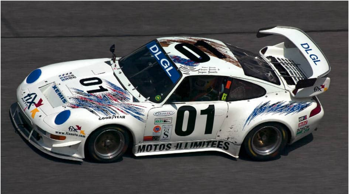
This is a Fabcar tube-frame chassis Porsche 993 Carrera 2 #AJR911GT3, powered by a 3.8-litre Porsche turbo engine at the Daytona Finale 3H, 10 November 2002, run by the Canadian team GLDL and driven by Jacques and Hugo Guenette. (MS)
