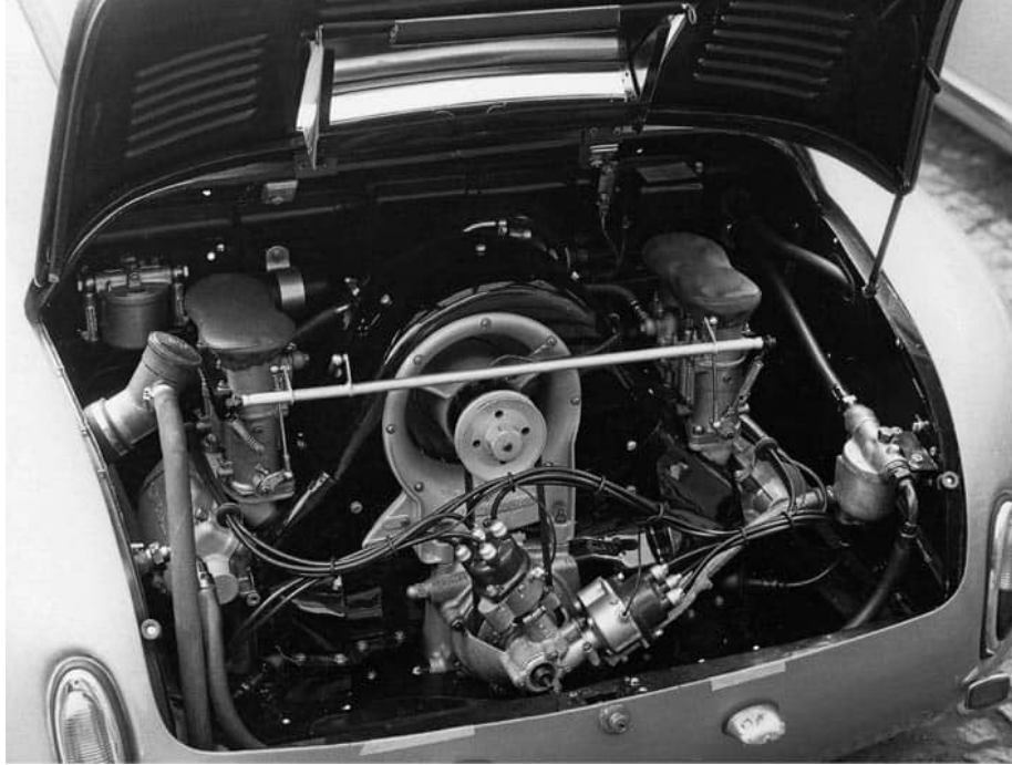
The 1600 GS quad-cam Carrera engine, featuring dual ignition circuits, 1960. (P)
