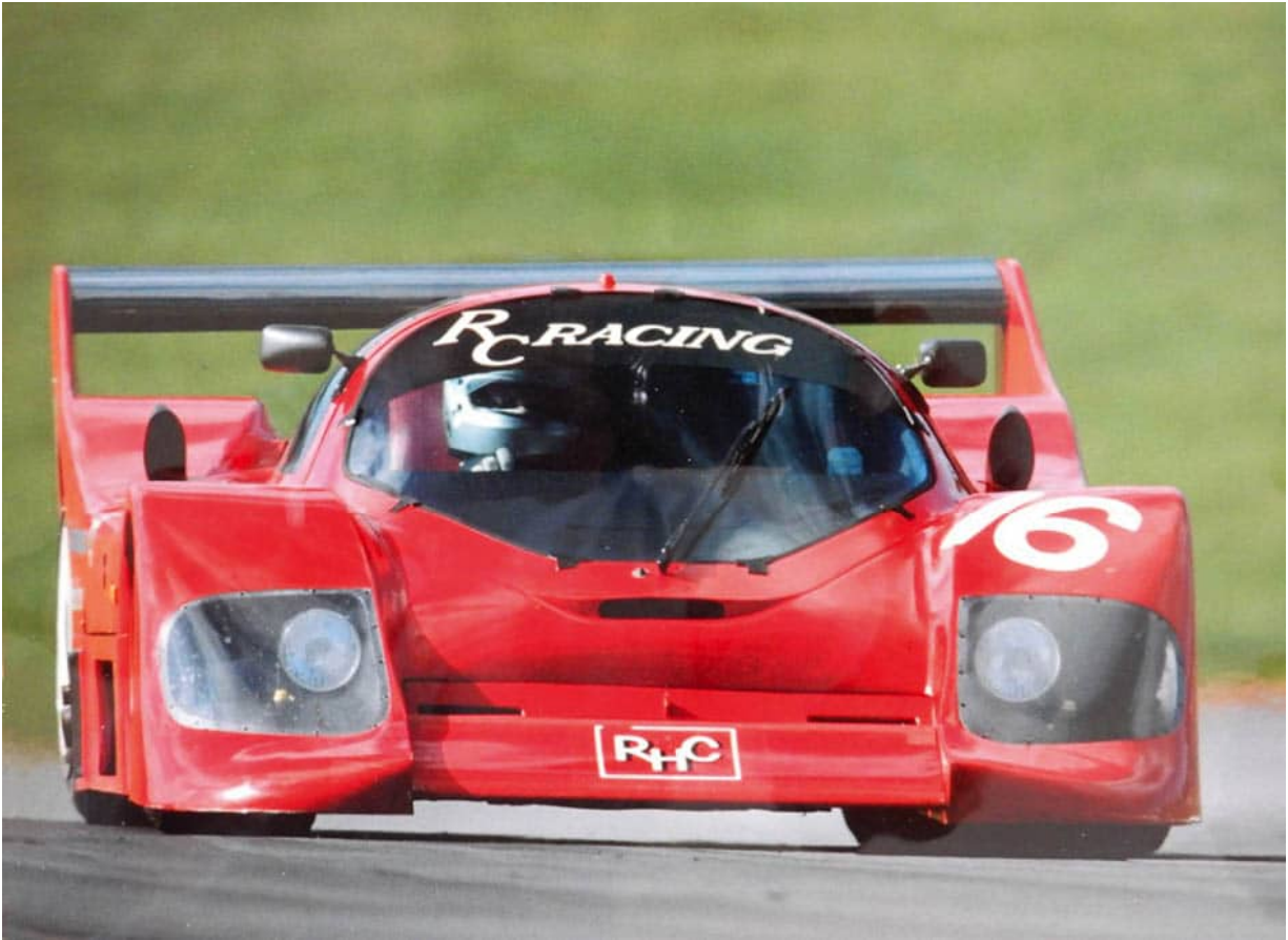
A now-modified Richard Cleare Kremer CK5. Peter Twitchen explains: "We tried several different aero modifications during our time with the CK5, and here we see the different nose with an airfoil section replacing the conventional smooth front end; this is at Brands Hatch, 22 September 1985." (PT)
