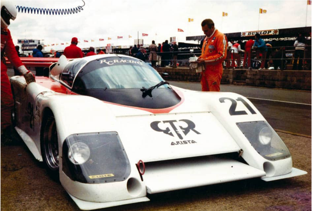
The former John Kalagian March-Porsche 85G-06, fitted with an Andial IMSA 3.2 spec engine, seen here at the Silverstone 1000km on its first eventful outing, 5 May 1986. (PT)
