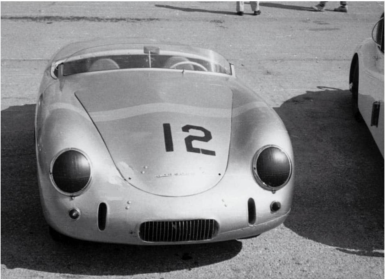
This is the Glöckler No 3 that would influence the new Porsche design, a sports racing car of its own which became the type 547, and eventually the type 550. Glöckler 3 had a 1952 Porsche 356 chassis with open alloy bodywork by Weidenhausen. (P)
