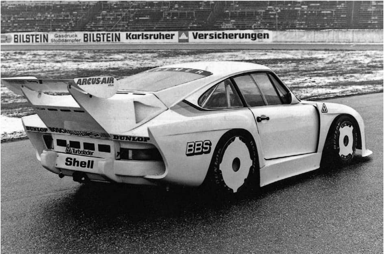
The Kremer 935 version K3 as it was introduced to the press in a presentation at Hockenheim in 1979. This one is chassis 009 0002, powered by a Kremer-tuned, twin-turbocharged Porsche 3163cc engine giving around 805bhp. (P)
