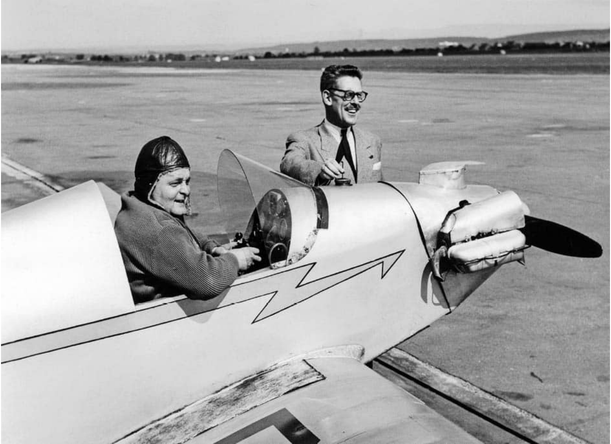
Here we see a Jodel B b  aeroplane in 1956 on the airfield in Echterdingen. The plane was powered by an aircraft type 678 Porsche engine. At the front of the plane stands Huschke von Hanstein. In the aeroplane, one Karl-Heinz Martin from Saarbr cken. (P)
