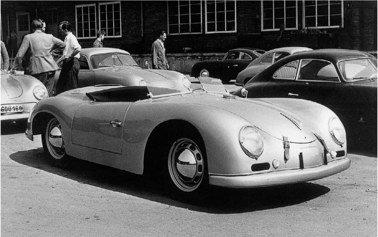
1951: the first special-bodied Sauter-Porsche, featuring an ultra-thin steel body, front-opening doors (often called suicide doors) by Klenk; the Porsche engine was modified from the standard 1100cc to 1300cc. (P)
