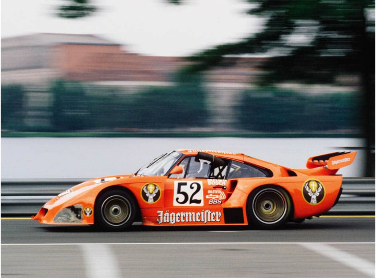
The 810bhp car could reach 300km/h. The K4 was derived from the shape of the earlier Porsche Werks car, the 935/78. (P)
