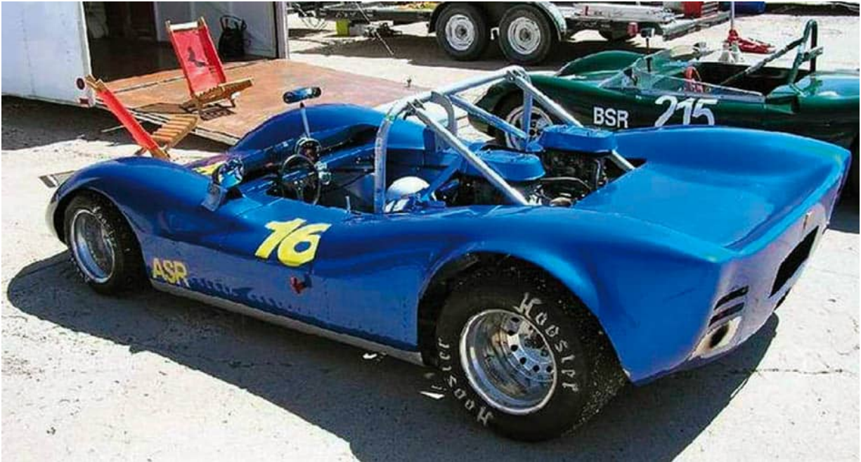
A Mk III Sabel-Porsche, seen here powered by a Porsche 2.2-litre six-cylinder driving through a Hewland Mk VIII gearbox. It still regularly runs in SCCA Regional events. (Sab)
