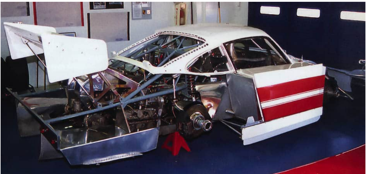
A tube-frame chassis with monocoque parts designed in a similar way to the GAACO 935, but with Dave Klym's Fabcar expertise it pushed the boundaries of aerodynamics. (DK)
