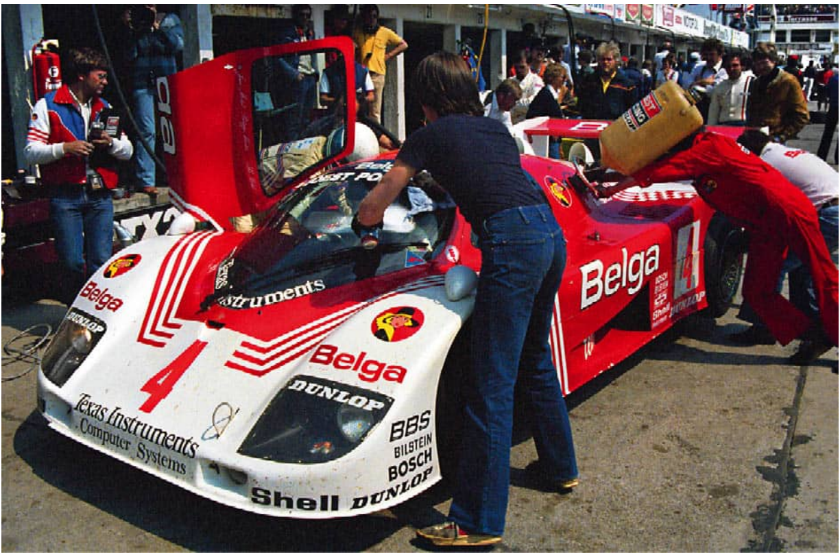
936C JR-005 at Monza 1982: the Belga car is the Joest-built 936C, using a 936 tube/space frame and 936/917 running gear. (P)
