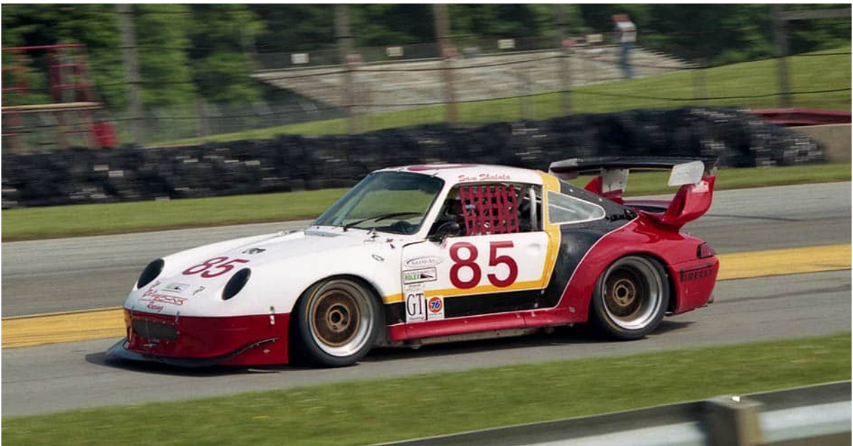
Sam Shalala's tube-frame Fabcar 911 rear engine with a 3.8-litre Lozano-Porsche engine at the Mid-Ohio 250 Miles. (MW)
