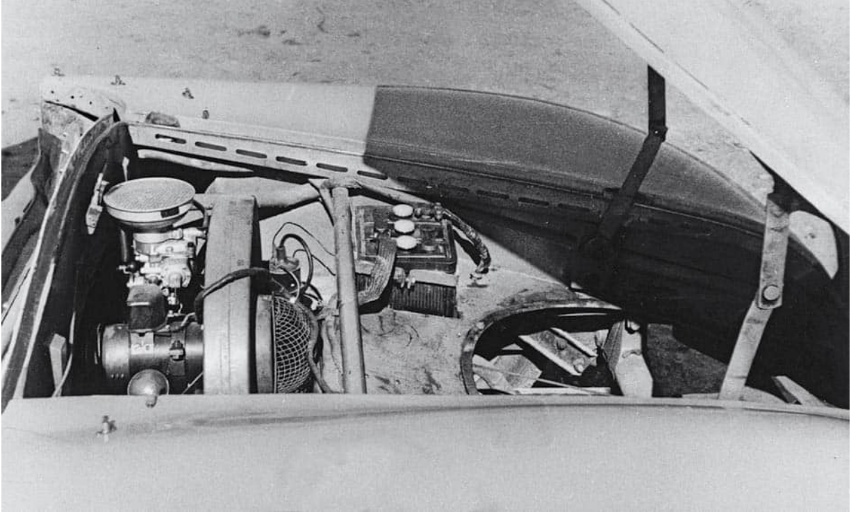
The original mid-engine installation; the first Porsche-created road car in 1948 with this mid-engine concept. (P)
