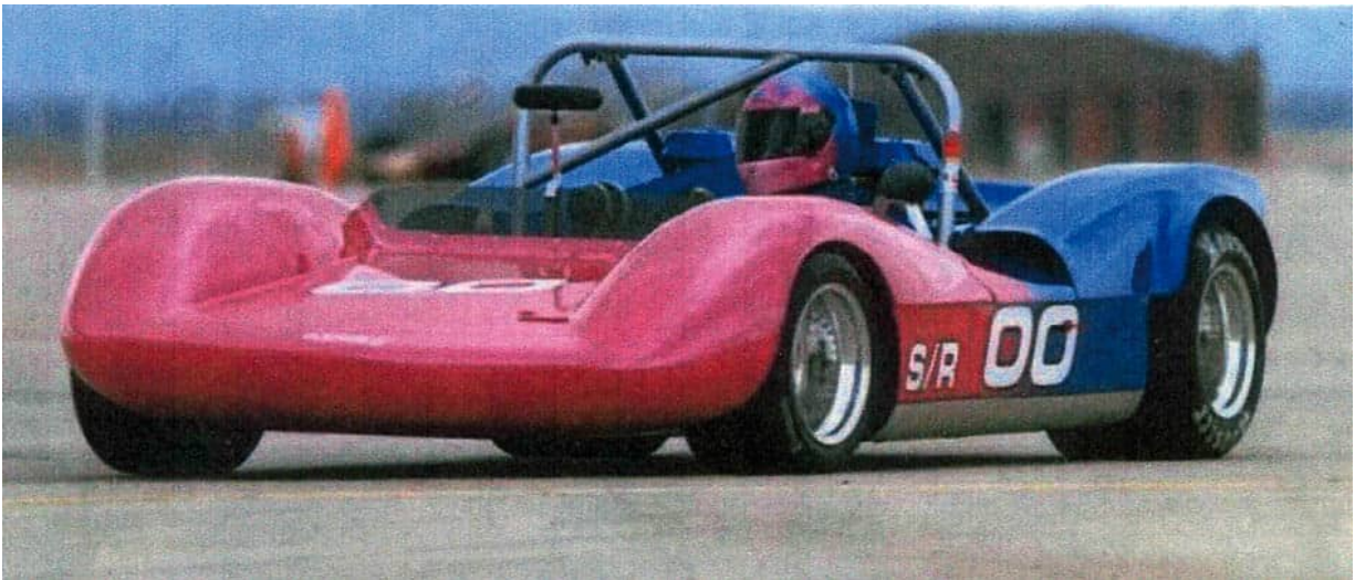
The ultimate Sabel evolution in recent times: Porsche 911-powered, mid engine Sports prototype racer. (Sab)
