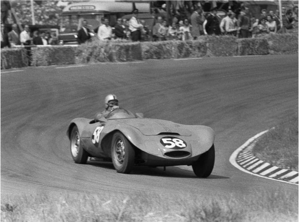
Henk van Zalinge's Hirondelette: a superlight chassis, it had its Porsche engine installed ahead of the driver. (JB)
