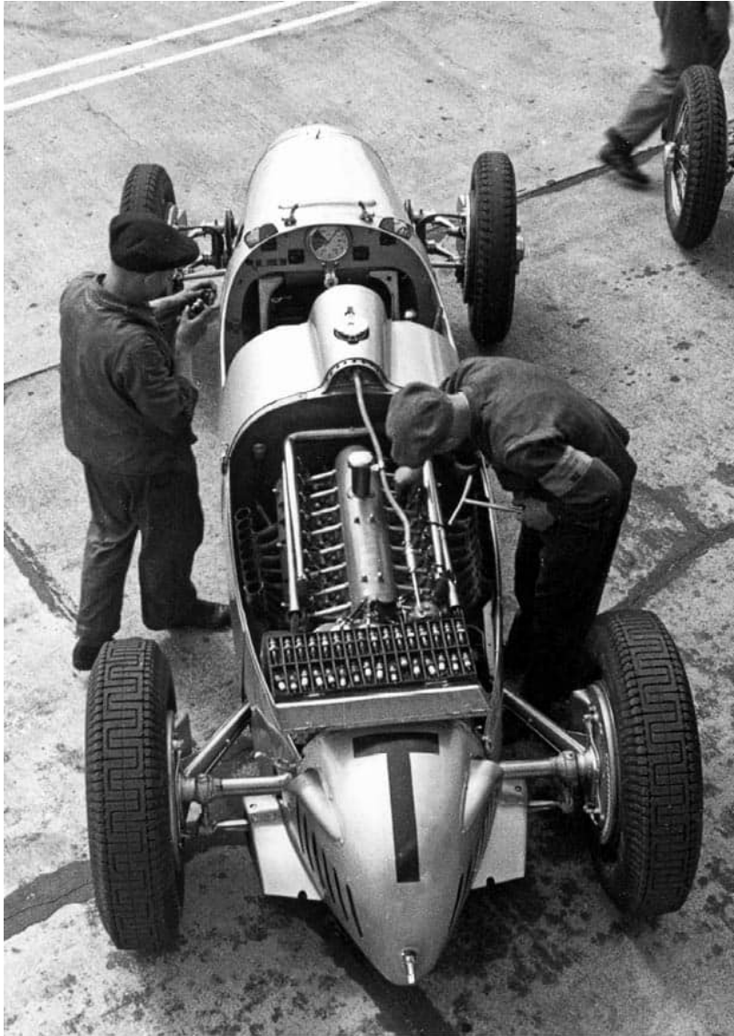
The V16 Porsche engine powers the new Auto Union. This one is the Type C Auto Union (Porsche Type 22). Mid-engine, 16 cylinders, V format at 45°, 6-litre. The first units produced 295hp from 4.4-litre. It was first driven in 1934 by Willy Walb, who had also been involved with the Tropfenwagen when at Mercedes. (P)
