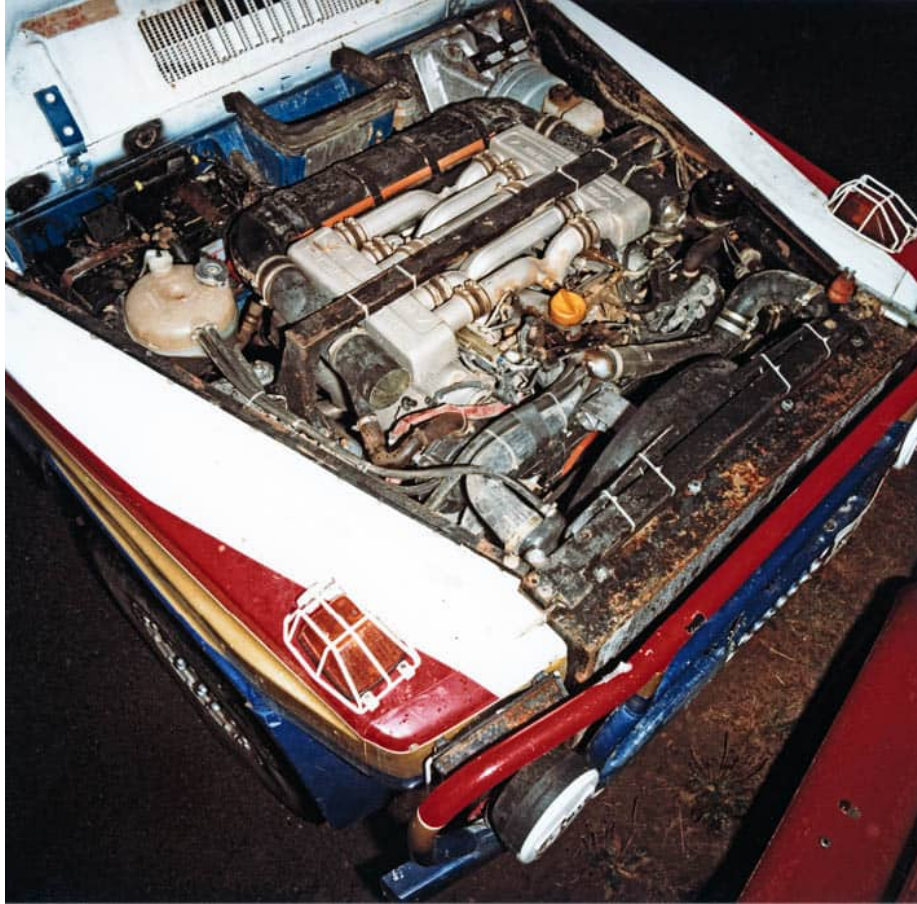
The Mercedes G-Wagen with its Mercedes engine; the inline six was swapped for the Porsche V8 928, 32-valve unit. (P)
