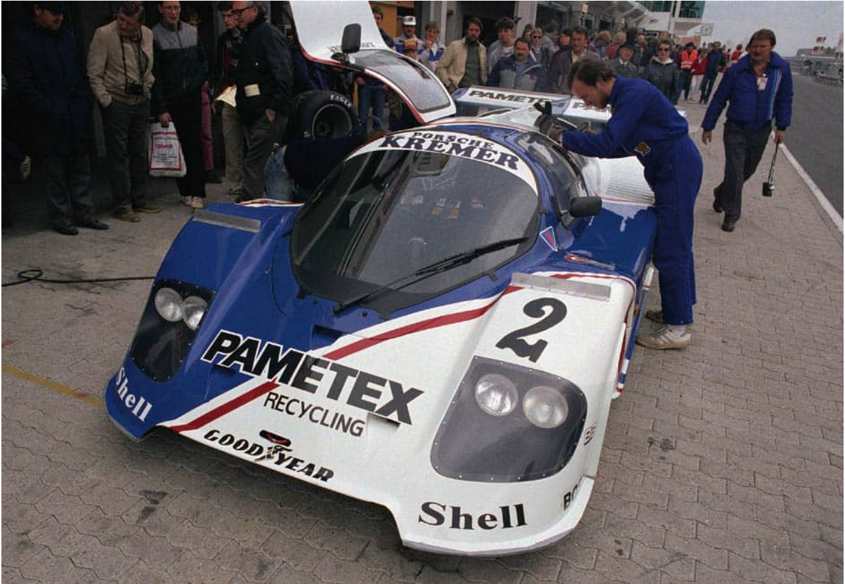
The CK5-02 at the Interserie Hockenheim for a German National Championship round on 21 April 1985. Note the aluminium strips aero experiment above the front wheelarches. (P)
