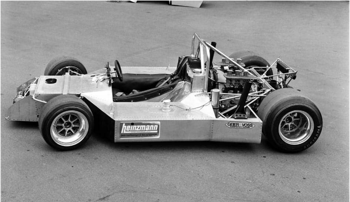
Conventional layout of fuel tanks in side pods, and a detachable rear part where a cradle supported the engine. (P)
