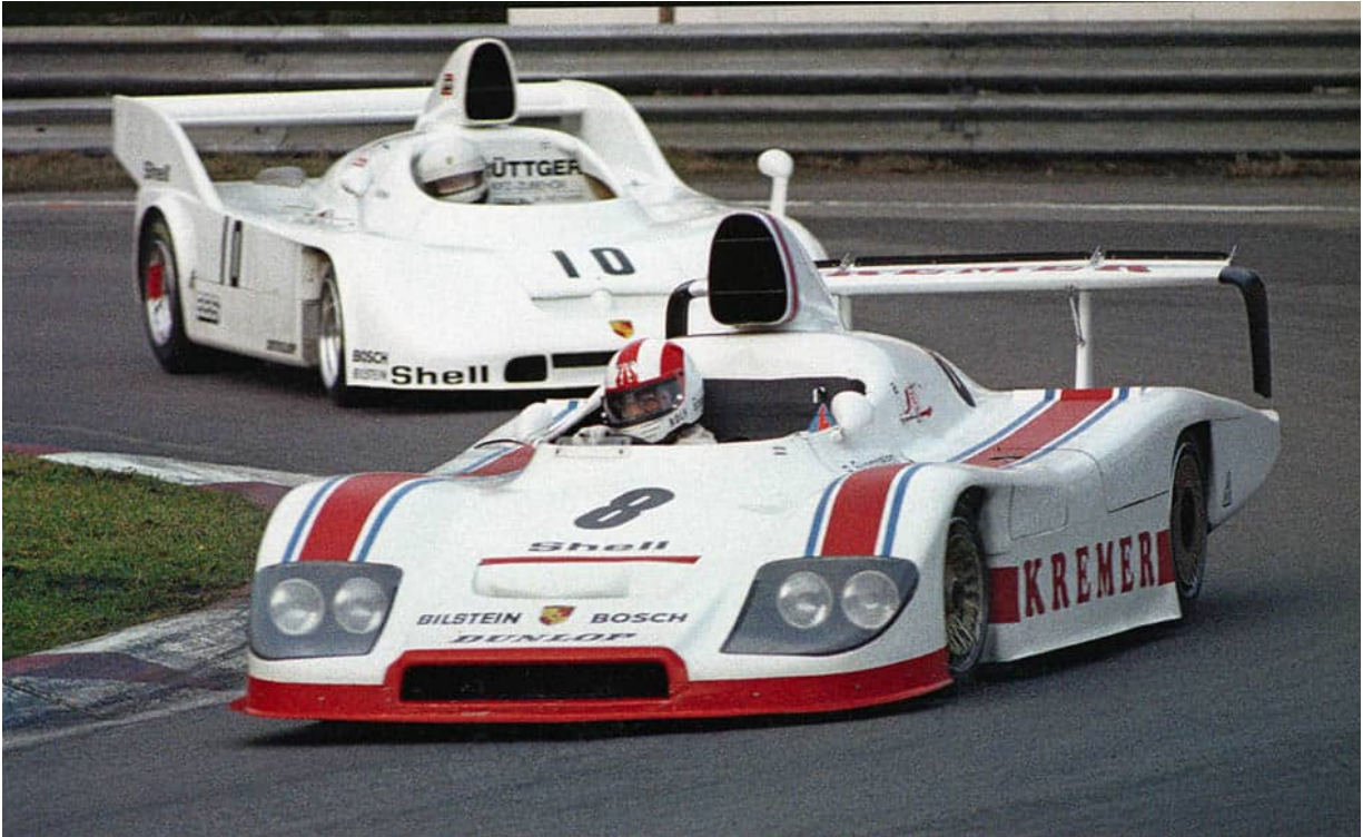
The (#8) Kremer 936-82-1, Porsche 2142cc, compression ratio 6.3:1 up to 7.0:1, 540bhp at 8000rpm. Twin KKK (Kant, Kopp, Kausch) turbos, boost adjustable by the driver using dashboard-mounted control. (P)
