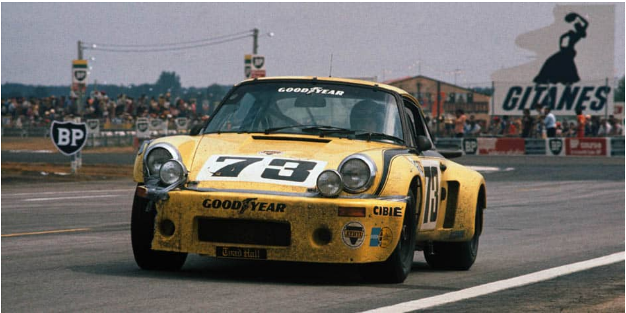
73 RSR of Milt Minter/Michael Keyser/Paul Blancpain at Le Mans in 1974 sporting the deep front bumper to aid aerodynamics. (MK)
