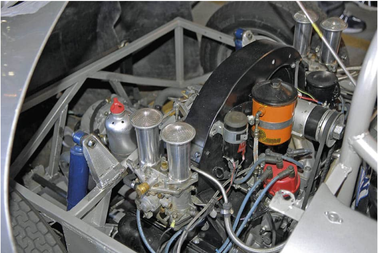
The 356 engine in the Pupulidy is installed behind the driver in a mid-engine position. The car weighs in at 1200lb (544kg). (PA)
