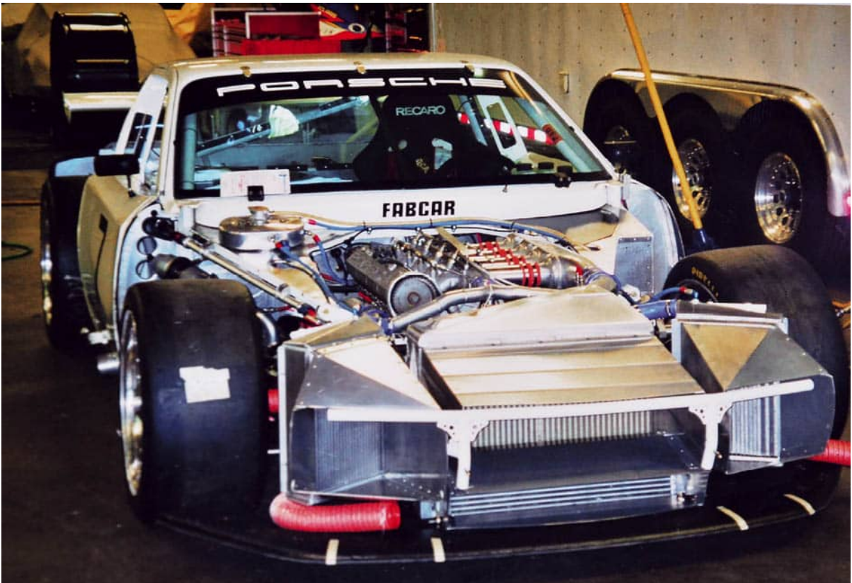
The Andial 2.5-litre installed in the Ludwig Heimrath car, 001 of the seven Dave Klym-built chassis. It would take a while to sort out.
