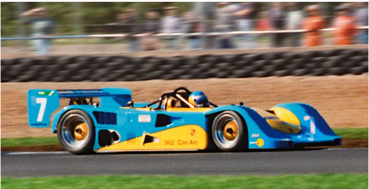
A whole new car, not a conversion. The 962-911 chassis was made by TC Prototypes as an open car from the start, to the Interserie CanAm regulations. (JS)
