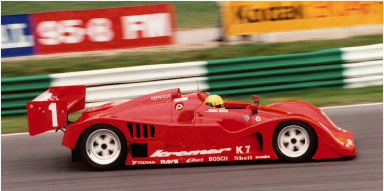
For the 1992 Interserie challenge, Kremer created the K7 from the Thompson-created 962 aluminium honeycomb-chassised CK6 car used in 1991, seen here at Brands Hatch. (JS)
