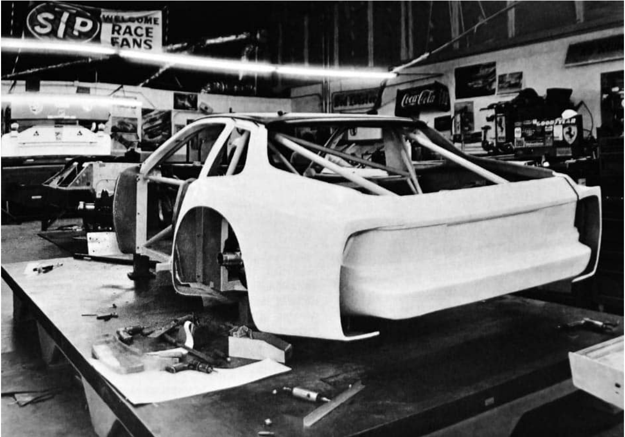
1985: a new superlight space-frame silhouette 924/944 GTR created by Dave Klym was on the cards, seen here in the workshop. (P)
