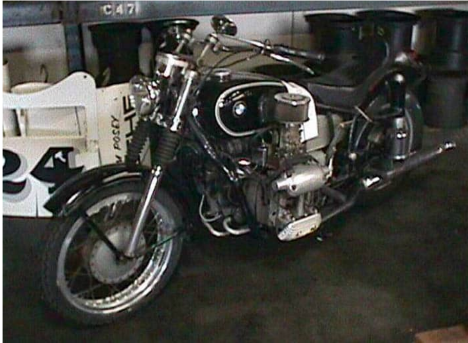
Vasek Polak's BMW, fitted with the four-cam 1957 Porsche 356A Carrera 547/1 Engine. (WDP)
