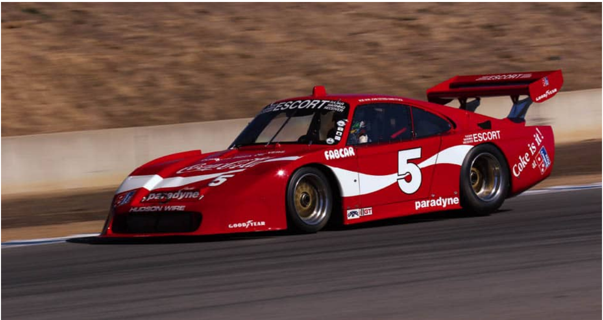
935-84: a tube-frame car, but similar in ideas to the JLP4 from the same design team at Fabcar. (MS)
