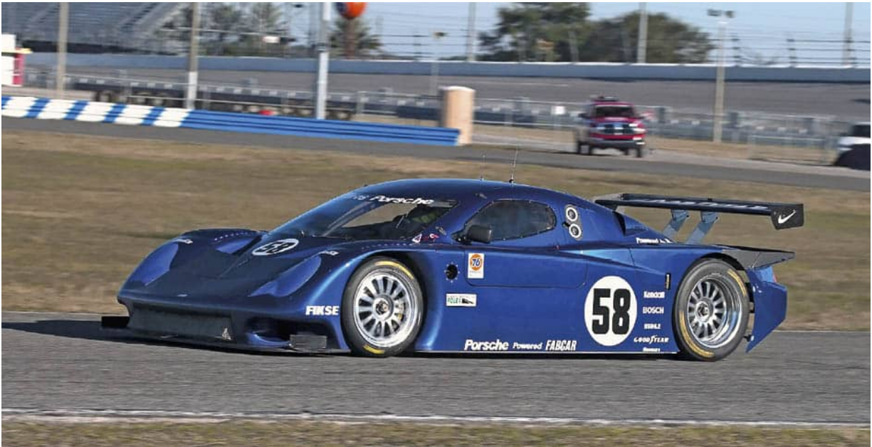
Advanced testing at Daytona in 2003: ready to rock and roll – the new Fabcar coupé Sports Prototype chassis 2, powered by the Porsche 3.6-litre GT3 RS engine, running in anger. (DK)
