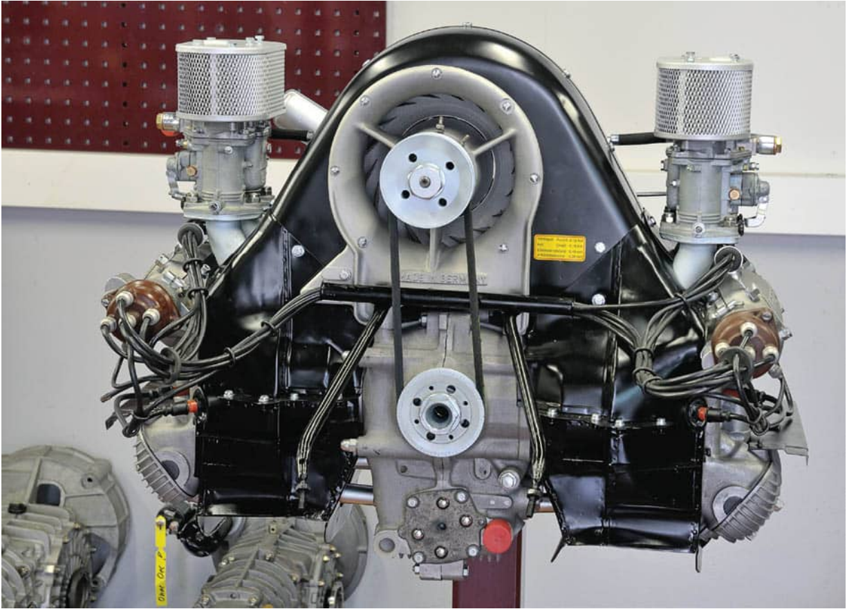
A beautiful piece of engineering: the Fuhrmann quad-cam Carrera engine. (P)
