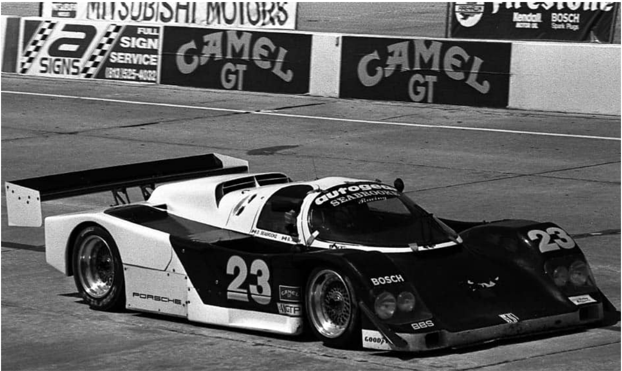
By January 1990, the RLR 202 DR1's front wing had been dumped in favour of the conventional nose arrangements, carried through from the Daytona 24 Hours to here at Sebring. (MW)
