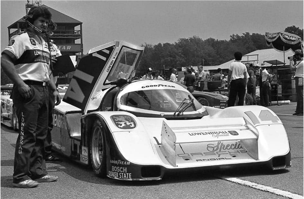
Mid-Ohio 1986: the new wing arrangement (similar to that employed on the Richard Lloyd car in Europe) for the Holbert/Bell 962 HR1. They took victory, but did the wing help? As far as Porsche was concerned, the jury was out on that one. (MW)
