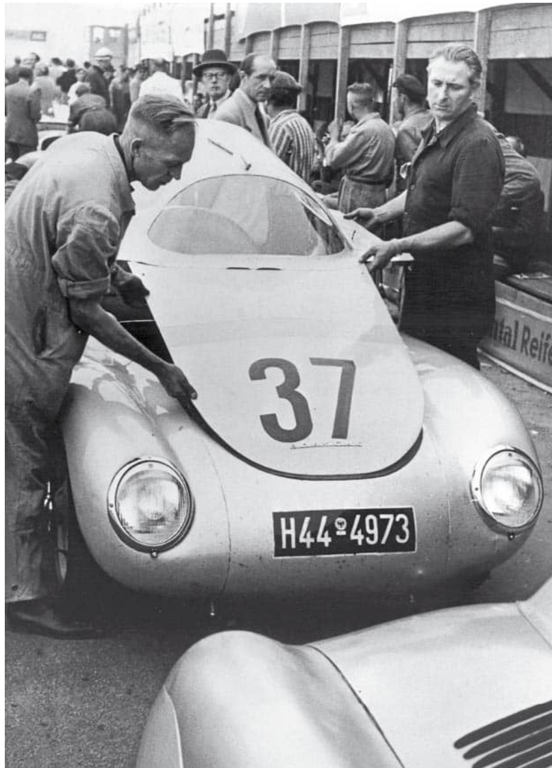
Glöckler No 2 having its detachable, Weidenhausen 2-312-37 body/canopy fitted; with the 85bhp Type 502 engine, the Glöckler No 2 weighed in at 450kg. (P)
