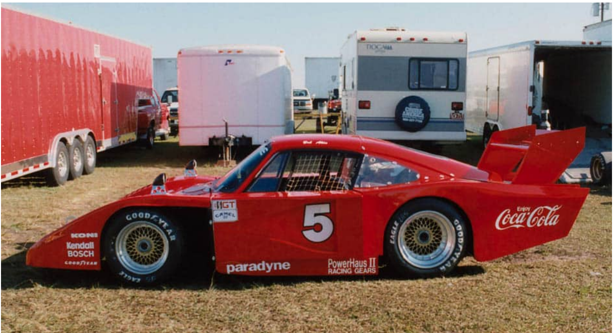
935 LT1 – a Lola T600-inspired long-nose, lightweight body covers the bonded monocoque chassis created by Team GAACO's 'Rabbit' Bartrills, designed by Lee Dykstra. (JS)
