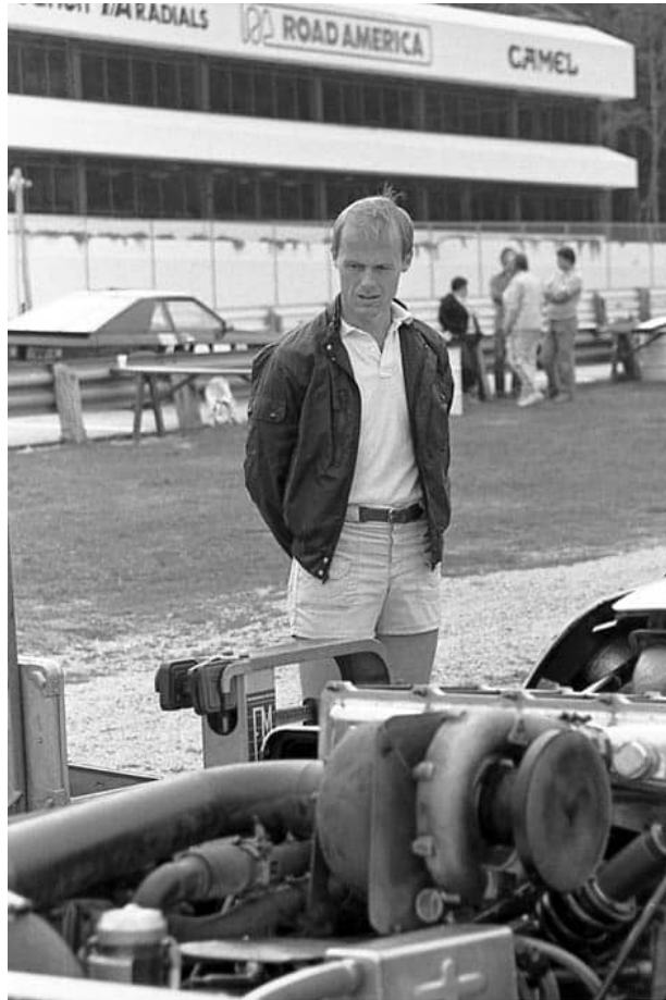
Al Holbert studies one of his cars at Road America, April 1986. Note the high-mounted intercooler and turbo; hence the air intake above the rear cover of the Holbert cars of the time. (MS)
