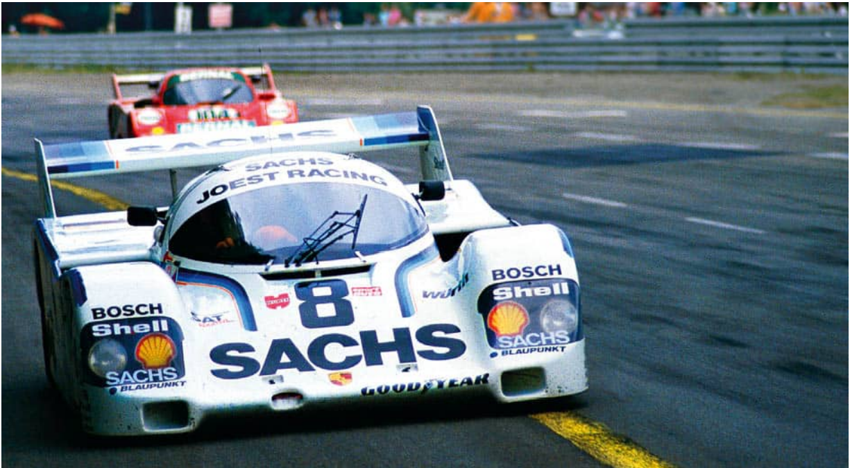
The Joest-run 962C utilising a Thompson monocoque numbered 116. This car was powered by a Type 935/79 DOHC 2826cc turbo engine. Seen here at the Norisring on 28 June 1987 for the Nürnberg 200 Miles: Louis Krages/St Stanley Dickens, 3rd overall from the aggregated two-heat race. (P)
