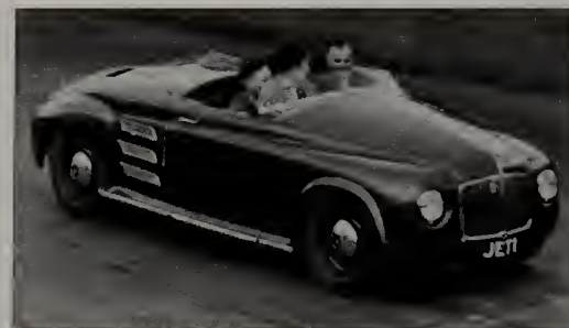
At this time Rover were busy with the development of their gas turbine car. Here it is in 1952.
