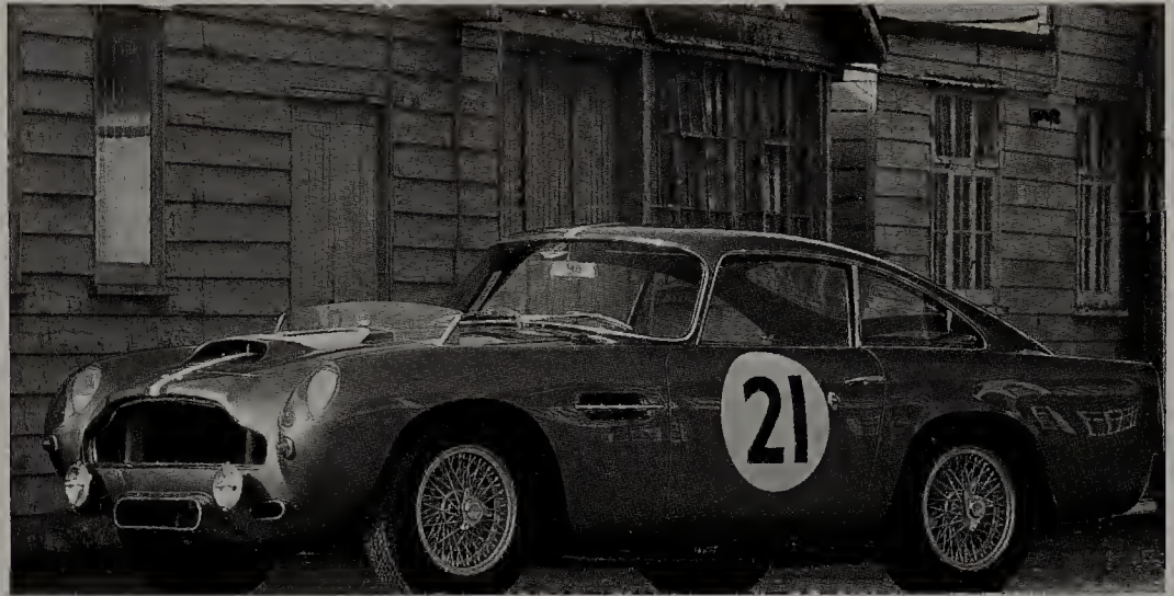
DB4 GT had a shorter wheelbase than the DB4 and power was increased to 302bhp.
