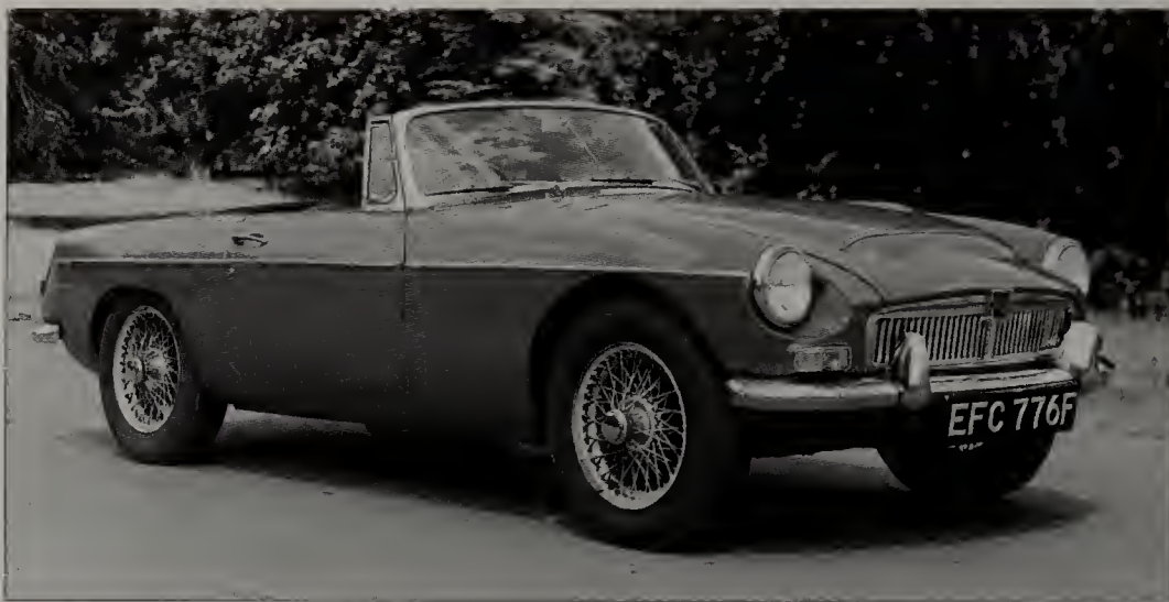
MGC, 1967, with characteristic bonnet bulge to accommodate the six-cylinder engine.
