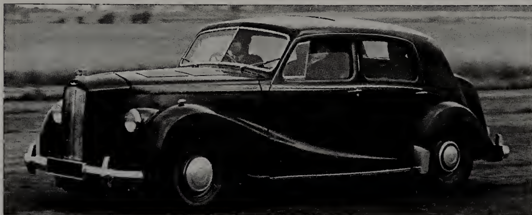
A gas turbine-powered Sheerline on test.
