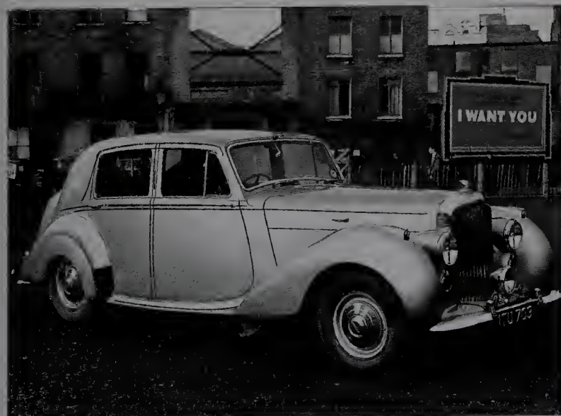
Later Mark VIs gained rear wheel spats.
