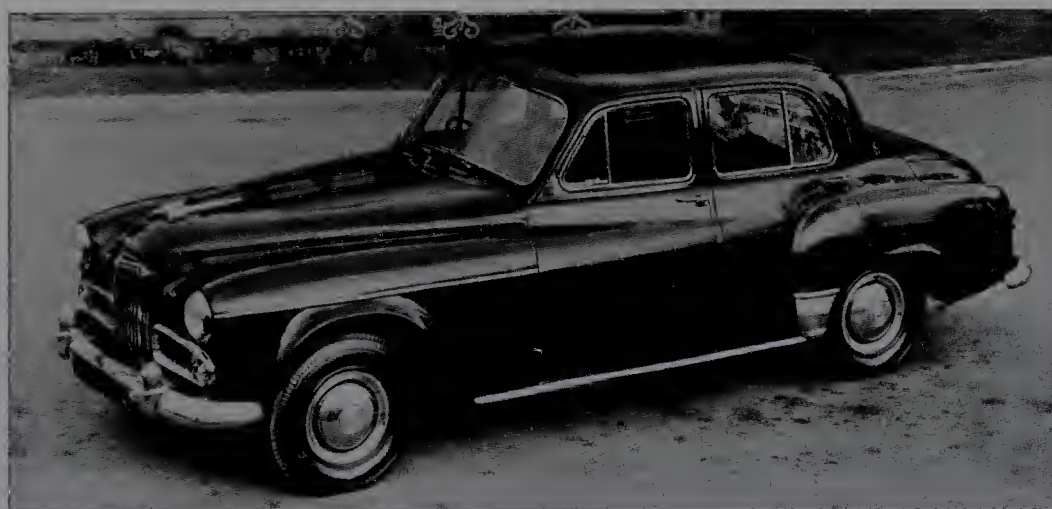
The new 1953 Super Snipe Mk IV, now with 4.1-litre ohv engine.
