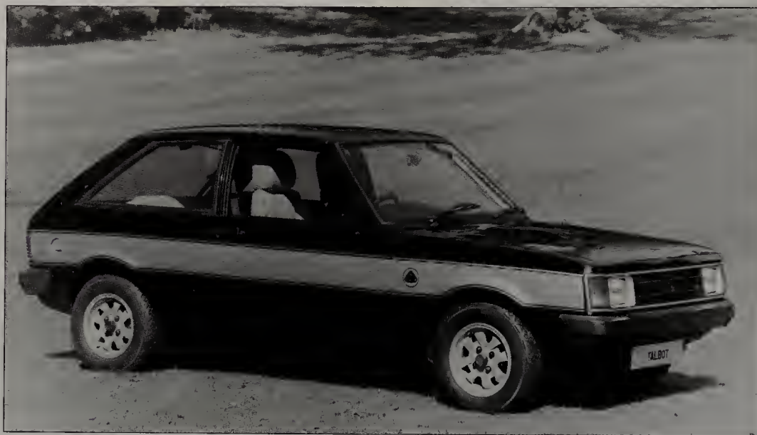
Talbot Sunbeam Lotus, with a 2.2-litre 150bhp twin-cam engine and five-speed gearbox.
