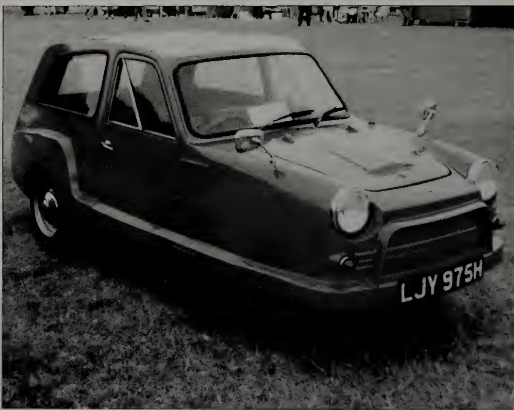
Bond 875: a three-wheeler with a Hillman Imp engine.
