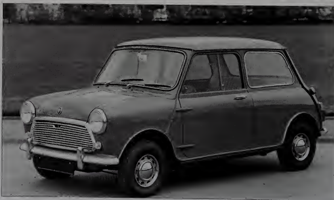
Mark II Mini with restyled grille but retaining external door hinges and sliding windows.
