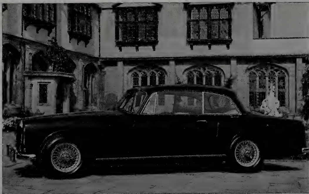
The TF21, sadly the last Alvis model, had 150bhp and a 120mph top speed.
