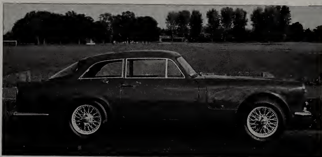
The 3.5-litre Warwick had the Buick V8 engine later used in Rovers.
