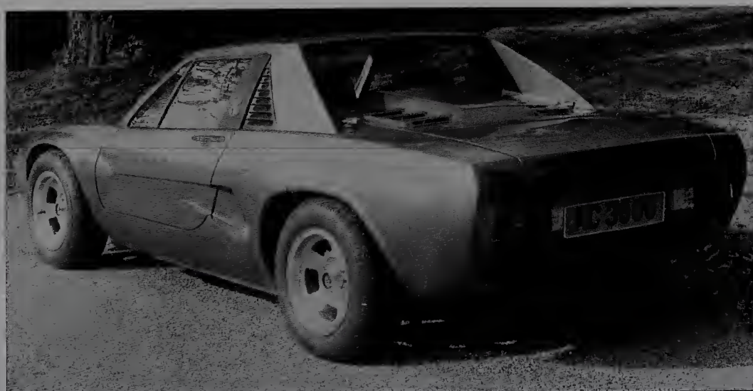
Chunky two-seater bodywork was made of glass-fibre.
