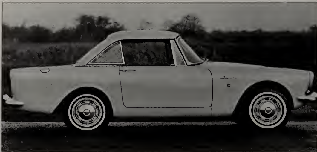
The tail fins were cut back for the Alpine IV, and the grille had a single bar.
