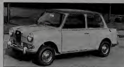
Mk III Hornet with concealed door hinges and Hydrolastic suspension.
