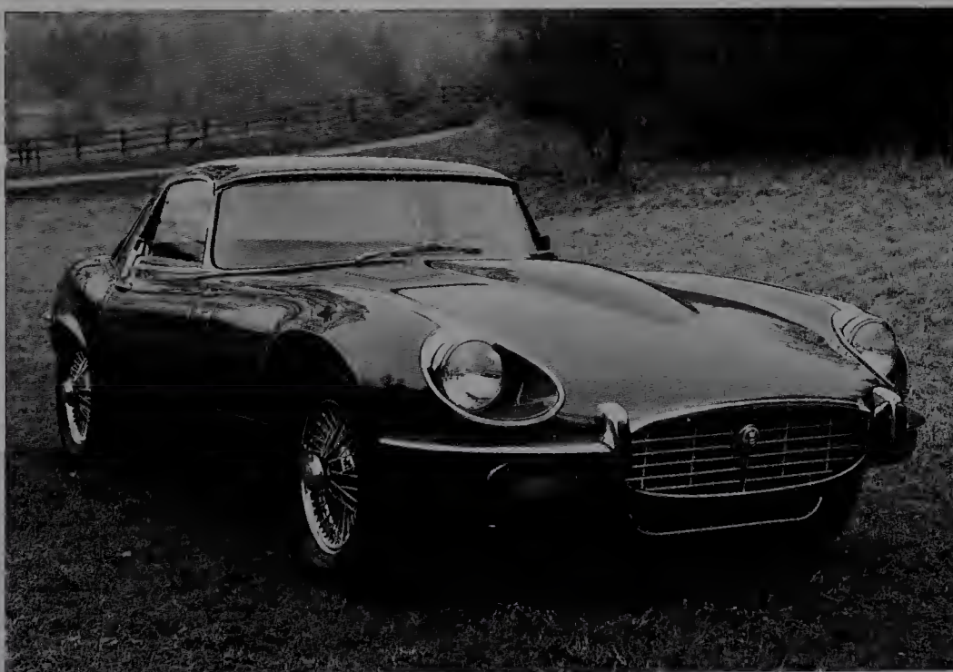
Series III with optional hard top and wire wheels.
