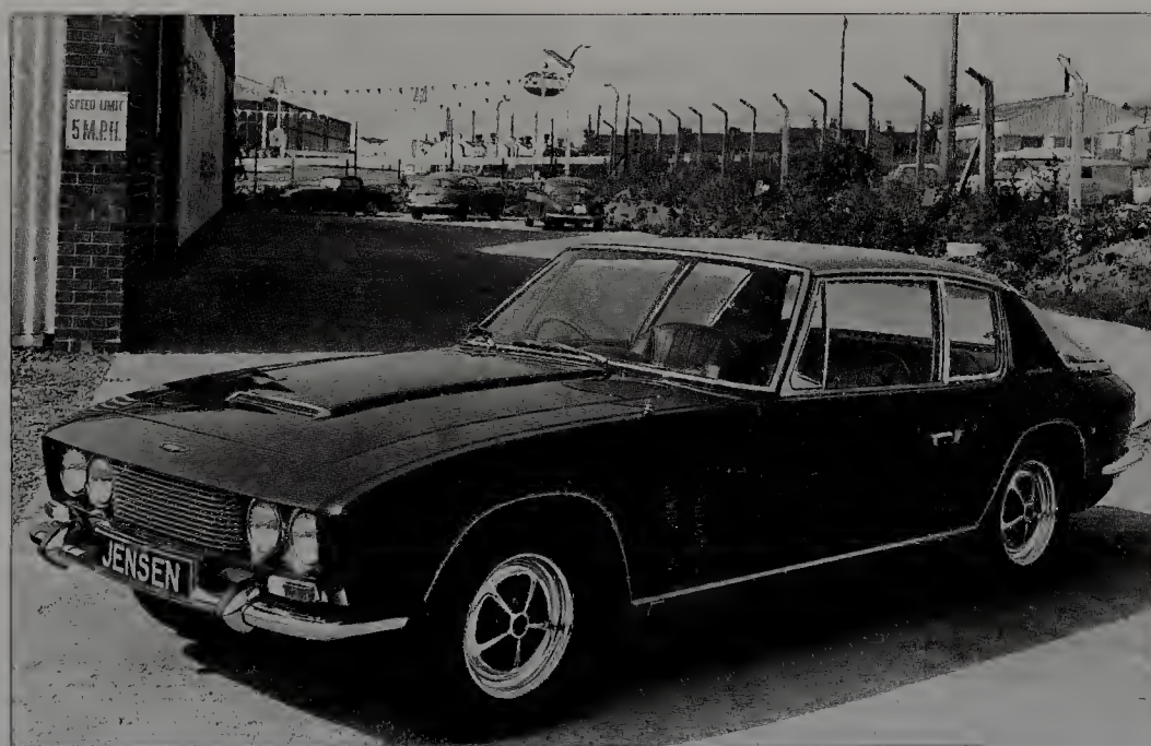
The four wheel drive Jensen FF, recognised by its dual side vents.
