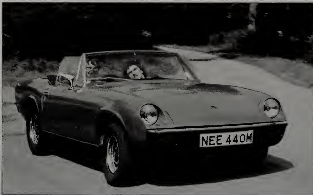
The 1972 Jensen-Healey Sports used a Lotus engine, Chrysler UK transmission and Vauxhall suspension.
