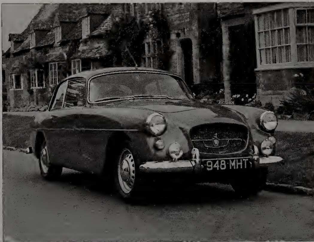
The 407 was the first Bristol to have a V8 engine, a 5.1-litre V8.
