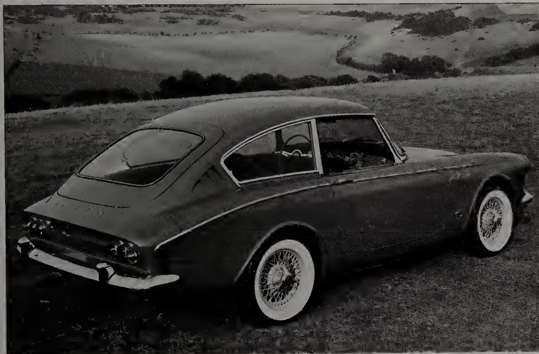
The Harrington Alpine Series B Le Mans, usually supplied with a 104bhp engine.
