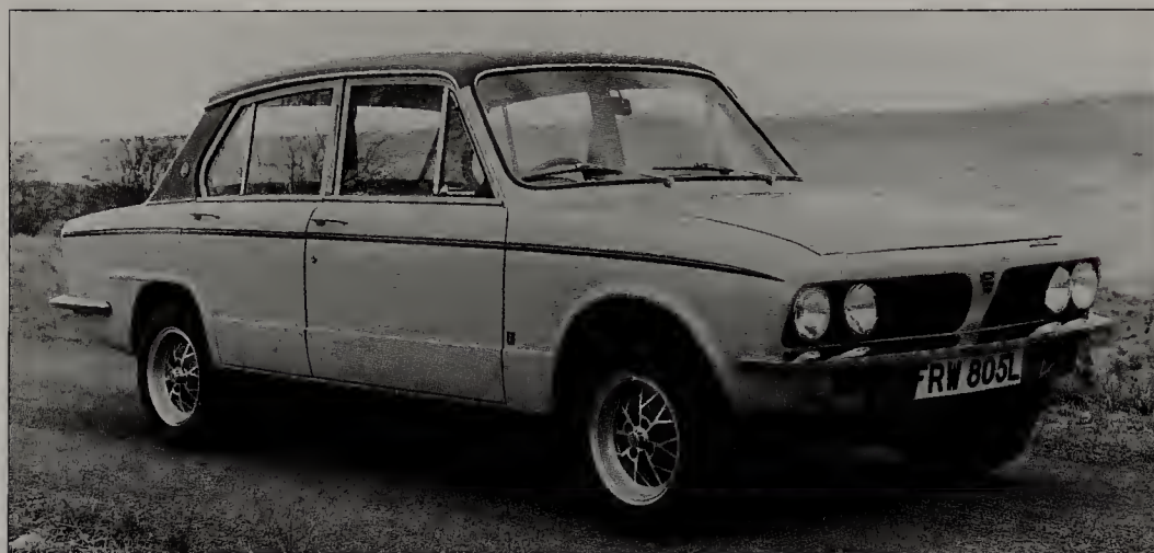
The 16-valve Dolomite Sprint, 1973, had 127bhp and alloy wheels.
