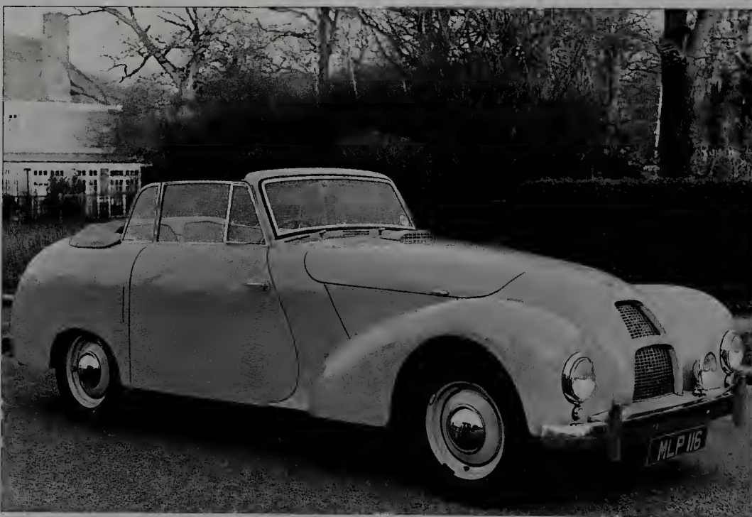
M2X Allard was a drophead version of the P1 saloon on a new chassis.
