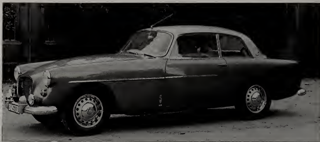
For the 1958 Bristol 406 the engine was enlarged to 2.2 litres.
