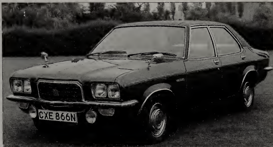
Ventora FE was the last model to use the 3.3-litre six-cylinder engine.
