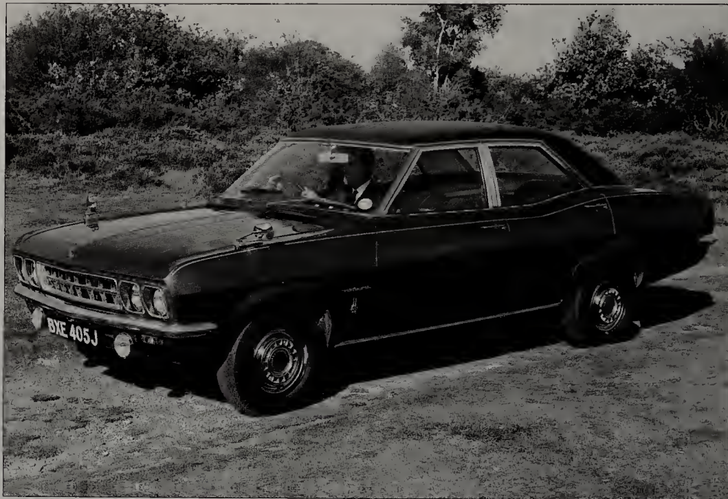
With the 123bhp 3.3-litre engine and plenty of torque, the 1968-72 Ventora was an effortless cruiser.
