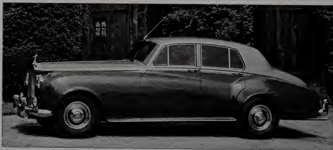
The 1959 Silver Cloud II was unchanged in appearance but a V8 engine replaced the previous model's straight six.
