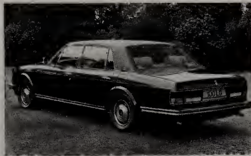
The Silver Spur had a longer wheelbase, and an Everflex roof covering.
