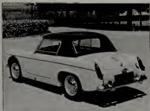
Mk I Midget with optional hard top and with its sliding side windows in position.
