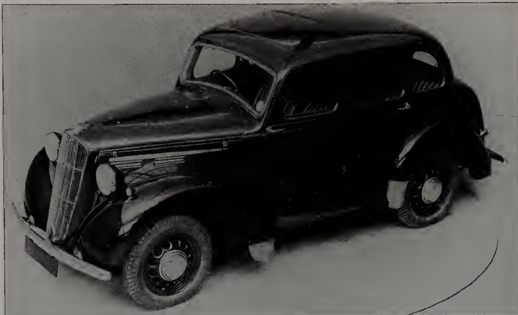
The Morris 10 Series M had an ohv engine and unitary construction.
