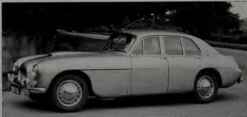
The 1954 405 saloon, powered by a 105bhp version of the 2-litre engine.
