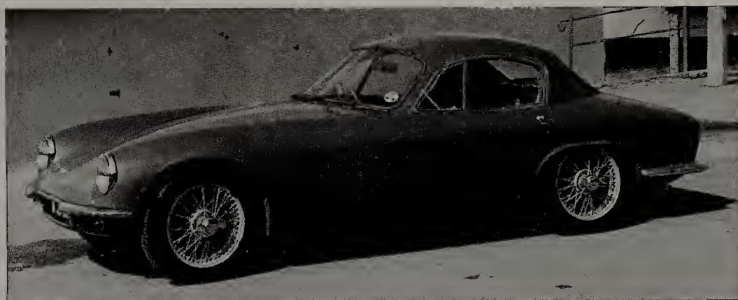
Lotus Elite, 1958, the world's first unit-construction glassfibre car.
