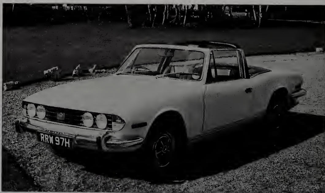
The handsome 1970 Triumph Stag. The T-bar gave extra rigidity.
