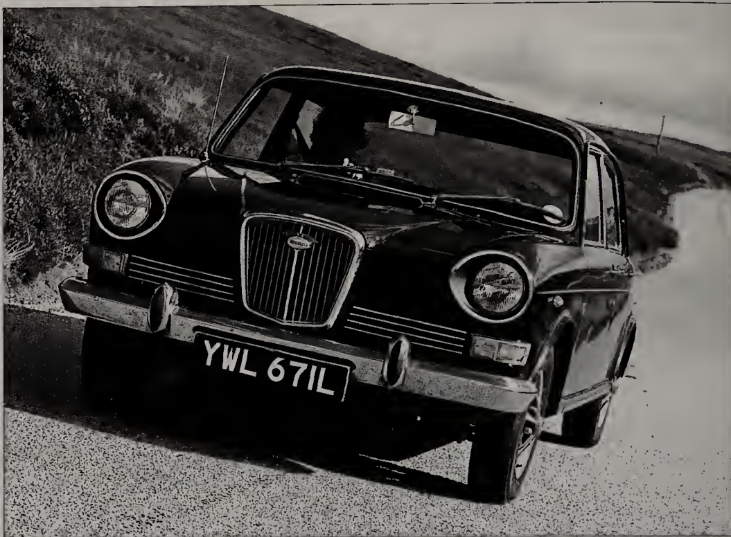
The 1972-75 Wolseley Six was wide enough to accommodate a transverse six-cylinder engine under the bonnet.
