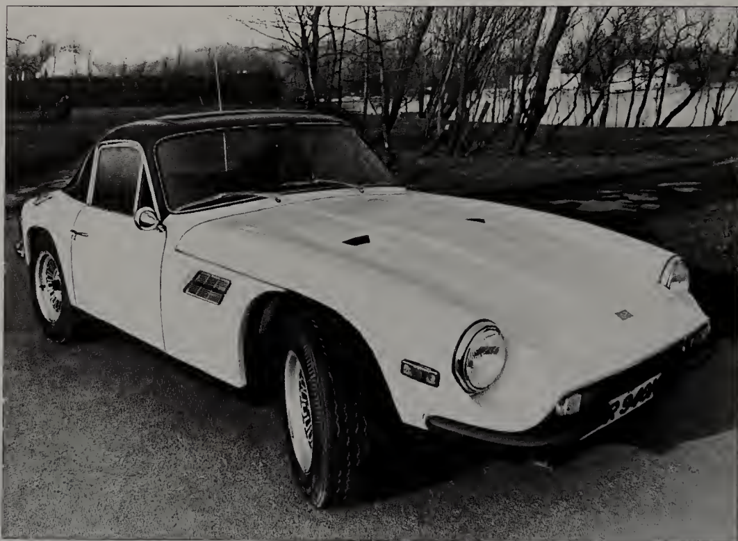
The 2500M had a new frame, a longer body and all-round independent suspension.
