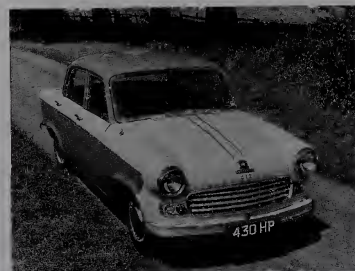
The Vanguard Luxury Six, 1960, had the body of the Vignale Vanguard with a 2-litre six-cylinder engine that was later to go into the Triumph 2000.
