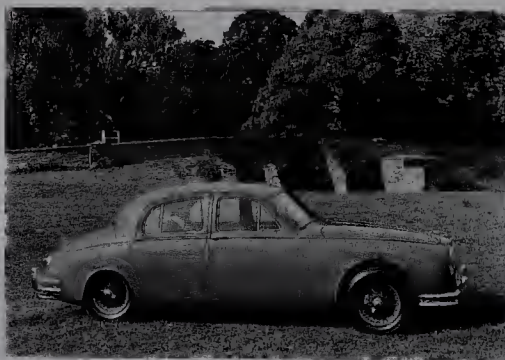
3.4 with wire wheels and cutaway spats.
