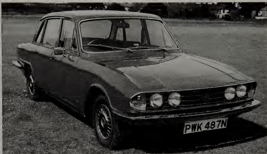
Triumph 2500TC, 1974. Twin carburettors replaced the 2.5 PI's injection system.
