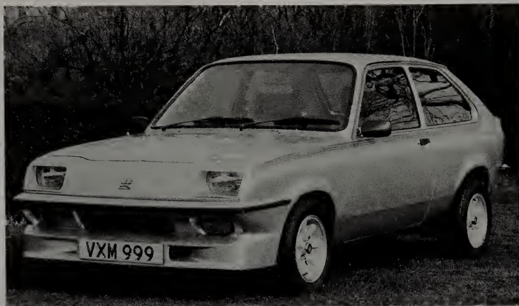
Chevette HS, 1976-79, was a "homologation special" with 16-valve twin-cam cylinder head and 135bhp.
