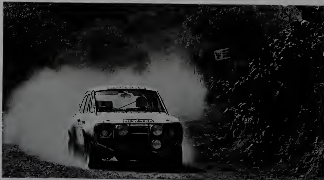
One of the 1970 World Cup Rally Escorts, car number 14, driven by Zasada and Wachowski. These cars were 1850GT "specials" with enlarged ohv Kent engines producing 140bhp.
