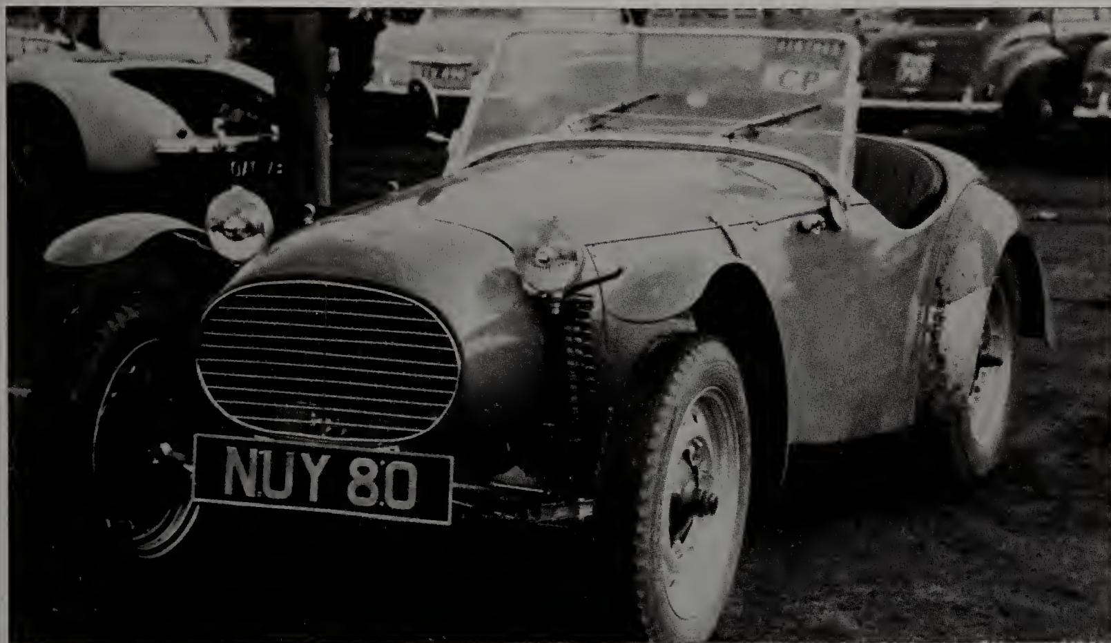
The Mk V Dellow had coil-spring front suspension.
