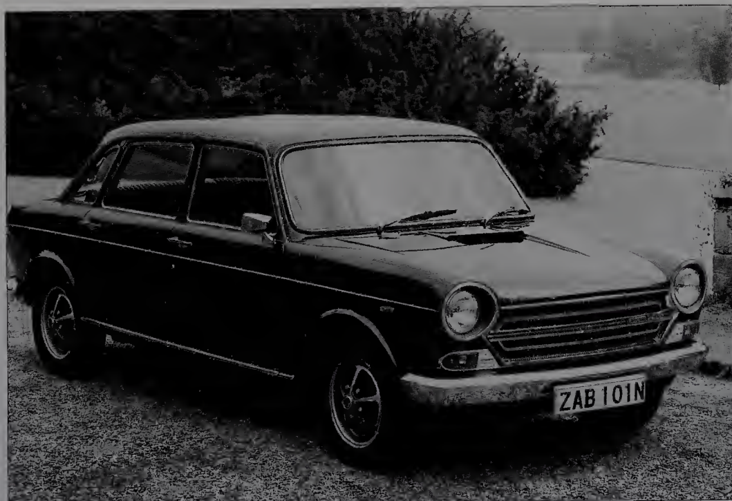
The six-cylinder overhead-camshaft Morris 2200.
