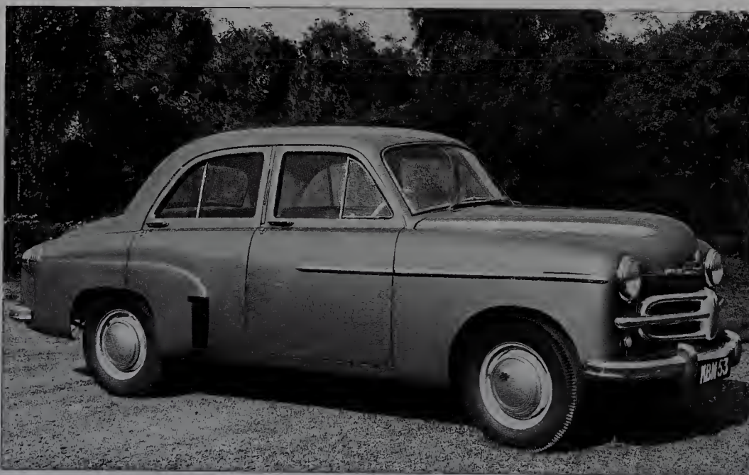
E-type Velox ran smoothly to nearly 80mph with the 1952-on short-stroke 2262cc engine. Its direct rival was the Ford Zephyr, whose engine was of the same capacity.
