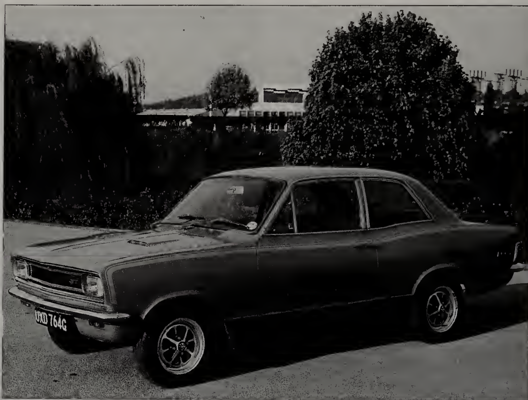
The 1968 Viva GT replaced the Brabham version. This time there were two litres under the bonnet, with 104bhp and a genuine 100mph.
