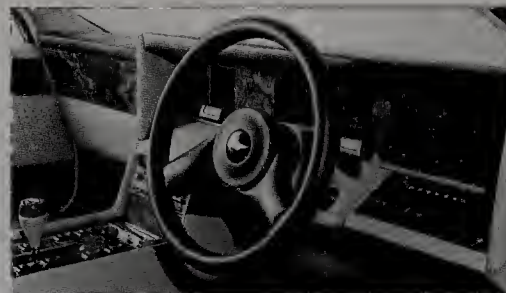
The Lagonda was first shown with this digital electronic dashboard.
