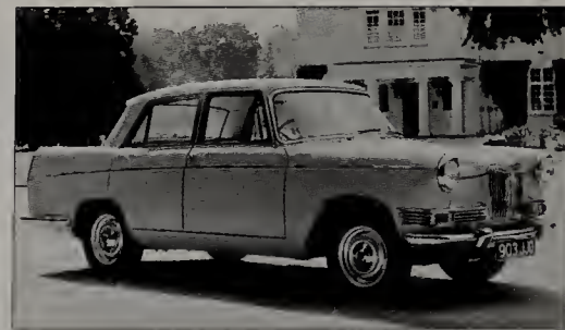
Riley 4/72, 1961, with 1622cc engine and widened track.
