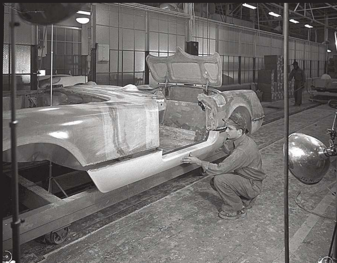
Above: An inspector at Detroit Forging examines the male and female molds for the new Corvette's upper front body panel in late spring 1953. This was the second largest piece on the car. GM Media Archive
