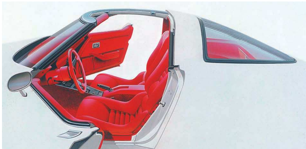
Left, bottom: The high-backed seat introduced in 1979 carried through 1980 and provided better lateral support. Engineers moved the fold-point higher up the seat back to improve access to rear storage. GM Media Archive
