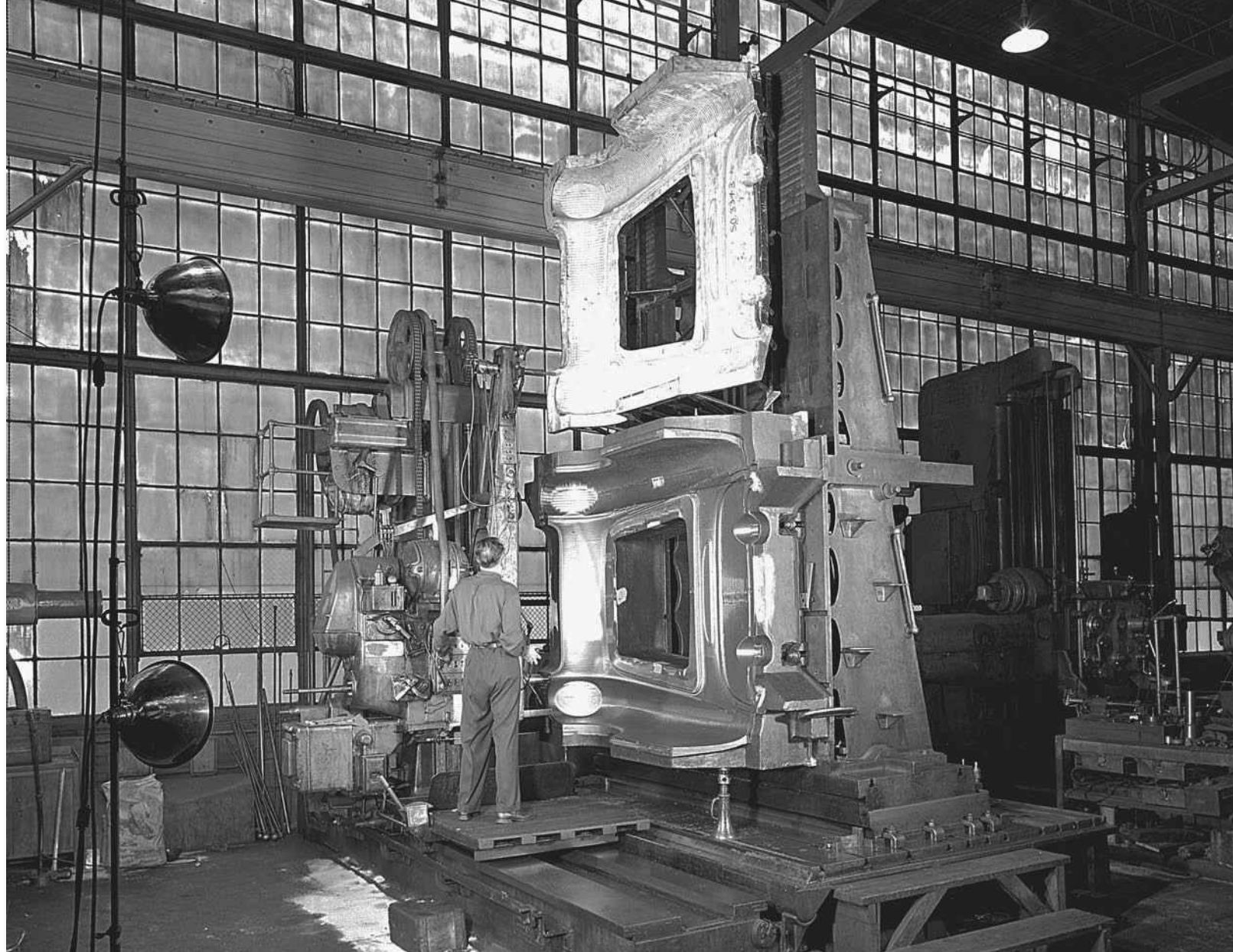
Above: An inspector at Detroit Forging examines the male and female molds for the new Corvette's upper front body panel in late spring 1953. This was the second largest piece on the car. GM Media Archive
