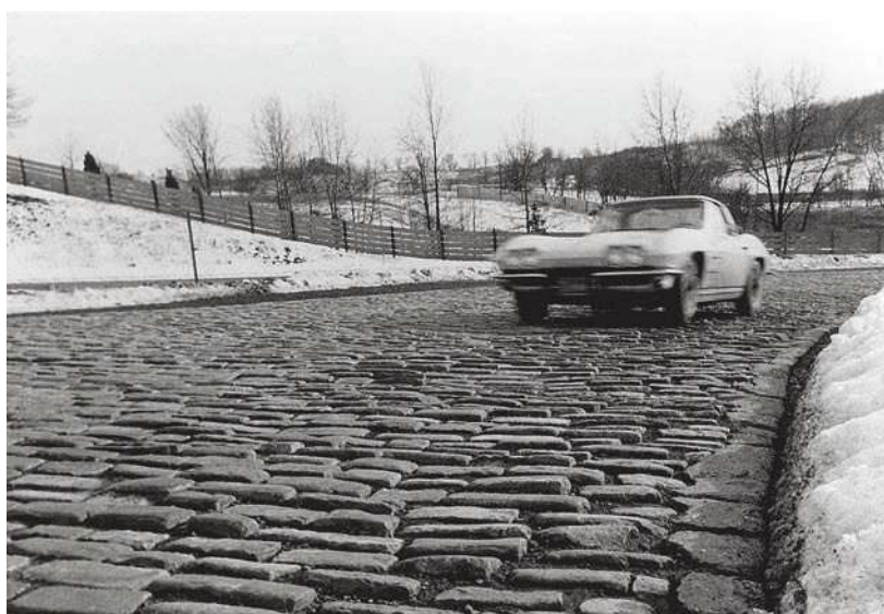
Above: Milford Proving Grounds engineering staff subjected 1964 prototypes to hundreds of miles on the "rough road." This test broke or shook loose components and electrical connections. GM Media Archive
