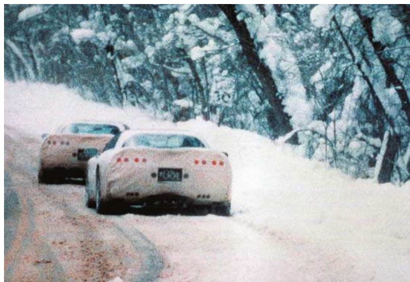
Left: After Chevrolet management committed to the body design for 1997, engineering fabricated functional running prototypes that they tested in all weather conditions from summer heat in Australia to winter cold in Michigan's Upper Peninsula. GM Media Archive
