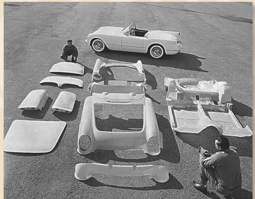
Fiberglas offered car designers many benefits such as lighter weight and lower manufacturing costs (the pressure molds cost a fraction of what matched-metal dies took to produce). In addition, it's likely the two men in this photo positioned each piece for the photographer without needing a forklift truck. GM Media Archive
