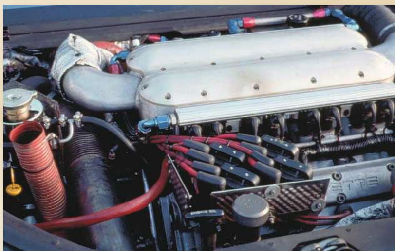
Above: When the Corvette Indy next appeared with all-wheel-drive and all-wheel steering, it was reconfigured as the CERV III. This powerplant, a twin-turbocharged 5.7-liter V-8, developed 650 horsepower. GM Media Archive
