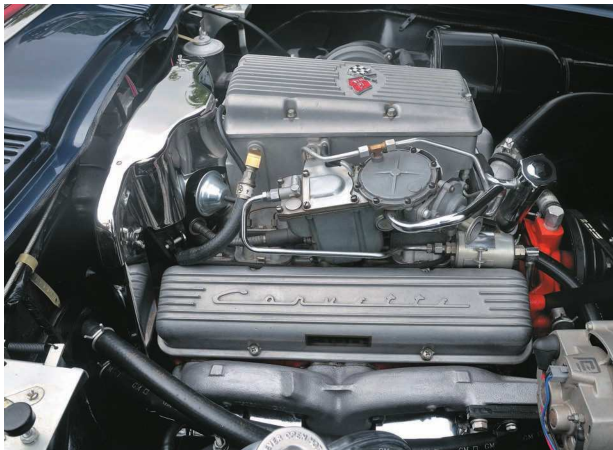
Left: Chevrolet carried over the base 1962 engine and transmission for 1963. However, they offered three optional powerplants ranging from 300- and 340-horsepower carbureted variants to this 360-horsepower, top-of-the-line fuel-injected version. David Newhardt © 2012
