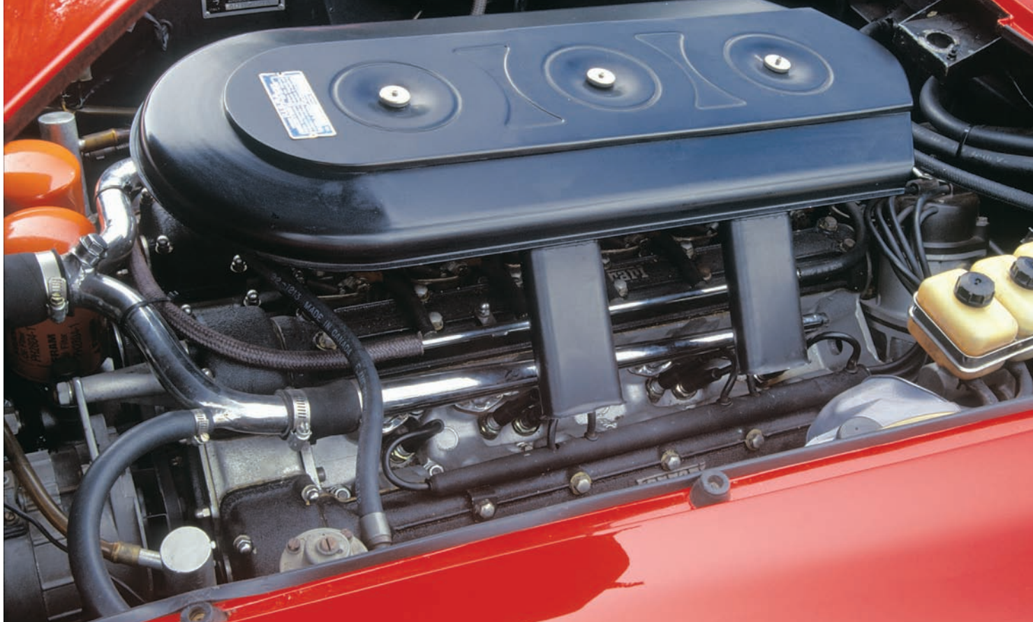
The Colombo-designed, sixty-degree, two-cam 275 GTB V12 had a swept volume of 3,285.7 cubic centimeters (273.8 cc per cylinder), and an output of 280 horsepower at 7,500 revolutions per minute.
