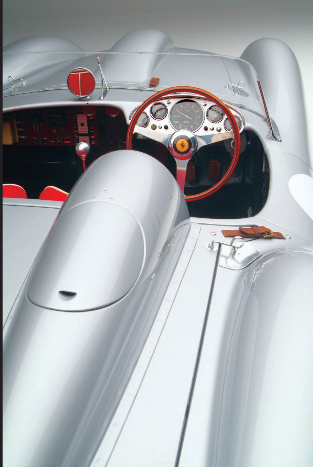
The driver's head fairing concealed the fuel filler, which was located beneath the cantilevered rear deck lid.
