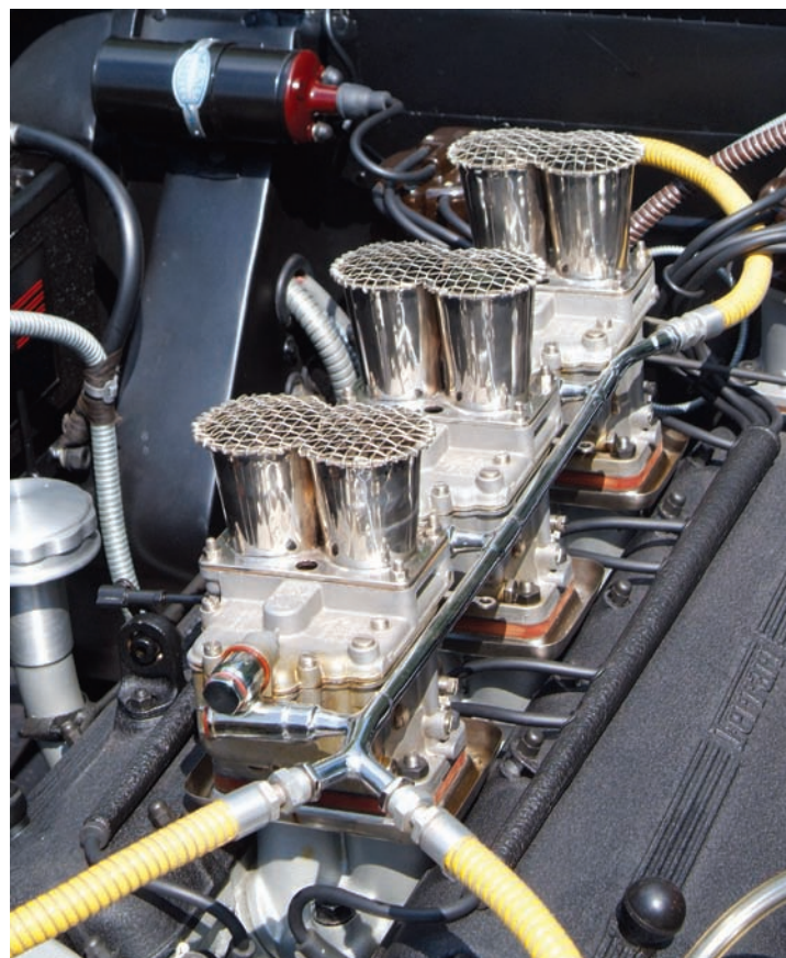
Under the hood, the Tour de France was all business with the 250 GT engine delivering 240 horsepower at 7,000 revolutions per minute. The V12 breathed through three Weber 36 DCF carburetors.
