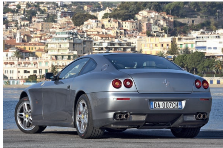
Ferrari's 612S Scaglietti is its largest-to-date Gran Turismo 2+2 coupe, replacing the previous 456 models. The 612's long wheelbase and overall length accomplished two primary goals; the first to allow front-mid placement of the 6.0-liter V12 (improving fore/aft weight balance and handling), and the second to increase leg and headroom for the rear-seat passengers. Michael Ward/Magic Car Pics
