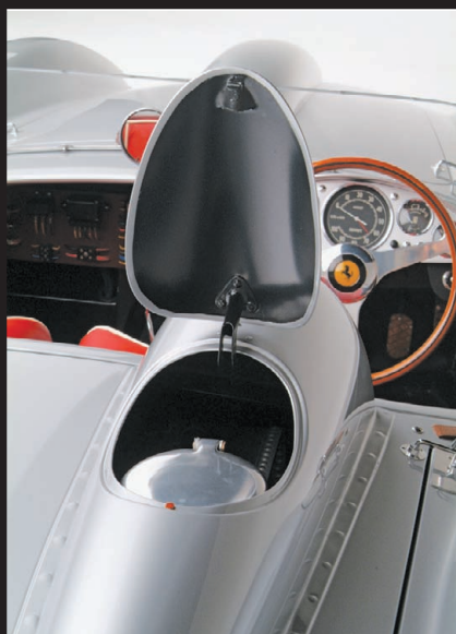
The driver's head fairing concealed the fuel filler, which was located beneath the cantilevered rear deck lid.
