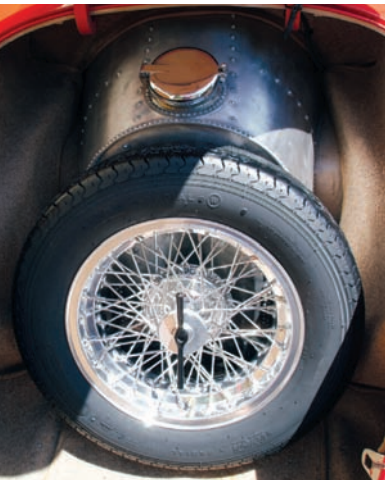
The spare took up most of the Barchetta’s trunk, and what was left was consumed by the fuel tank.
