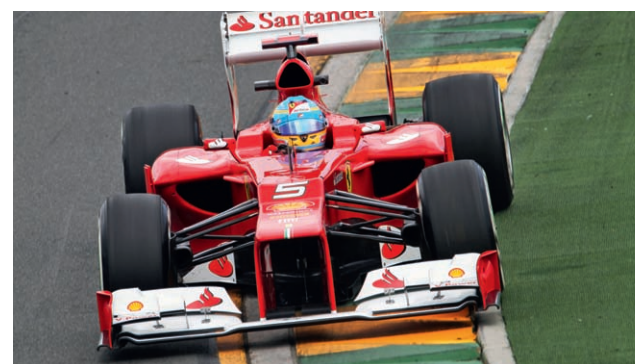
↑ The F2012's ugly stepped nose was typical of this year's crop of F1 cars, the result of poorly phrased technical regulations. Pullrod-actuated front suspension offered a lower center of gravity in this crucial area.
