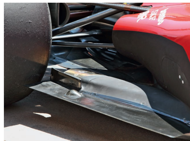
↑ The floor area at the rear of F1 cars became a focus of development as designers looked to use hot flow from the exhaust to accelerate airflow and boost downforce. Note the Ferrari’s wide and flat exhausts mounted flush to the floor.
