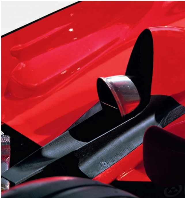
← Chimneys on the F2002's rear deck vented hot air from the radiators and used the hot exhaust gases to accelerate the flow, drawing out more air.
