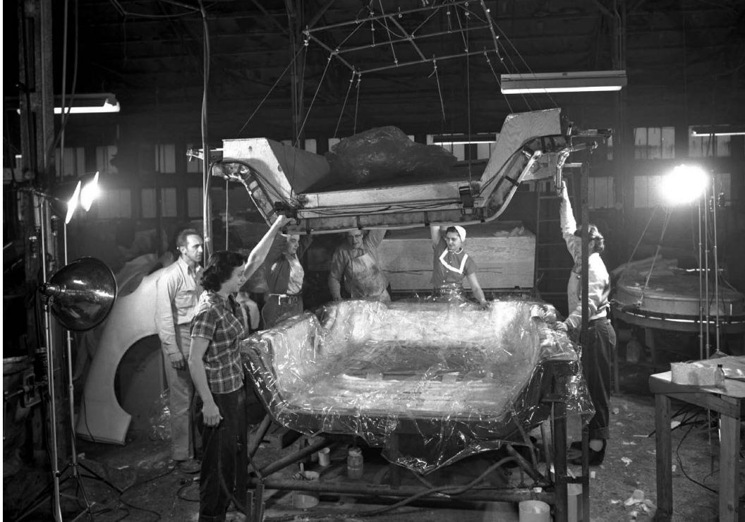
▲ Sandwiching the fiberglass-and-resin matrix between matching male and female molds, as shown here, produced smoother, stronger, more consistent parts compared with the hand-lay-up method used previously.
