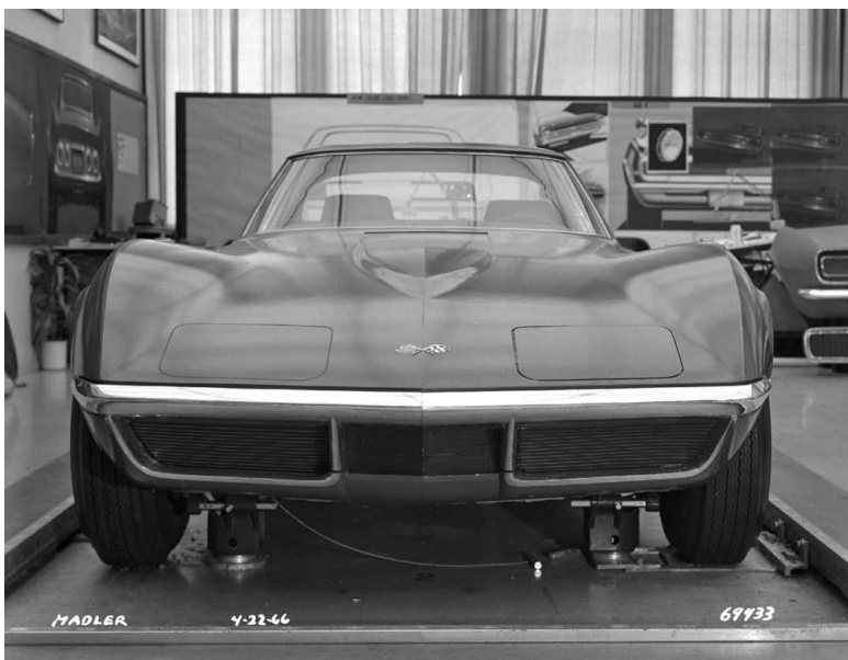
▲ (Both) Full-size, trimmed clay model, photographed April 22, 1966, is close to final C3 design.
