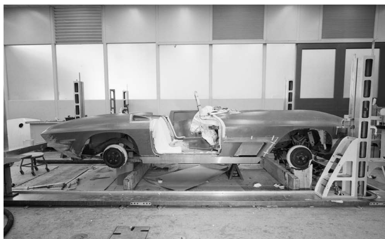
◀ Assembly begins for Mako Shark I , built with a newly conceived and fabricated fiberglass body and completely bespoke interior mounted to a production 1961 Corvette chassis.
