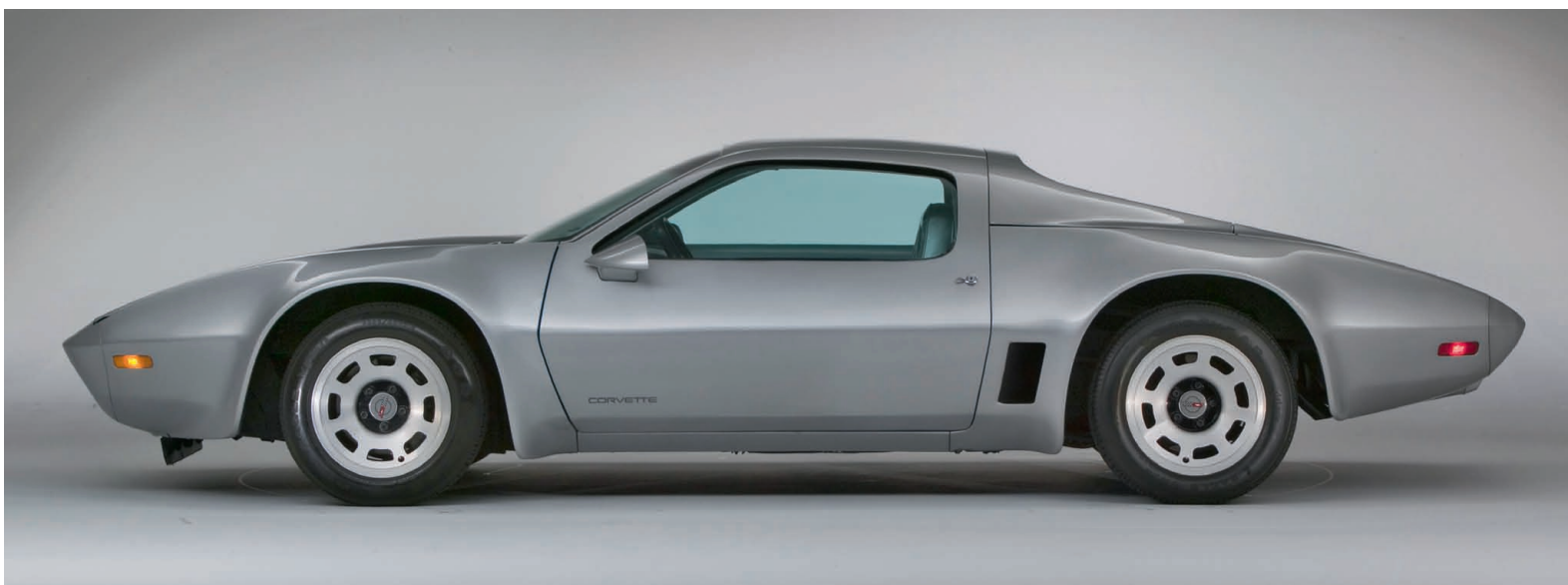
◀ XP-895 performance showed promise, but it was too heavy, due in part to a 1,150-pound (521.63-kilogram) steel body, so a new body was fabricated in 1972 using 2036-T4 aluminum, which trimmed almost 500 pounds (226.79 kilograms).
