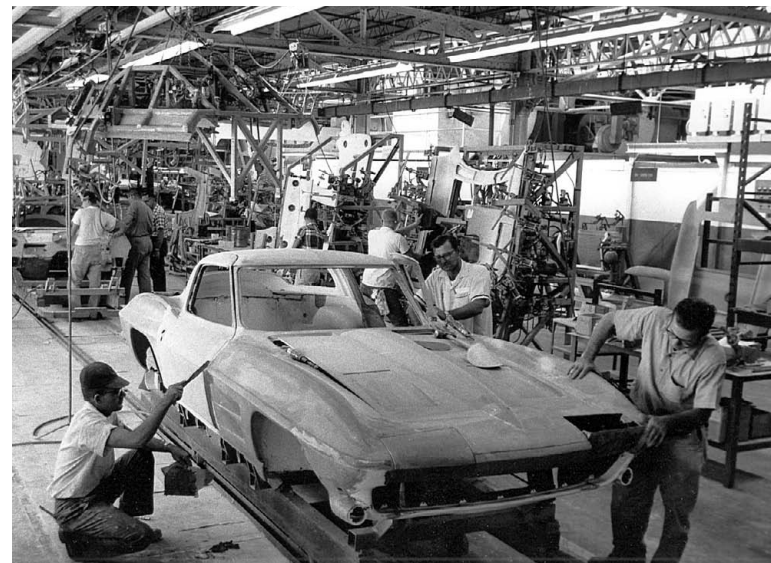
▲ C2 Corvette bodies were hand-assembled and finished, a labor-intensive process that sometimes resulted in erratic fit and finish.
