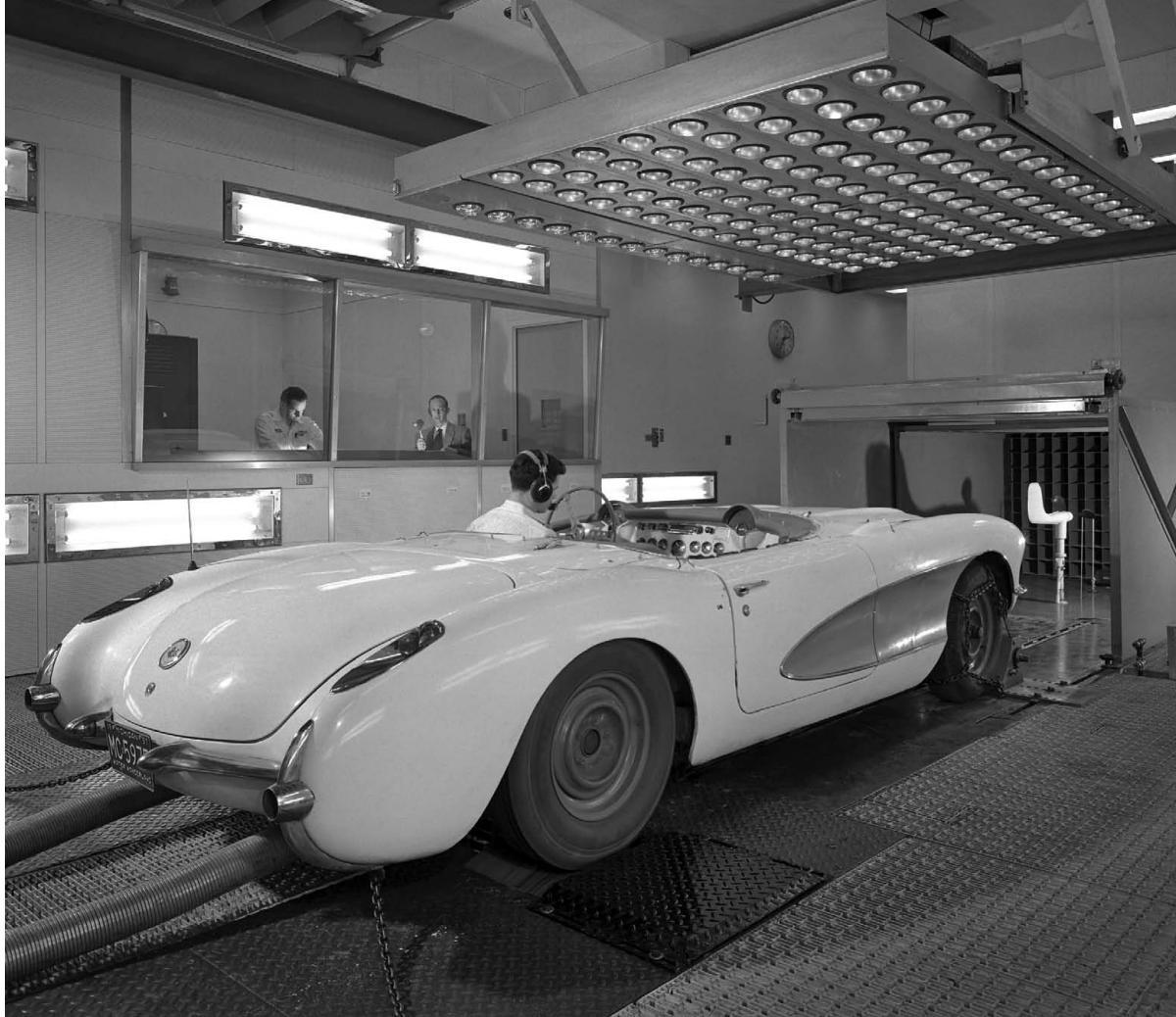
▲ A 1957 undergoing cooling system tests in a climatic wind tunnel was part of the complex, ongoing efforts to improve every aspect of Corvette's performance.
