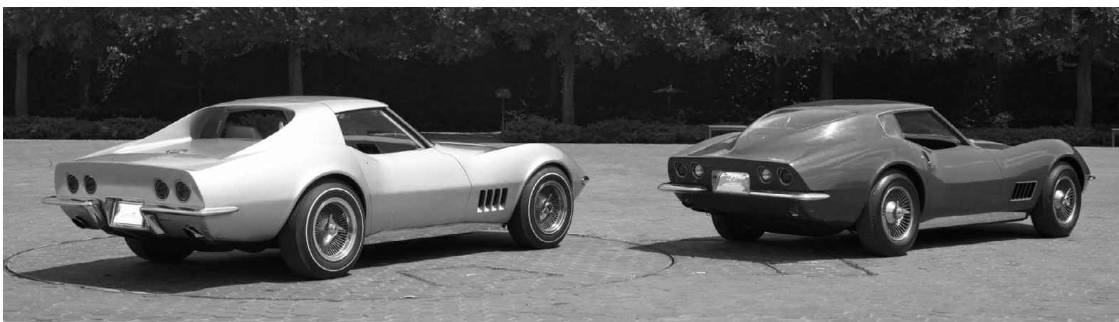
▲ Full-size clay looks halfway between Mako Shark II and final C3 production, with fender vent treatment similar to what was introduced in 1970 and door handle recess in quarter panel that resembles the door opening system for C6.
