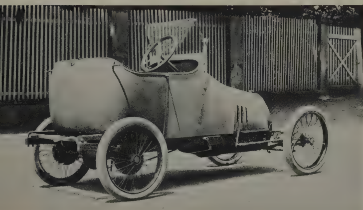
Same Type, different treatment. The smart Type 13 above is fitted with wings and a hood. The experimental car below is evidently later as it has wire wheels and rear suspension by reversed quarter-elliptics.
