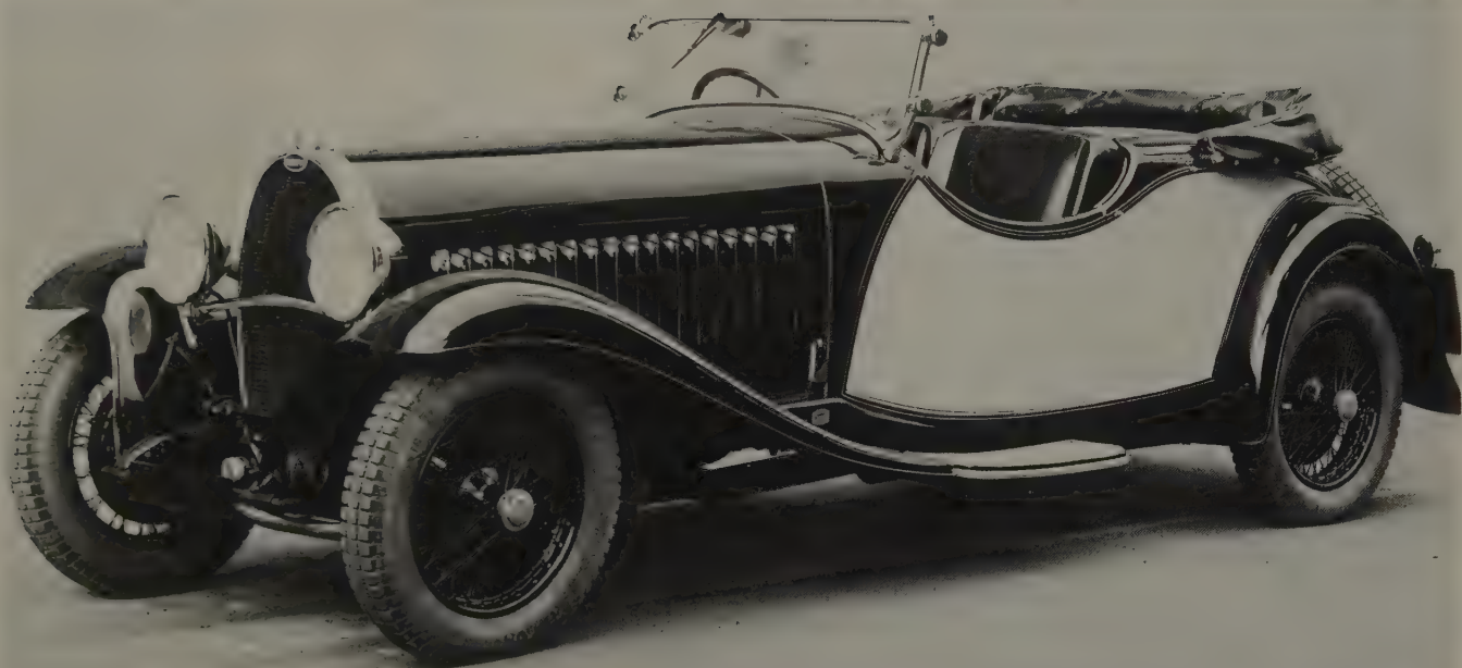
Gangloff too was enterprising when it came to body sides. The wing line is lightened by a broken running-board, which ends at the shut-line of the doors.
