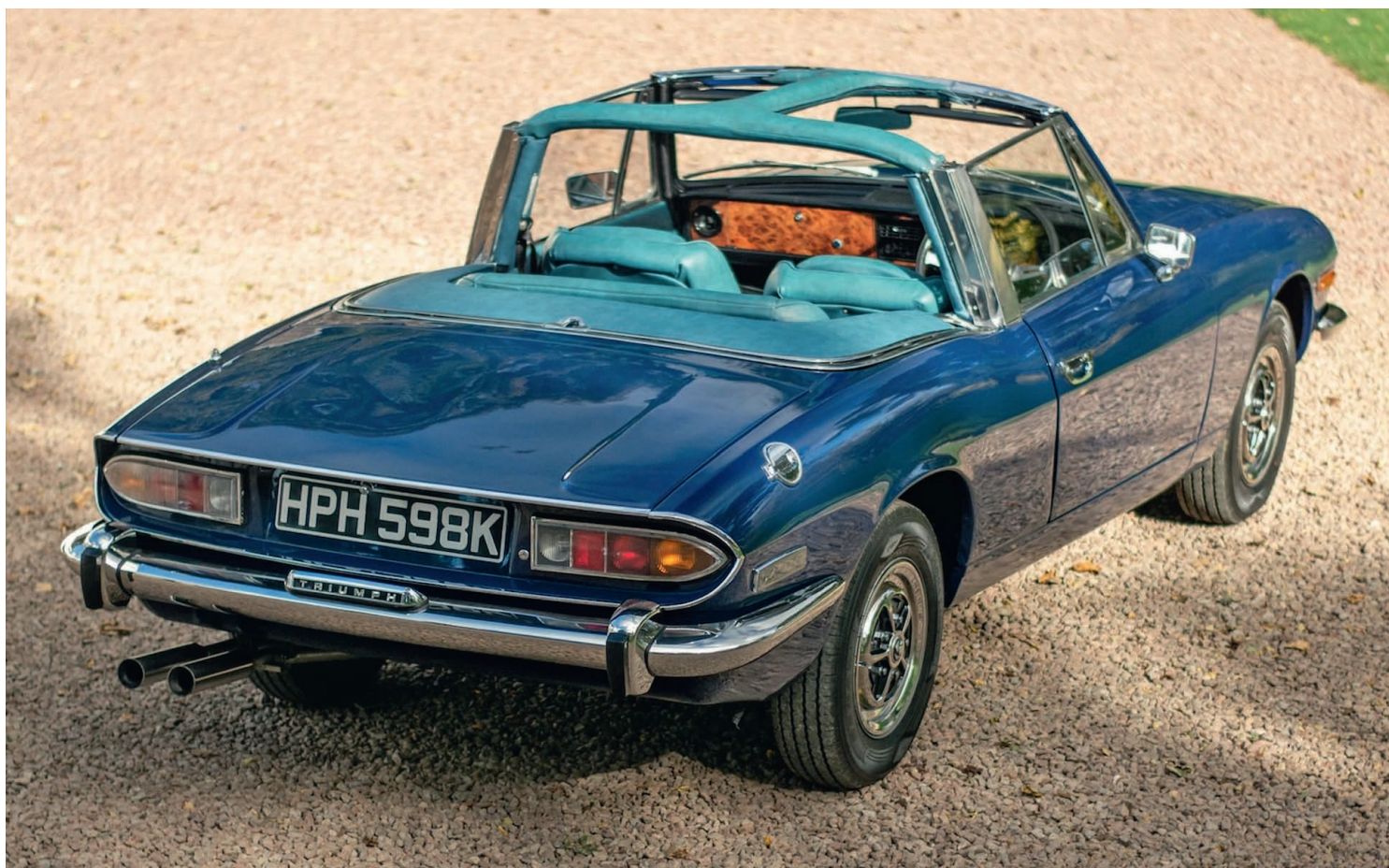
The defining feature of the T-bar helped to eliminate scuttle shake by significantly straightening the roofless car's structure.
