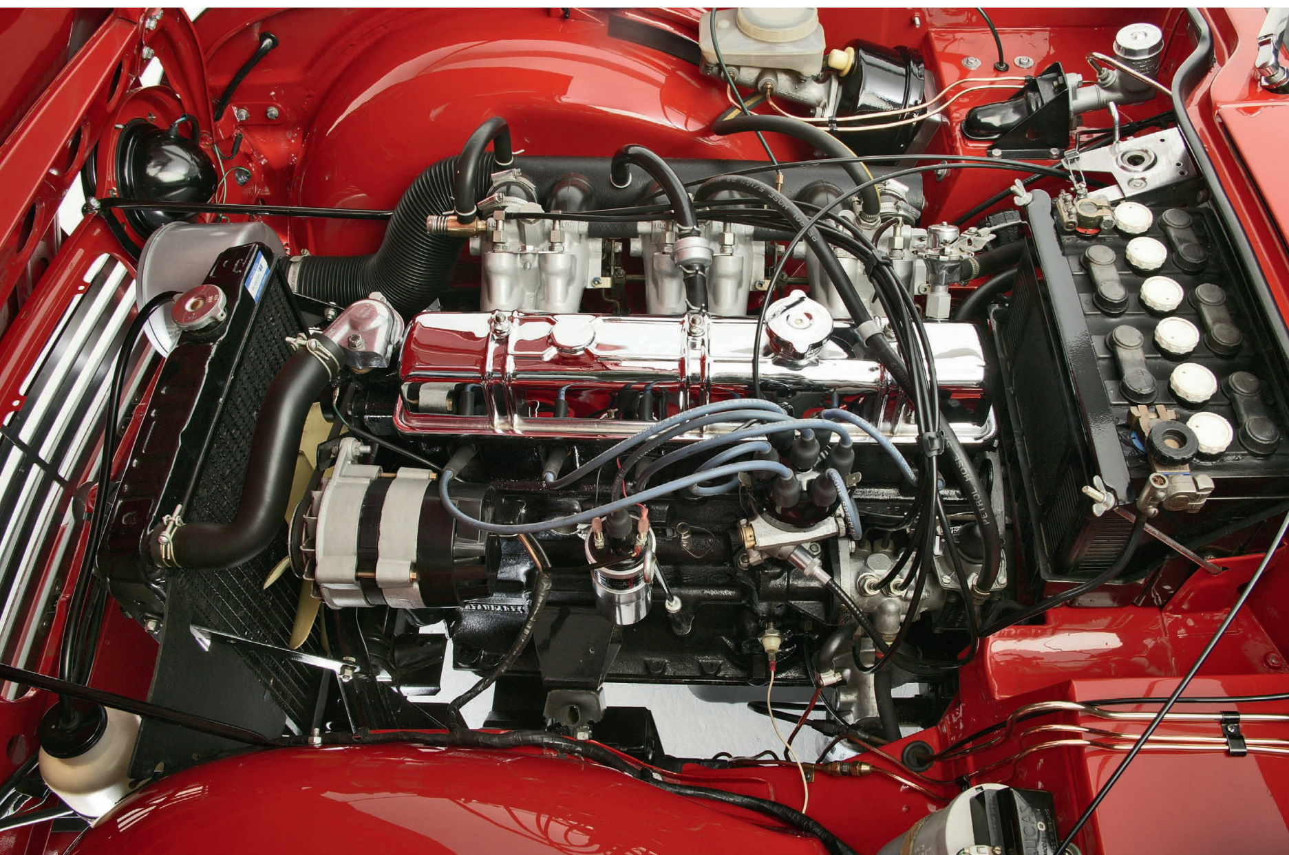
The six-cylinder TR5 engine in all its fuel-injected glory—good for a smoothly delivered, but decidedly hefty 150bhp and 164lb ft of torque!
