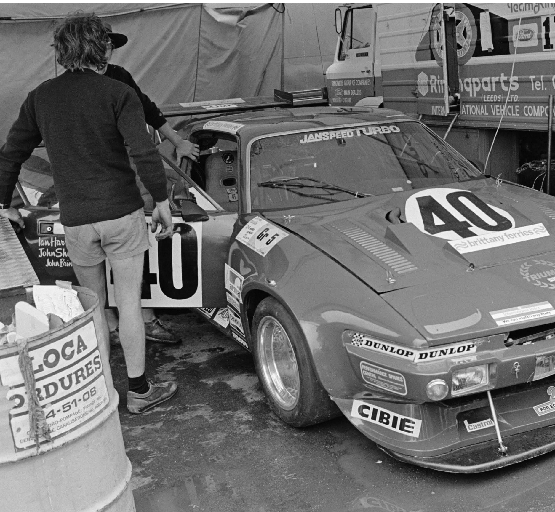
Triumph returned to Le Mans in the form of a 500+bhp, twin turbocharged TR8 model. Aided and abetted by wild aerodynamic accoutrements, and only lightly supported by the factory, it ultimately proved unsuccessful in both 1980 and '81.
