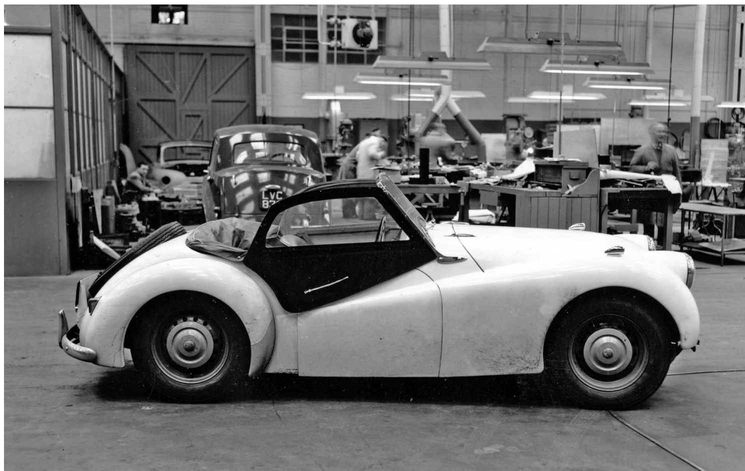
The bob-tailed 20TS prototype (here dirty after workshop testing) combined both modern and traditional design elements. The latter would disappear on the production TR2.
