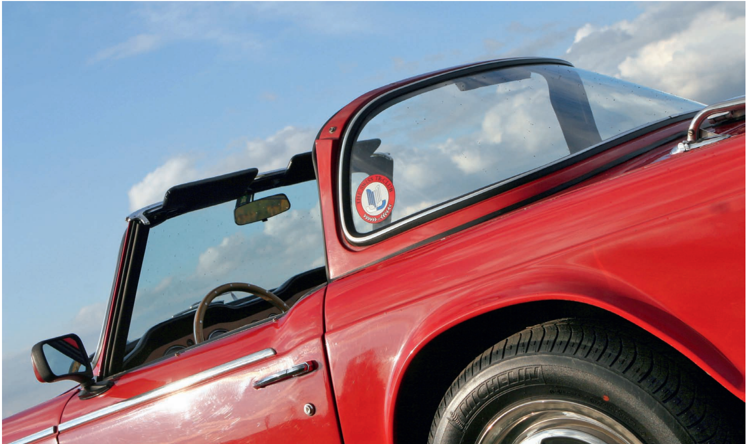
This image shows the metal center section of the unique roof design removed. Today, we would describe it as a 'Targa' thanks to Porsche's much better-known use of the design in later years.
