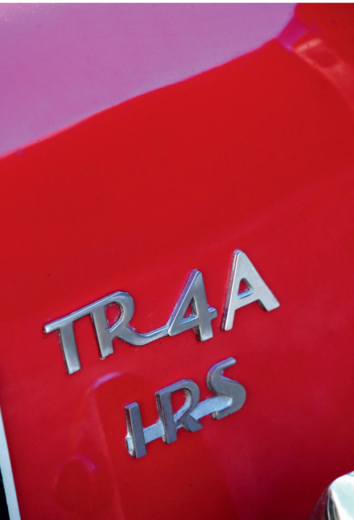
The letters IRS (on all U.K. cars, and some U.S. cars) below the model badge denotes the fitment of independent rear suspension on a TR4A.
