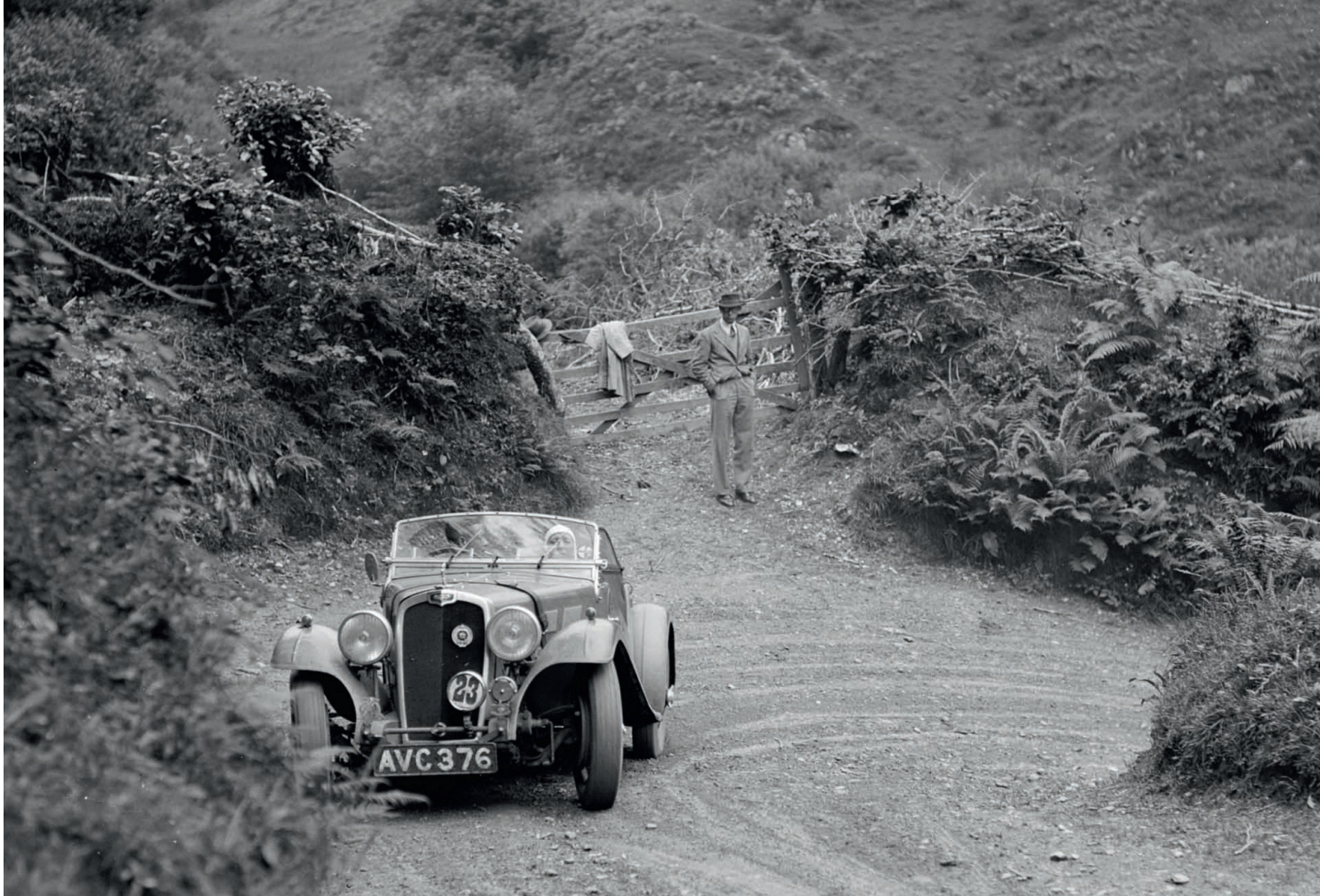
A two-seater Gloria Southern Cross sweeps around a corner on a motoring trial in Devon in 1935. With their shortened Monte Carlo chassis, they would prove adept little sporting cars.
