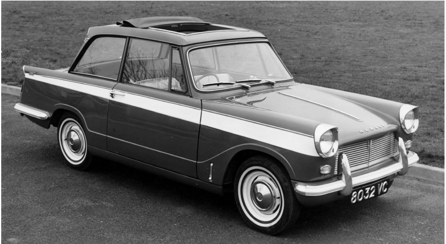
The Weathershields sunroof, fine mesh radiator grille (with no central pillar), and the off-white wheels mark this as an 'up-market' 12/50 model Herald. £56 more than a standard 1200 bought you a smoother transition and 28 percent more power.
