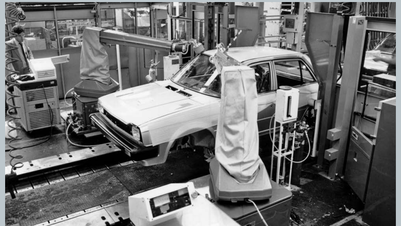
A significant proportion of the newly developed Triumph Acclaim production line comprised of automated construction, including an automated framing jig.
