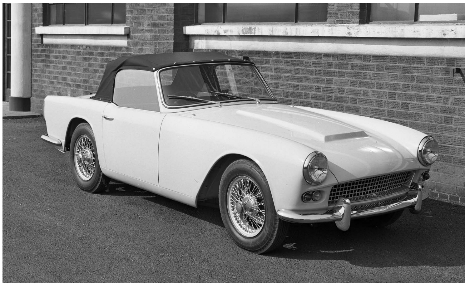
One of the 1959 Triumph TR4 Zoom Prototypes, which lent some of its physical attributes to the finished outline (most notably from the A-pillar back), has a distinct Ferrari look to its front-end.
