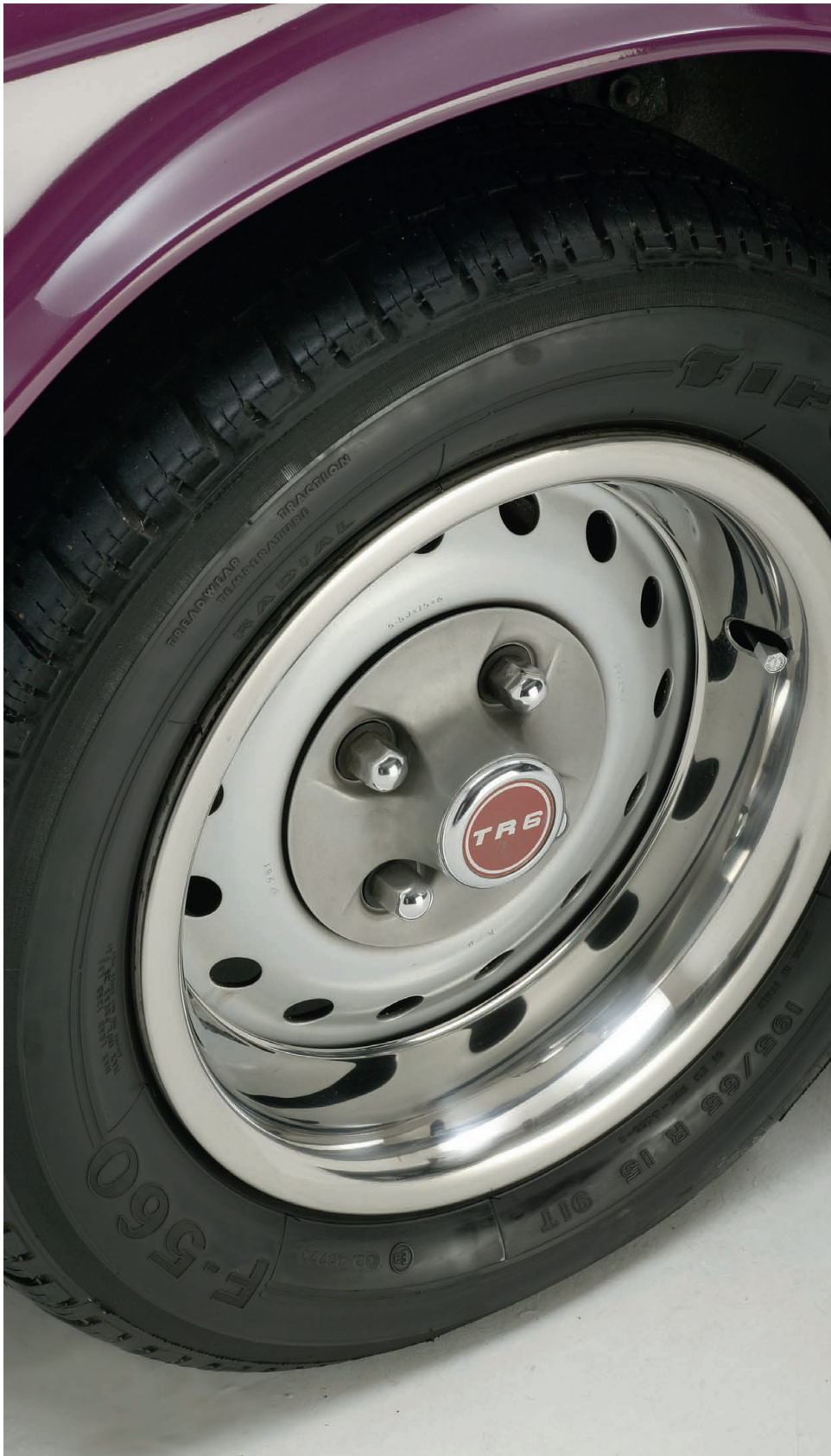
Perforated silver wheels quickly replaced the Rostyle trim items. Wire wheels, even if they somewhat fought against the modern look, remained an option.
