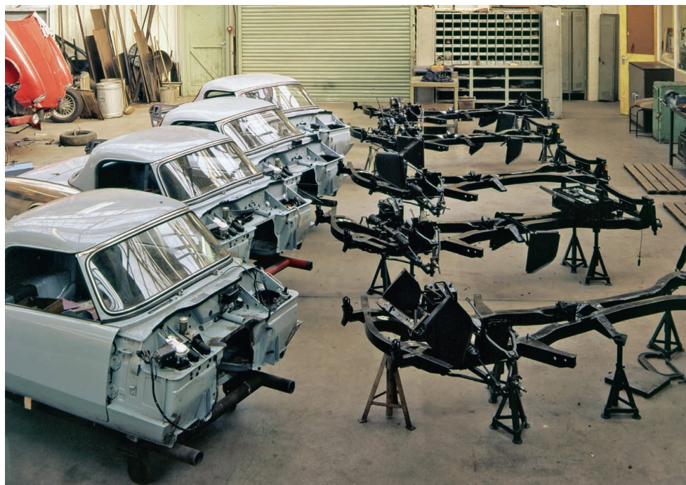
Spitfire 4 bodies and chassis await unification. The overall structure of the car proved surprisingly rigid.
