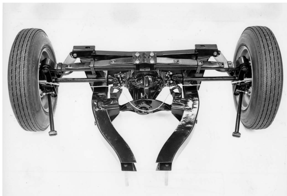
The uprated swing-axle suspension of the Triumph Spitfire MkIV. The GT6 model had received an improved set-up a full two years earlier.
