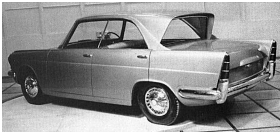
Project Zebu featured an interesting reverse-slope rear window. One problem though, unknown to Standard-Triumph, was that rival Ford had a very similar body design in the offing.
