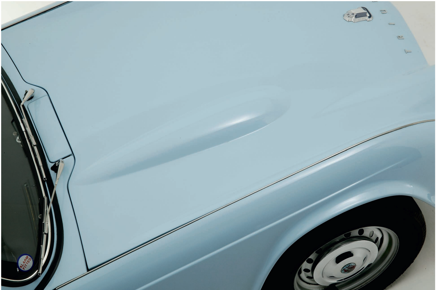
Bonnet bulge necessary to clear the twin carburetor set-up, which from 1962 saw the 'in-house' developed Zenith-Stromberg units replace the SUs of previous iterations.
