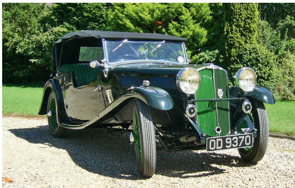
The Gloria Speed Model Tourer four-seater retailed for £285, but for an additional £40 the Gloria Competition Tourer had an identical spec with Telecontrol shock absorbers, a lighter frame, oversize Fort Dunlop tires, and a larger petrol tank with a quick release filler cap among the modifications.
