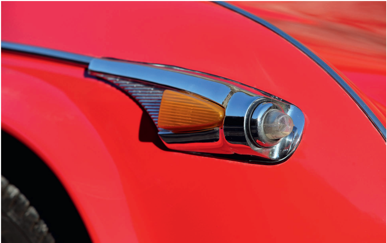
Innovative design combined sidelights (moved from their original positions on the grille) and indicator repeater lights.
