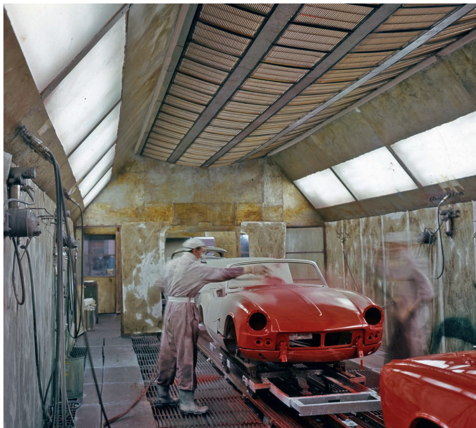
Spitfire 4 bodies in the paint shop at the Canley factory. Their achingly pretty outlines proved attractive to buyers from the start.
