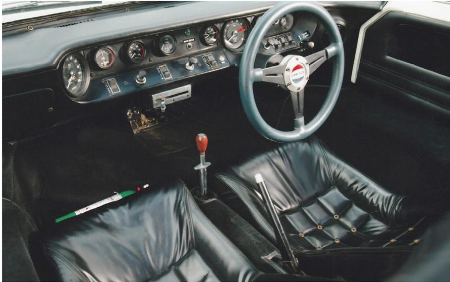
*Interior of the Mark III. Note that the gearshift has been moved from the right to the middle of the cockpit, as is usual for street cars. (Courtesy Graham Robson)*
