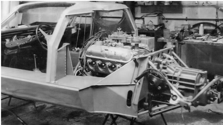
*The 4.2-liter aluminum engine and Colotti gearbox installed. (Courtesy Lola Archives)*
