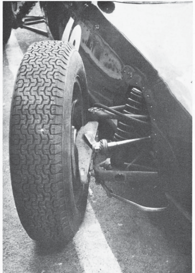
BRM front suspension is another example of the craftsmanlike construction of the Bourne cars
