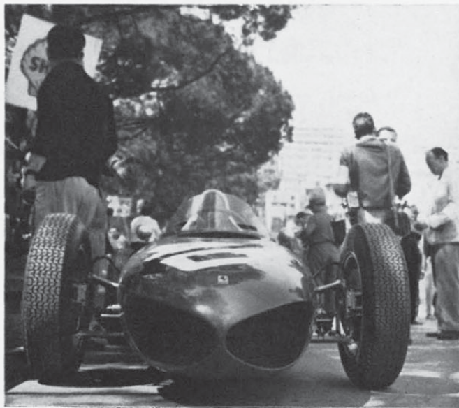
In this frontal view of the Ferrari the negative camber of the front wheels is shown to be excessive by normal standards. The frontal area is very small when compared to previous Ferrari single-seaters
