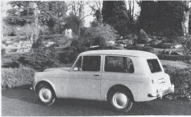
The 1954 prototype with all-glass-fibre station wagon body, the back of which foreshadowed styling adopted by some popular models several years later. The engine is now at the front, carried by a sub-frame detachable from the narrow, ladder-construction platform frame which has replaced the simple tubular chassis member. The photograph was taken at Mr. Ferguson's home at Stow-on-the-Wold
