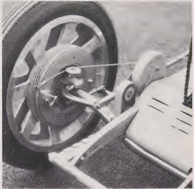
*Right: The front brake operation was by cable along the lines of the later Brescia and T30 cars.*
