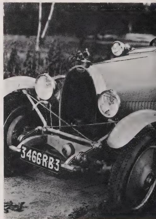
The T40 1½ litre 4 cylinder car was introduced in 1926 to replace the Brescia. It combined the road manners and driving charm of its larger and faster sisters, but at a surprisingly modest price, about a third of the racing model T35. The first series had a Brescia frame, but soon the chassis was lengthened and strengthened, and the standard factory body was this Grand Sport. Here is Maurice Phillipe, one of France's best known motor journalists of the period.
