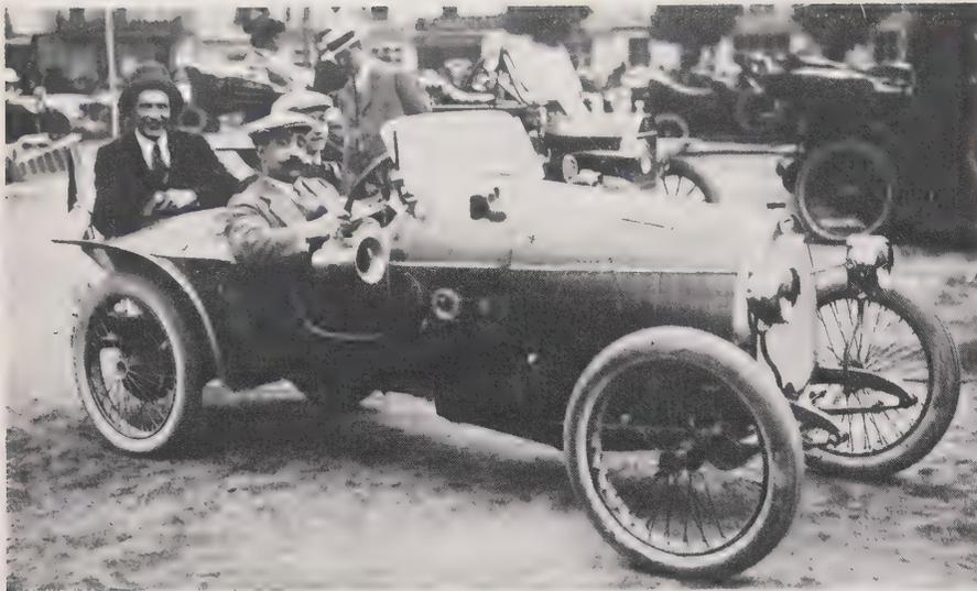
*The 1913 model with rounded radiator; a meeting at Tours. The body seems to be wood-decked, and riveted.*
