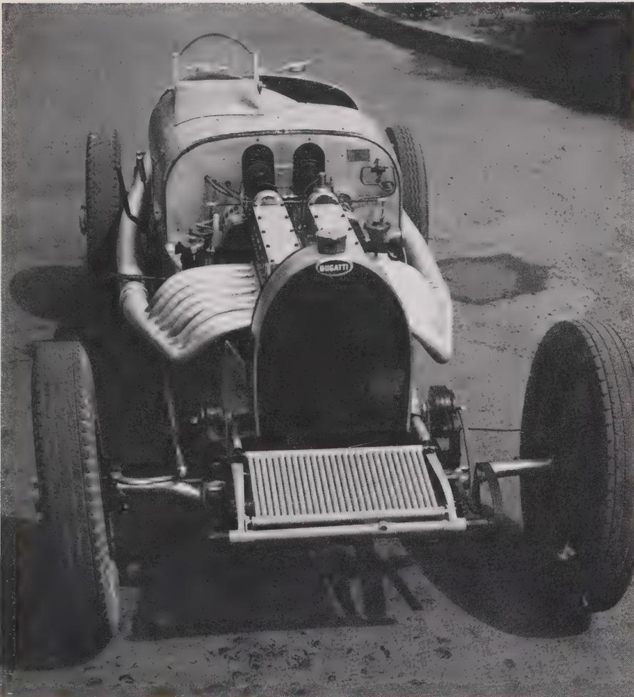
*The 16 cylinder car, twin exhausts and an oil cooler in front.*
