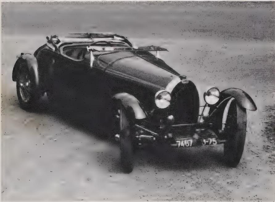
*The Type 38 replaced the T30 as the normal 8 cylinder touring model, still 2 litres. The engine was similar both to the T30 and the later T35A. The radiator is now flat based, and the gearbox was new, with a more conventional gear change, first gear being forward, and top back. It was successful enough with light coachwork, but really needed more power.*
