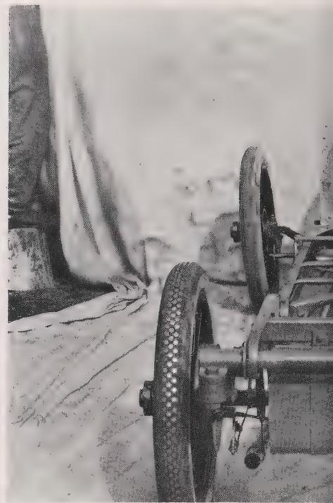
The 1913 chassis now had the reversed rear quarter elliptic springs and an improved oiling system.
