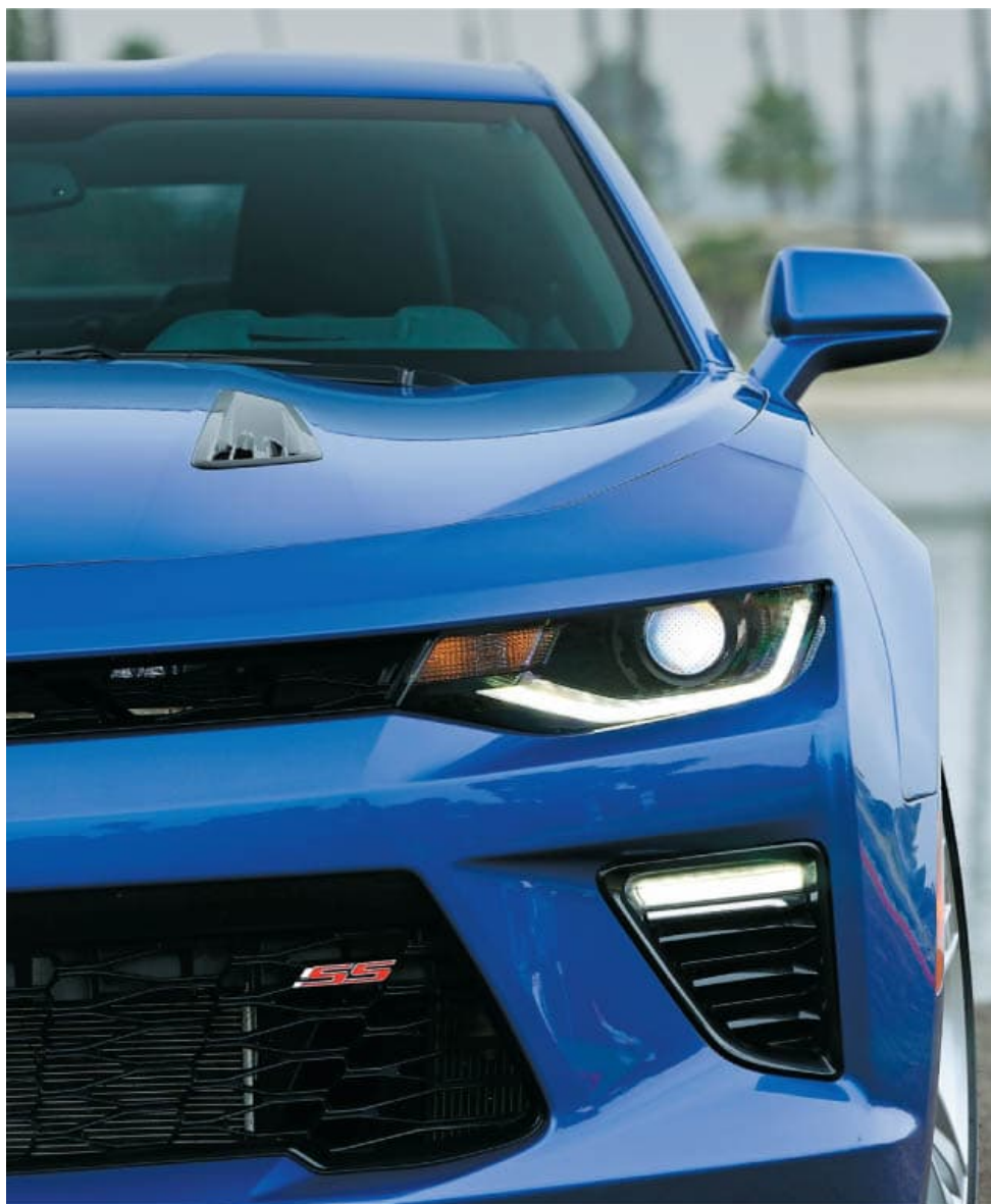
The 2016 Camaro SS uses horizontal daytime running lights (DRL) in its aggressive front end. Camaro RS models use tall, vertical DRLs. Hood vents are unique to the SS model.
