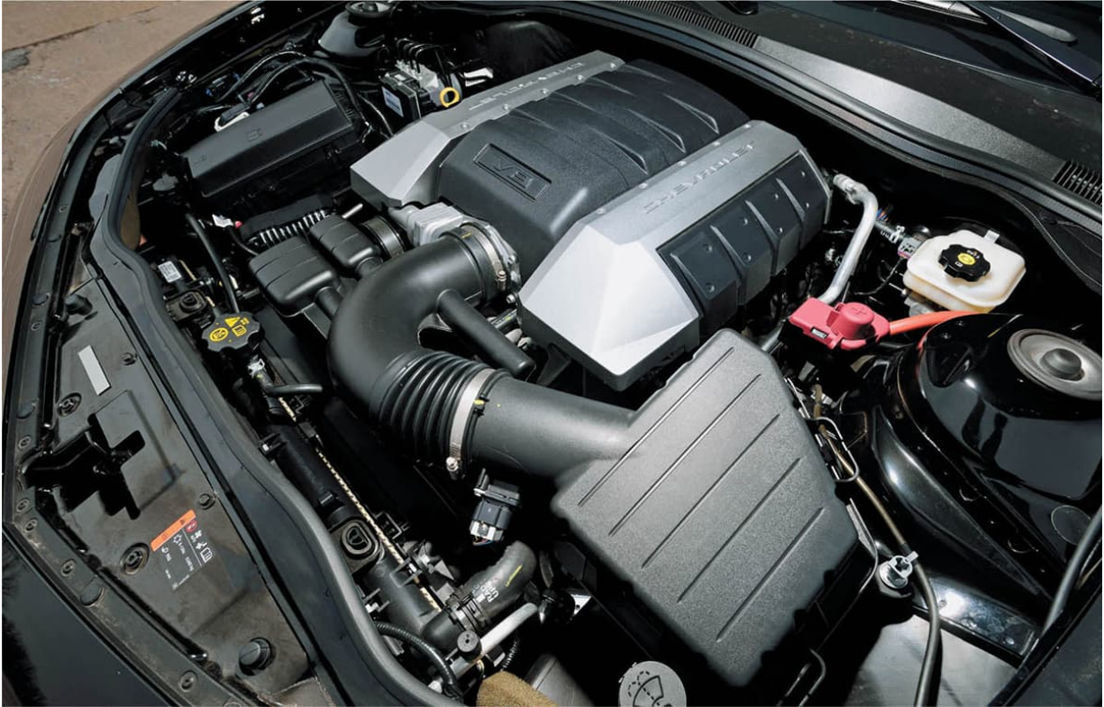
The LS3 6.2-liter engine in the 2014 Camaro Pace Car edition uses an aluminum-block, alloy L92-type rectangular-port heads, a high-lift hydraulic camshaft, and 10.7:1 compression to generate 400 horsepower.
