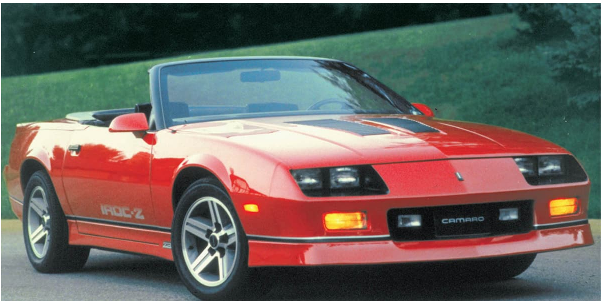
IROC-Z buyers received a detuned version of the Corvette's 350-cubic-inch V-8 that generated 220 horsepower. General Motors 2012
