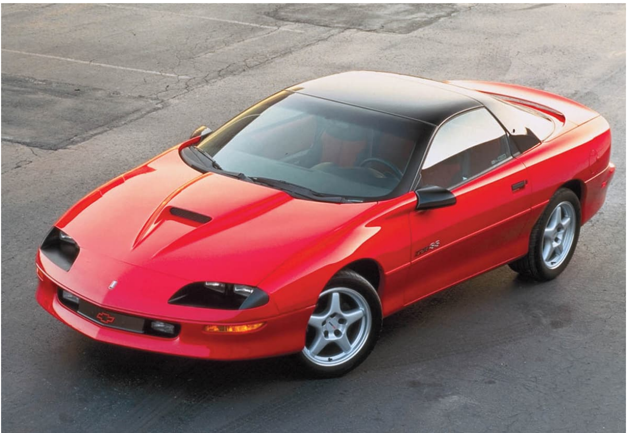
The scoop on the 1996 Z28 was functional. General Motors 2012
