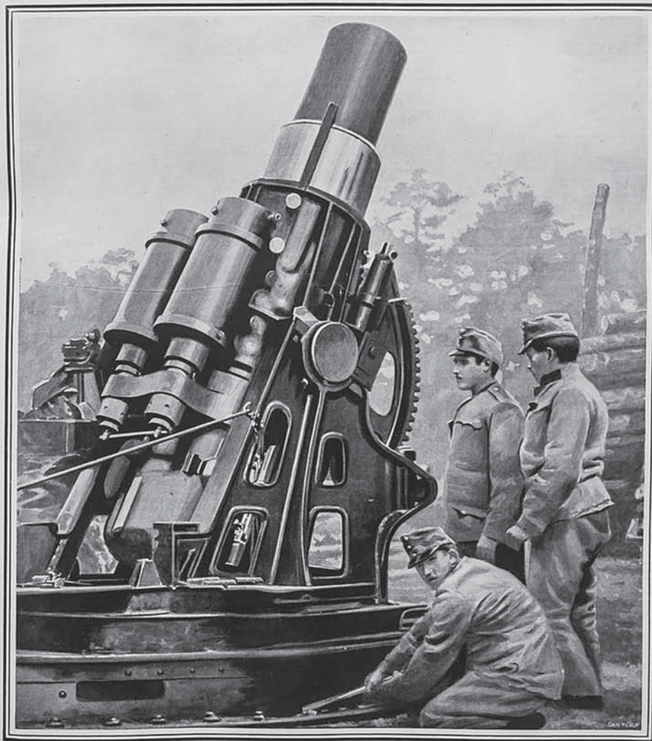
AN ENEMY WEAPON WHICH FIRES A SHELL WEIGHING OVER 1000 LB.: THE GREAT 12-INCH SIEGE-HOWITZER OF THE AUSTRIAN ARMY.
