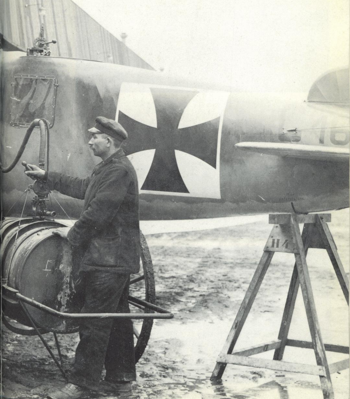
68. An LFG Roland CII 'Walfisch' being refuelled. This flying school machine lacks armament but still retains all the fittings for the two machine guns. Produced as early as 1915, the Roland exhibited many features ahead of its time: a semi-monocoque fuselage, simple 'I' struts, faired-in wing roots and large celluloid fuselage windows to improve visibility. The device on the upper wing between the men is a crash pylon. (Bruno J. Schmaling Collection)
