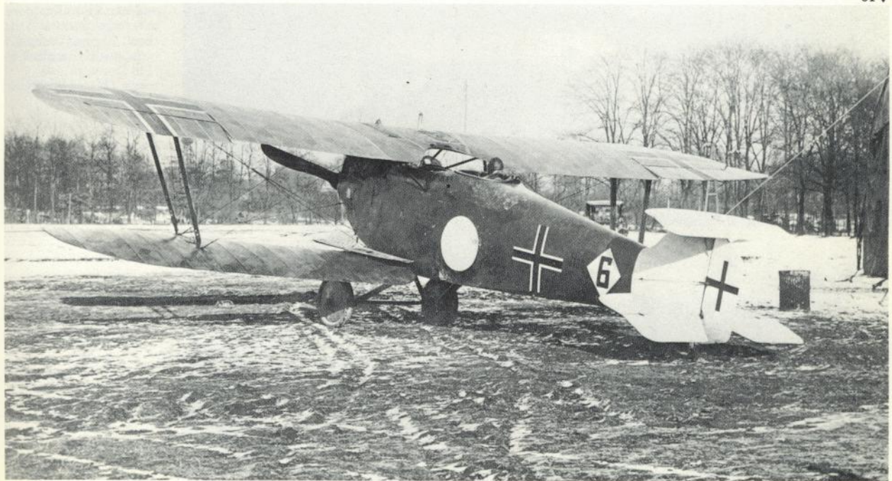
61. The Hannover CLIII, unusually for a single-engined machine, featured a biplane tail unit, which did, however, give the observer/gunner a wider arc of fire. The type became operational towards the end of 1917 and was a formidable opponent for Allied fighter pilots. Over 1,000 Hannover two-seaters were eventually built; postwar, a few saw Dutch service. (Harry Woodman Collection)
