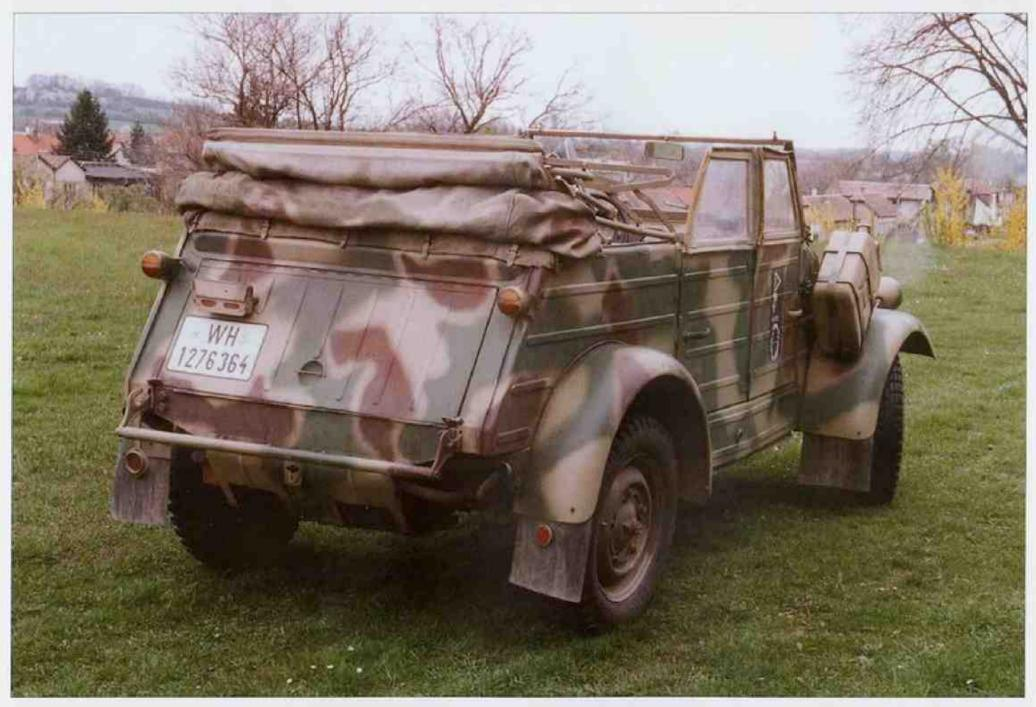
Front registration number plates were always painted on the nose of the body, despite the body colour and production year, see left bottom picture on the opposite page. In the early years of the war the rear registration number was painted on the sheet metal plate fixed on the engine cover, see page 2 on the bottom. In March 1943, the engine cover was modified shortening two left mouldings and since that moment also the rear registration number plate was painted on the cover directly.
