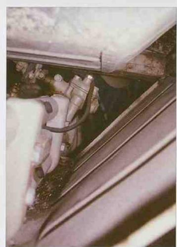
Steering worm and sector gearbox is installed directly on the axle transversal tube and is the same like on the KdF 166 Schwimmwagen. Note the trailing arms, radius rod connected to steering arm and bowden actuating brake.
