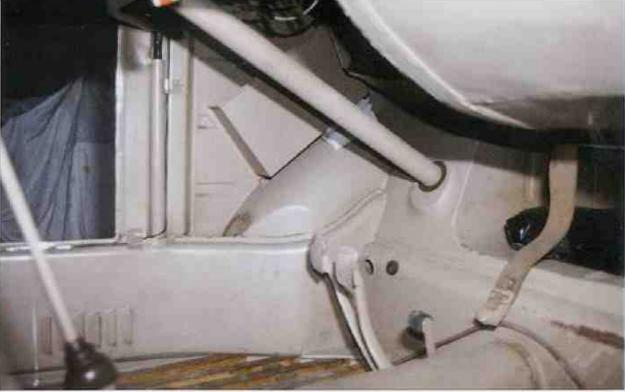
Air vents below door are a part of heating system and lead the warm air from the engine compartment to the cab. Heating has, however, very low efficiency and the warm air is hardly able to warm up the driveris boots. Note also the sheet metal box for storing documents located on the body side left to the steering column.
