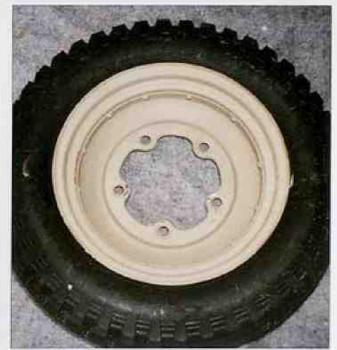
The spare wheel shown on the picture below is wearing a brand new tire which is a copy of the original one. Top right picture shows the inner side of wheel disc. These discs with riveted rims were made by manufacturers Kranprinz or Hering.
