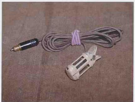
Clamp lamp with two bulbs, made by HELLA, picture above right, was a part of standard vehicular accessories. I could be connected by Bosch plug to the socket on the dashboard. The keyring with VVV logo is original.
