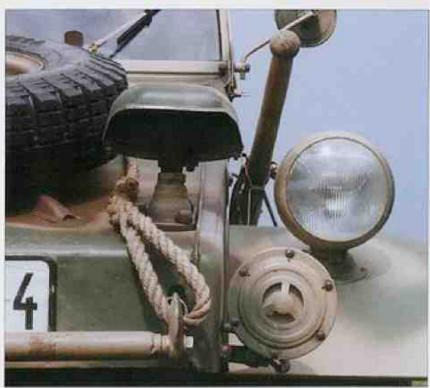
Spare wheel carrier shown here was used since March 1943, left bottom picture as well as the horn, shown on the right pictures. This horn has the front cover made of pressed sheet metal and the body made of brown bakelite while the early one was completely made of bakelite. Note also head lights made by Bosch. Electrical cable is connected to the rear part of the light body by means of screw connector.
