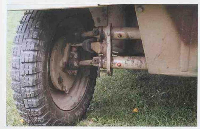
Because of rather low load on the front axle the front shock absorbers are rather small and only 140 mm long, bottom left picture. The front end could be easily hoisted manually when necessary.
