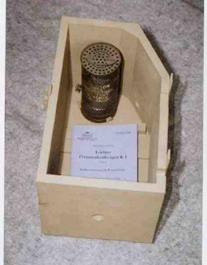
Pictures on this page show parts of battery winterising kit. Battery was located in wooden box. This box was connected with warm air duct by a piece of tube (see rounded opening on the bottom left picture) which heated the battery when the engine was running. When the engine was stopped the battery was heated by gasoline burner shown on the left top picture. Note also the original lettering on the box lid and operation manual.
