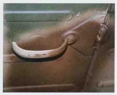
Detail shown above is the opening for Picture above shows the cab door hin- Detail of external door handle is shown on the picture above. The handles themselves were the same like internal ones.
