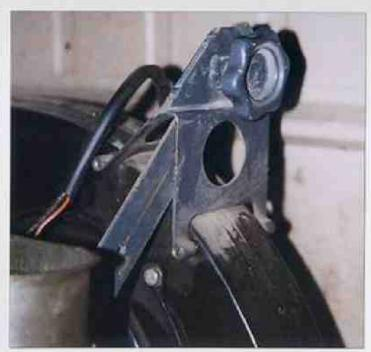
Dry centrifugal air filter shown on pictures above was typical feature of KdF equipped for desert use, as well as a small can on intake manifold knee. This can contained engine fuel and helped to enrich to mixture of air and fuel in the hot weather. The can was filled using the dropper shown on the previous page.
