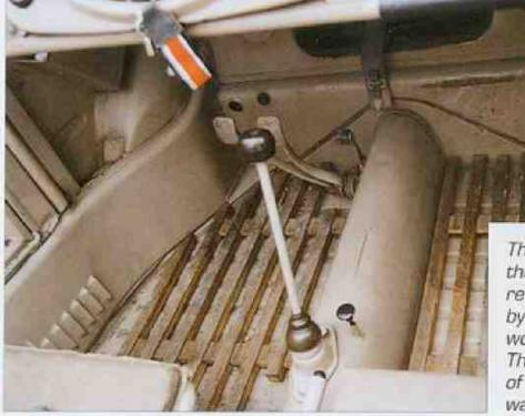
The first aid kit locker is above the steering wheel column, picture above. Cab floor is reinforced by grid made of integral beech wood laths, picture below.
