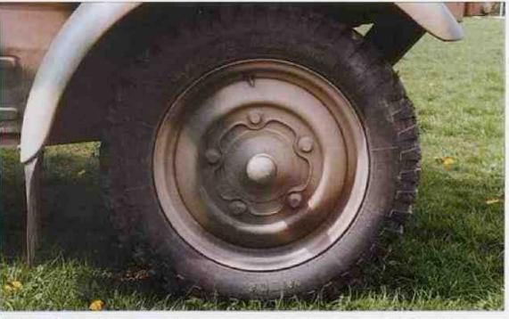
All these wheels are wearing very accurate copies of original tires. This tire pattern appeared in the second half of the war. The spare wheel shown on the central picture has the wheel cap which was typical for the first KdF production series.
