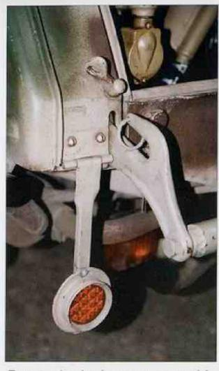
rod forming rear bumper, picture above. Note also hinged reflector.
