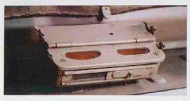
So called Notek lights, typical feature for most German vehicles having been used during the war, were used in black out conditions. Intensity of the front light could be adjusted using rheostat on the dashboard. The rear light consisted of two group of lights.
