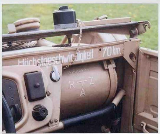
Windshield vipers engines are connected to electrical system by means of cables allowing to fold the windscreen, see also page 15.
