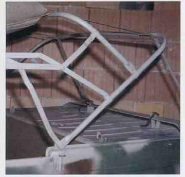
Pictures on this page show the baggage compartment behind the rear seats. Removable cover on the bottom of baggage compartment enables removing of the engine starter, the oblique cover in the rear wall is used for better access to coil. These cover were not installed on vehicles made before March 1943.
