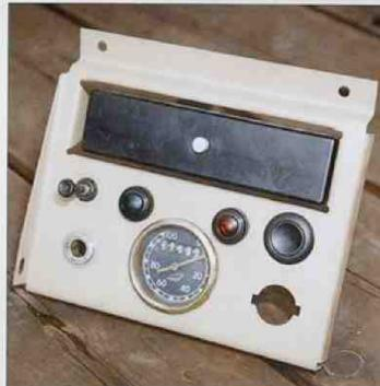
Compare the original oval dashboard, picture above, used on the first series of Kübelwagen with the newer one, installed during the second half of the war, picture on the top. The newer square dashboard is identical with the one installed on KdF type 166 Schwimmwagen.
