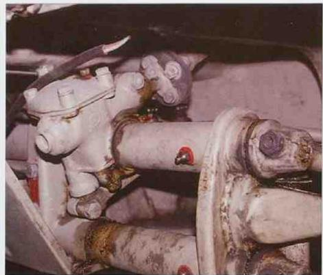
Top and bottom left pictures show frog view of the rear part of the body and engine. There are two exhaust silencers, one on each engine side. Left silencer tube is connected with injector sucking dust and sand from centrifugal filter installed on air intake.
