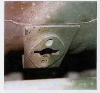
starting crank located on the rear ge, viewed from inside. part of engine compartment.
