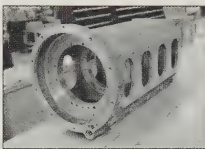
Above: A look into the rear of an Offy crankcase showed its barrel-type construction and the circular apertures to which the diaphragms carrying the main bearings were bolted. Oval side openings gave access to the engine's interior for the mechanic.
