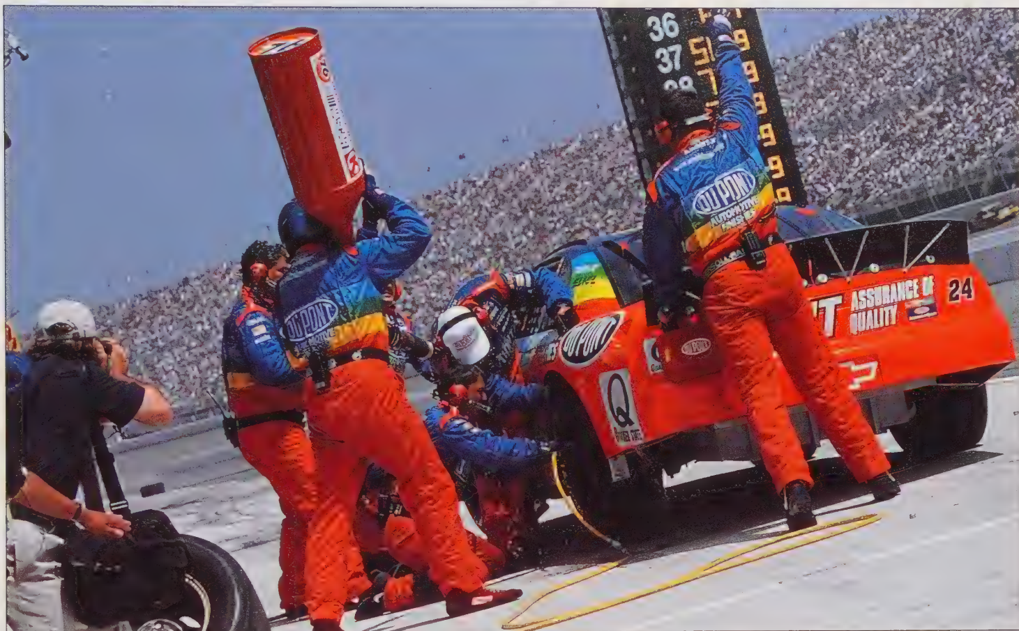
Jeff Gordon's Chevrolet Monte Carlo is helped on its winning way by the 'Rainbow Warriors' crew during a pit stop at Riverside, California in May 1999. The mechanic at the back of the car indicates the refuelling is complete, while the fresh wheels are torqued up.
