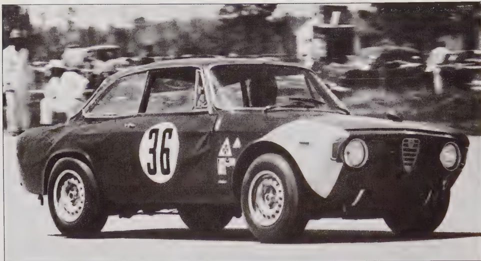
Bearing the scars of Bussinello's practice crash, Jochen Rindt's Alfa Romeo GTA was first overall and under 2.0-litre (122-cubic-inch) 'U2' class winner in the very first TransAm race at Sebring in 1966. The GTA was powered by a twin-plug head 1600 twin-cam engine.
