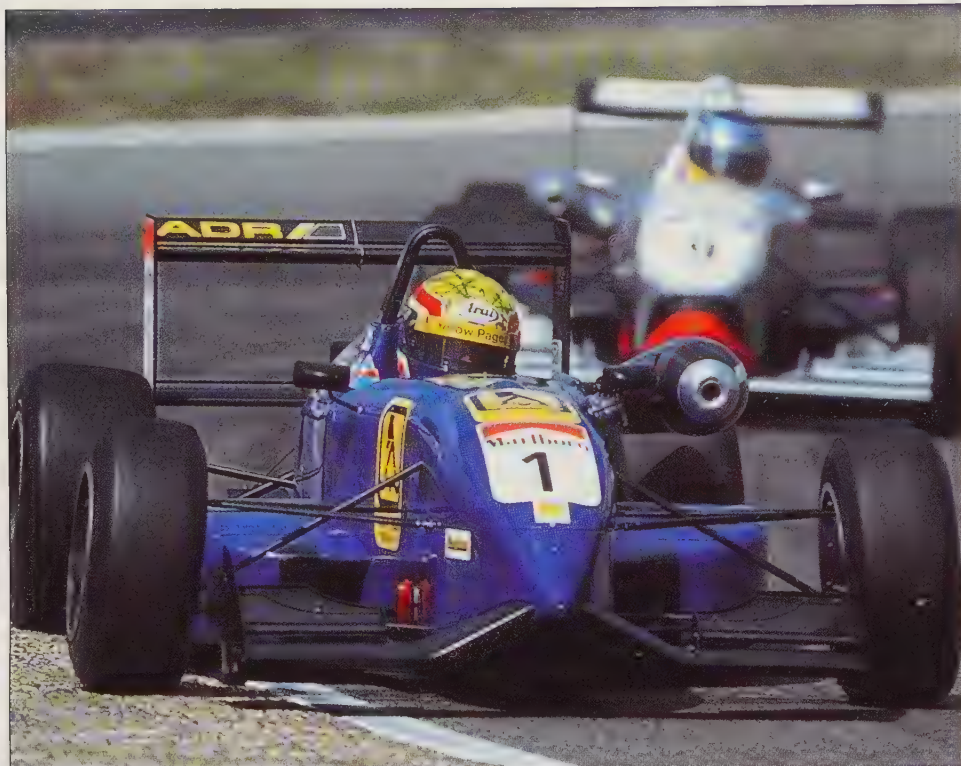
Mark Webber in the Alan Docking Racing Dallara gets two wheels off on his way to 3rd at Zandvoort in a round of the Marlboro Masters F3 series in 1997. Note the prominent air restrictor on the left of the engine cover.
