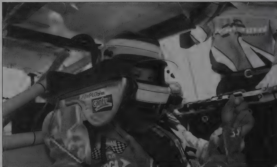
Milka Duno is shown here in her Venturini Motorsports race car. Duno, who captured the pole for the 2013 ARCA Racing Series International Motorsports Hall of Fame 250, is wearing her protective gear, including a HANS device, harness, and protective cage with padding. Her window net has not been secured at the time of the photograph. (Courtesy of Venturini Motorsports.)
