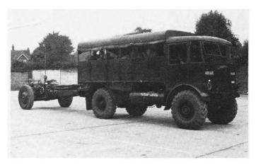
An early production AEC Matador (diesel) towing a 6 inch 26 cwt howitzer of 3rd RHA. Note lack of access door in body fitted to later vehicles.
