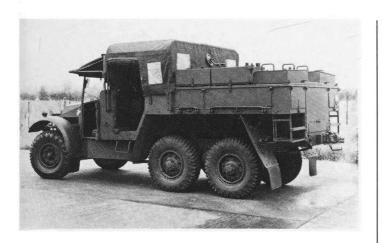
Early production version of the CD/SW LAA tractor with standard body. The enclosed prototype body having been completely redesigned to give a lower silhouette.
