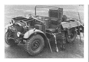
The Royal Engineers used air-compressor versions of the 15 cwt for a variety of tasks. This pre-war Morris CS8 is fitted with an Air Pumps Ltd compressor to power a variety of pneumatic tools including shovels, drills and hammers.
