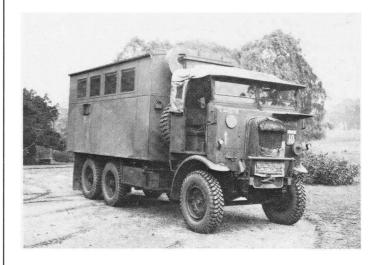
The sound-ranging and plotter body was used in conjunction with sound-locating equipment to determine the position of enemy guns. A comparatively rare vehicle. The Retriever now sports a windscreen as a sop to driver comfort.
