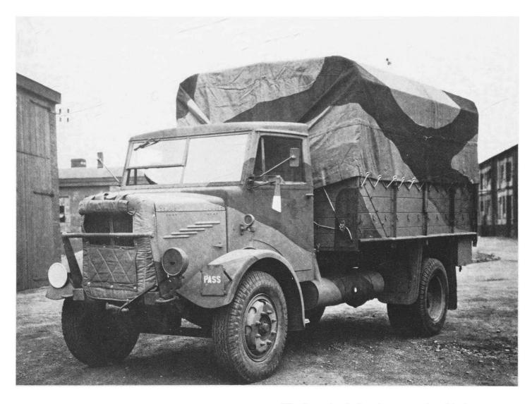
termites etc. Planners looking ahead to the Far East required steel bodies for jungle warfare as water absorption of wooden bodies eventually led to rot setting in.
