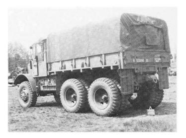
The Mack No. 27 $\frac{1}{2}$  ton 6 × 6 artillery tractor. Designed to tow heavy artillery such as the 155 mm gun and 8 inch howitzer. This particular vehicle has the special trail clamp fitted to which trails of certain guns were attached.
