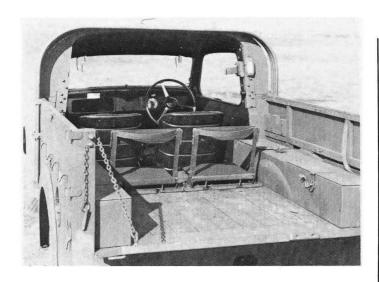
This interior view of an Austin 10 hp G/YG light utility shows the folding rear seats, tilt hoops stowed and various stowage lockers.
