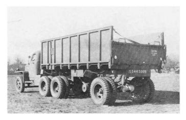
The American equivalent of the Bedford was the Studebaker  $6 \times 4-2$  4/5 ton cargo truck supplied under lend-lease to the British Army, and to the RAF with different pattern of semi-trailer.
