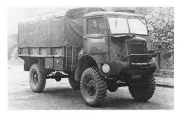
The  $4 \times 4$  load carrier was intended to replace the  $4 \times 2$  in production but this was never achieved. The Bedford QL was perhaps the best known British  $4 \times 4$  3 tonner. Shown here fitted with a US-style steel cargo body.
