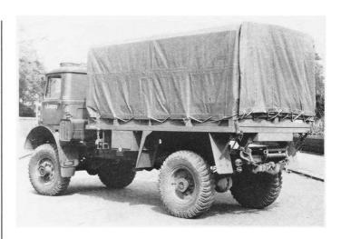
The Bedford QLW tipper was an airportable vehicle but had to be completely stripped down for airlifting in two Douglas C47 Dakota aircraft.
