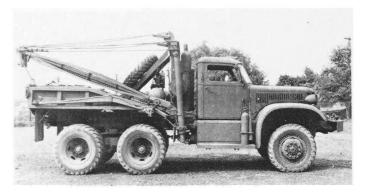
The Diamond 'T' Model 969 4 ton  $6 \times 6$ , with Holmes twin boom lifting gear, saw widespread service post-war with civilian garages.
