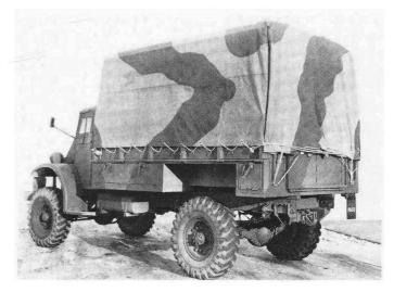
The Ford F30L was typical of the early CMP 30 cwt body type 3A1 and was discontinued in favour of the 3 ton class. The 3 ton version was similar in appearance but with heavier springs and larger tyres.
