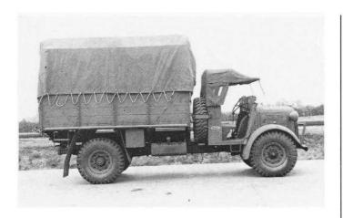
The other type of light lorry in British service was the  $4 \times 2$  30 cwt typified by the Austin K30. Large numbers were lost in 1940 and production tapered off in favour of the 3 ton class.
