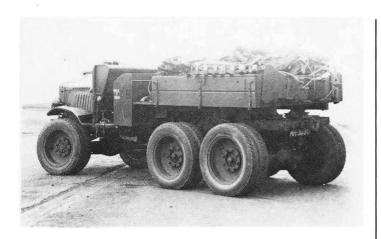
The experimental  $6 \times 6$  artillery tractor produced by the RASC from standard Hathi components and fitted with a WD-pattern rear bogie was probably Britain's first  $6 \times 6$  military vehicle. Census no. T 17542, registration no. MH 3090.
