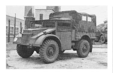
The 6 pdr A/Tk gun tractor version of the Guy Quad-Ant  $4 \times 4$  15 cwt can be distinguished by the winch rope guide rollers on the front bumper and the translucent 'windows' in the tilt.
