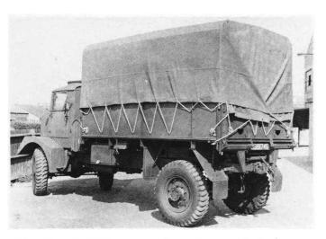
The Karrier K6 was another airportable 3 ton vehicle, but only if stripped down. The winch version was a much sought after vehicle within British units and saw useful post-war service.
