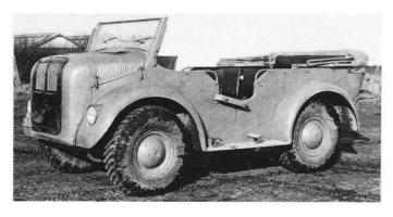
Top Another Czech product to undergo testing was a late example of the Tatra  $T82.6 \times 4$  command car fitted with a flat-four 2,500 cc aircooled engine.
