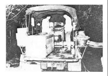
An American Army mobile kitchen on a  $1\frac{1}{2}$  ton  $4 \times 4$  – the troop seats have been folded outboard to provide extra working tops.
