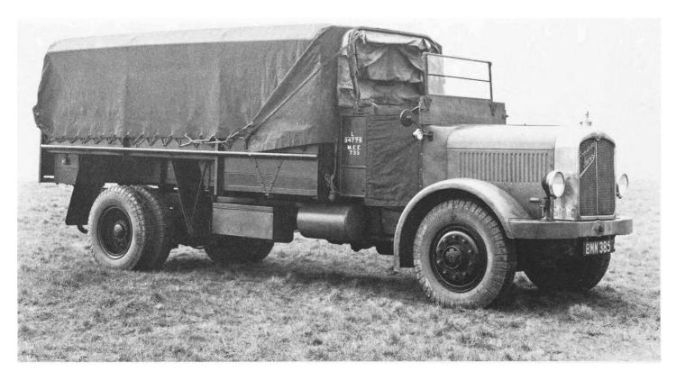
discovered that the specialist bodies designed to be mounted on the  $6\times 4$  could not be accommodated on the shorter  $4\times 4$  chassis without major re-design. Also the demand for  $4\times 4$  load carriers was so great at the time that none could be spared to replace the  $6\times 4s$ , and this type continued in production until the end of the war.
