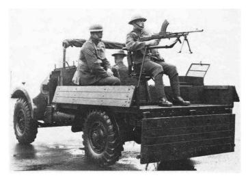
An early production Morris 15 cwt with standard body showing the sides dropped for use with the special Bren gun mounting which gave a good field of fire but left the gunner rather exposed.
