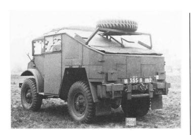
Typical CMP field artillery tractor. This is a Ford FGT fitted with the fourth type of body, carrying a spare wheel on the rear sloping deck indicating that run-flat types were not fitted.
