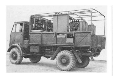
Thornycroft produced about 5,000 Nubian TF/AC4 chassis from 1940 to 1945 and the basic design is still evident in current fire tenders. Illustrated is an RAF tender, type 348, for generating electrical power. It proved popular with showmen in the immediate post-war era.
