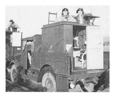
A Bedford MW 15 cwt fitted with an AFV crewtraining box in post-war service. These cabins were used to initiate trainees in the mysteries of R/T procedures before they were let loose on real AFVs.
