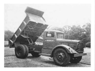
The American Brockway 10 ton  $4 \times 2$  tipper saw service with the British Army in relatively small numbers.
