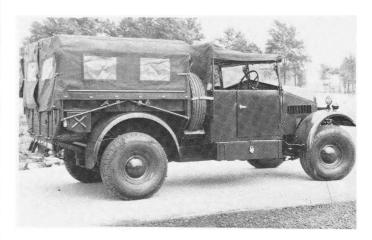
The personnel/utility 8 cwt was produced in the early war years and the Morris Commercial  $PU/Mk\ 2\ 4\times 2$  was a typical example. The tilt could be removed and used as a tent, folding ground spikes providing supports.
