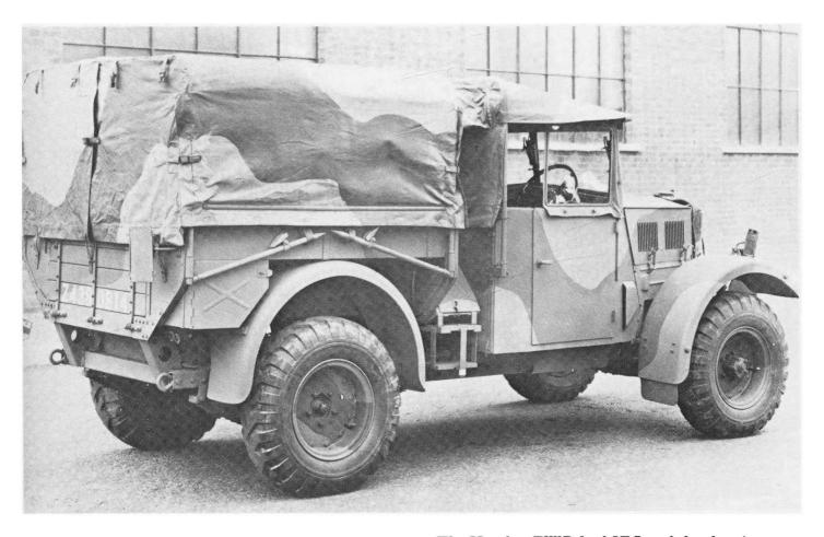
The Humber FWD had IFS and the chassis carried heavy utility (Humber box) light ambulance and light recce car bodies as well as the PU body illustrated.
