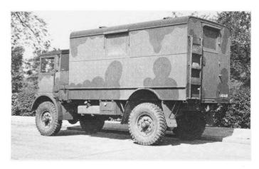
The Austin K5 shown here is fitted with a Westex Recorder body used by heavy A|A regiments in conjunction with locating radar.
