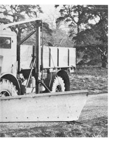
This example of an FWD – SU-COE fitted with a British medium artillery tractor body has been extensively modified to take snow-plough equipment.
