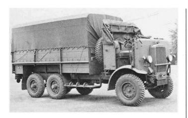
The Leyland Retriever  $6 \times 4$  3 ton chassis was fitted with a wide variety of different bodies – here is an early production 3 ton GS lorry.
