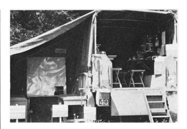
A Divisional HQ signals lorry set up for field operations. A sign reads 'public telephone' and the vehicle is an early CMP 3 ton GS.
