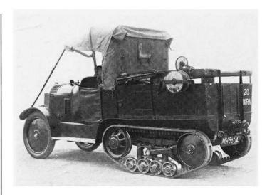
In the 1920s the British Army experimented with various types of semi-tracked vehicles, the 9th Regt Field Artillery being equipped with a selection for trials. The Citroen-Kegresse P7 battery car being one type.
