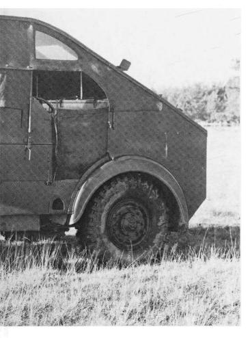
Morris 'Quad' now with hard top and sloping rear to accommodate the 25-pdr traversing wheel, the holding-down attachments can just be seen.
