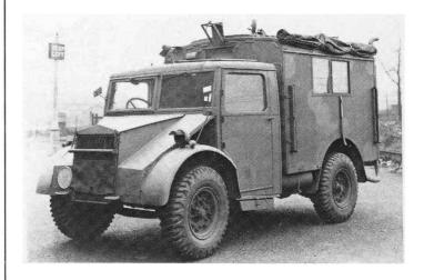
A late production Guy Ant with enclosed 'Vixant' type cab and light warning body – a radar vehicle used with AA Regts.
