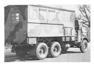
The machinery (house type) body could be fitted out to fulfil several mobile workshop roles. The generator supplying power for the machinery is located forward of the rear bogie. The vehicle is an Albion BY3.
