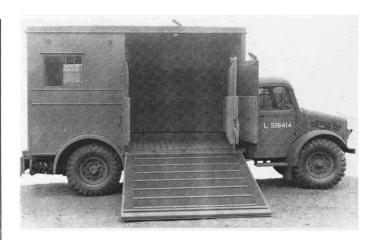
Small numbers of horse ambulances were required despite complete mechanisation of operational units, and bodies of pre-war design were fitted on Bedford OY chassis.
