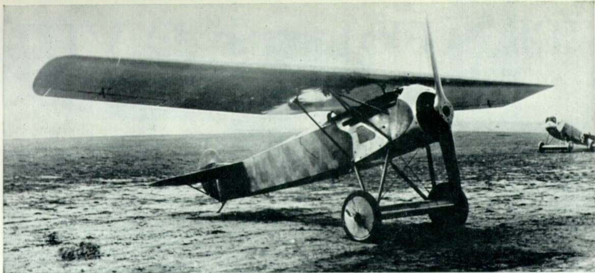
Third of the Fokker parasol monoplanes that participated in the first German fighter trials, the V.27 had a 195-h.p. Benz Bz.IIIb engine. (Photo: via R. Ward)
