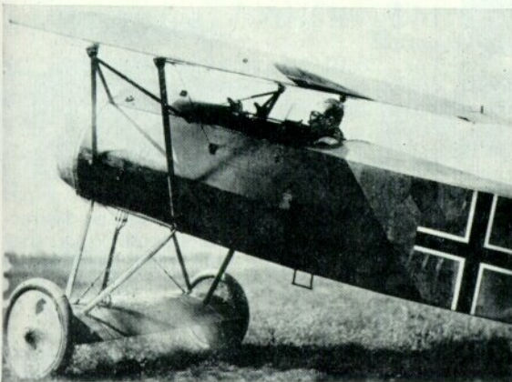
Fok. EV, 238/18, with the main fuel tank in the undercarriage aerofoil. In the cockpit is Ernst Udet. (Photo: Peter M. Bowers)
