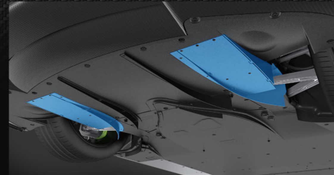
Diffusers in the underfloor
