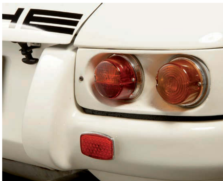
Lights were by Hella and installed in lightweight glassfibre housings. Rear bumper was glassfibre, too. Louvred rear quarter windows aided ventilation
