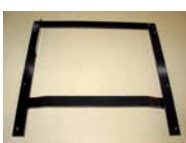
Part of the month T6 'B' and 'C' Seat sub-frame for Speedster seats. PRS Product to convert Speedster seats to fit into your 356 'B' T6 or 356 'C' £115.00 +P&P
