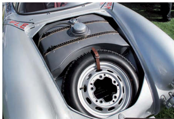
Above: Everybody wanted their photograph taken with 550-03... Spyder was dwarfed by contemporary American automobiles. Right: second spare wheel was stored away, along with the long-range fuel tank, under the removable front panel. Hardtop may not have been used in the original event, but it sure looks good!
