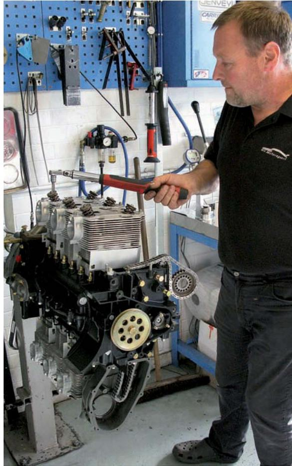
Neil Bainbridge buttons up the top-end of Mike Moore's motor. RSR-spec air deflectors were used between cylinders - they're aluminium rather than steel
