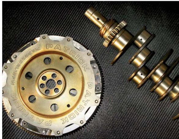
Mike managed to locate a standard/standard crank which is shown just back from polishing and balancing with the Patrick Motorsports RSR flywheel, ring gear and a Sachs power clutch. It's coated here with a tectyl protective wax, which has given it the golden colour
