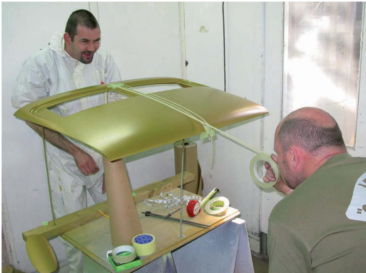
engine grille – the distance between the bars that hold the individual slats of the grille together gave us the reference points we needed. But it still took an age just to mask up the engine lid! However, once we'd set the width, it was relatively easy to transfer the dimensions to the bonnet/hood.
