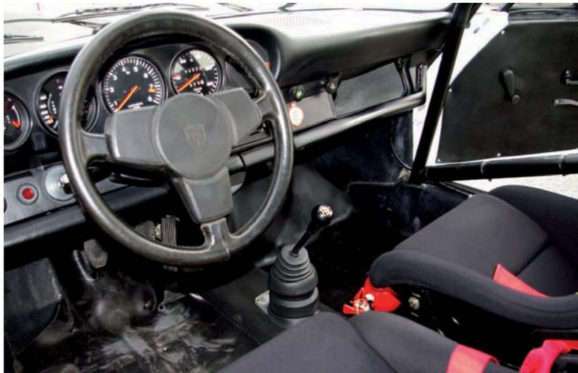
*Recaro seats have been upgraded to meet current FIA regulations. Full-on RSR version came with 10,000rpm tach, but road-going RS featured regular 8000rpm instrument*
