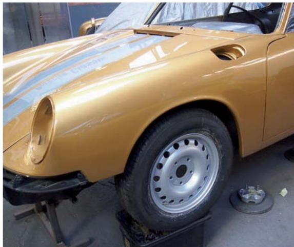
We chose Vredestein tyres in 195/65 section to use with the 15in space-saver wheels. These have been powder-coated in dull silver to replicate aluminium colour. Couldn't resist offering one up to the car to see what it looked like
