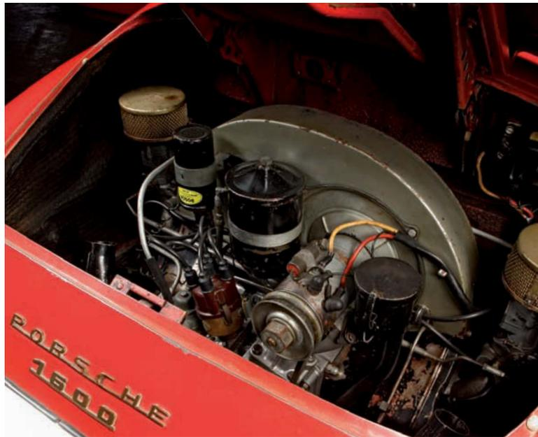
*356 Speedster's interior is basic, to say the least, with few home comforts. Trusty dual-carb 1600cc pushrod 'four' develops 75bhp in 'Super' specification*
