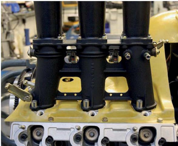
Far left: Shroud and the other 14 pieces of 'tinware' were specially made for the engine. MFI stacks were mounted using correct barrel nuts
