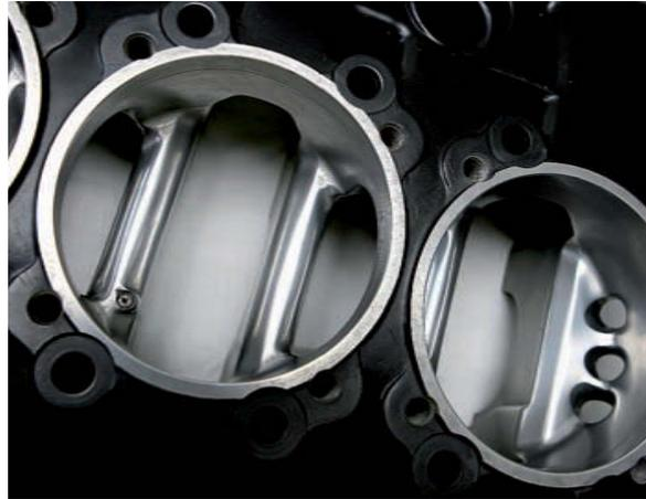
The 2.8 RSR ran as a 3.0-litre late in '73, and now due to the fragility of the 7R case the FIA has homologated the 930 Turbo cases for the car, which is what Mike opted to use. They were gas-flowed and finished by hand, and then treated with a protective no-friction coating used in the Formula 1 industry that's only 20 microns thick
