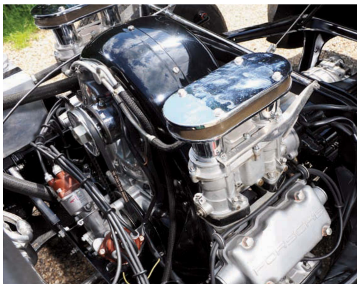
The two-litre version of the four-cam 'Fuhrmann four' sits immediately behind the driver. The Type 587/3 unit was developed by Hans Mezger to give 185bhp
