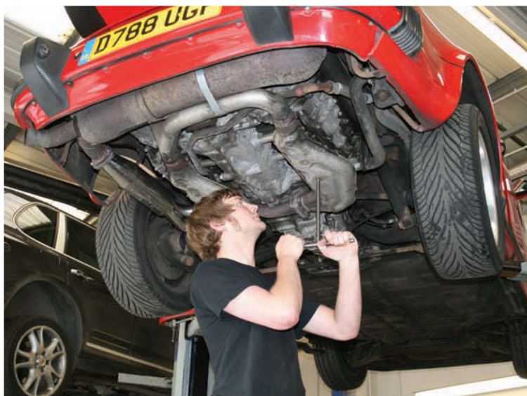
Exhaust re-fitting at PCT after pre-silencer failed
