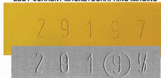
"VIN-PRINT" OF ALLOY USING EDDY-CURRENT MAGNETOGRAPHING IMAGING
