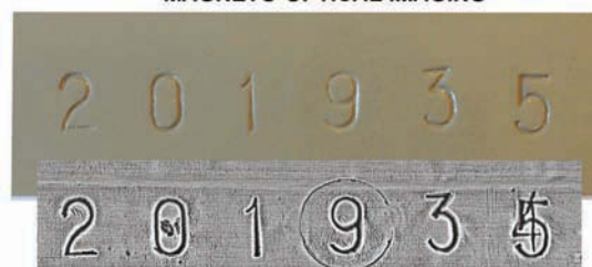
"VIN-PRINT" OF STEEL USING MAGNETO-OPTICAL IMAGING
