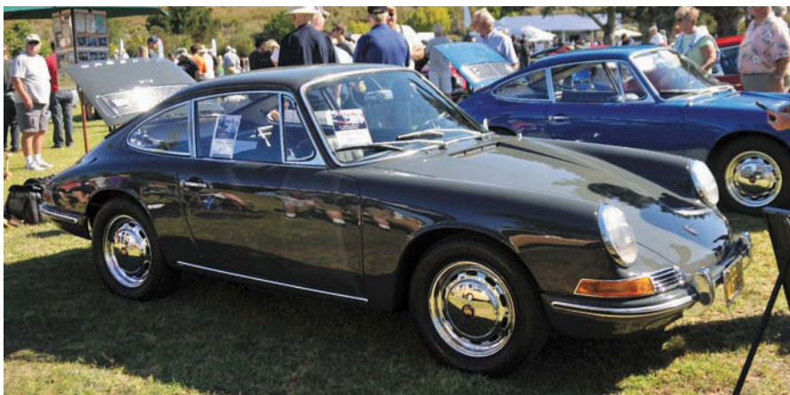
David Derr owns this 1969 912-based RS-clone conversion. Under the deck lid is a 3.2-litre motor and a 915 transmission, amongst other upgrades
