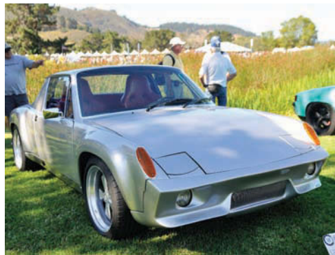
This 1971 914 was converted to an all-steel 916 clone. Under its silver metallic paint is a full roll cage, a 964 3.8-litre RS-spec 315bhp engine sending power through a 1985 915 five-speed, 964 four-piston brakes, air conditioning and full leather interior. It's built and owned by Patrick Motorsports
