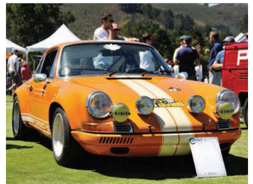
Originally a 1971 Signal Orange 911T, it was custom built to emulate a 911ST factory race car. Some features incorporated are 'ST' style seats, aluminium roll bar, a balsa wood-reinforced glassfibre hood, aluminium engine lid, centre-fill gas tank, external oil cap and Cibie Rallye lights. It was built by TRE Motor Sports and is owned by Robert Abbott
