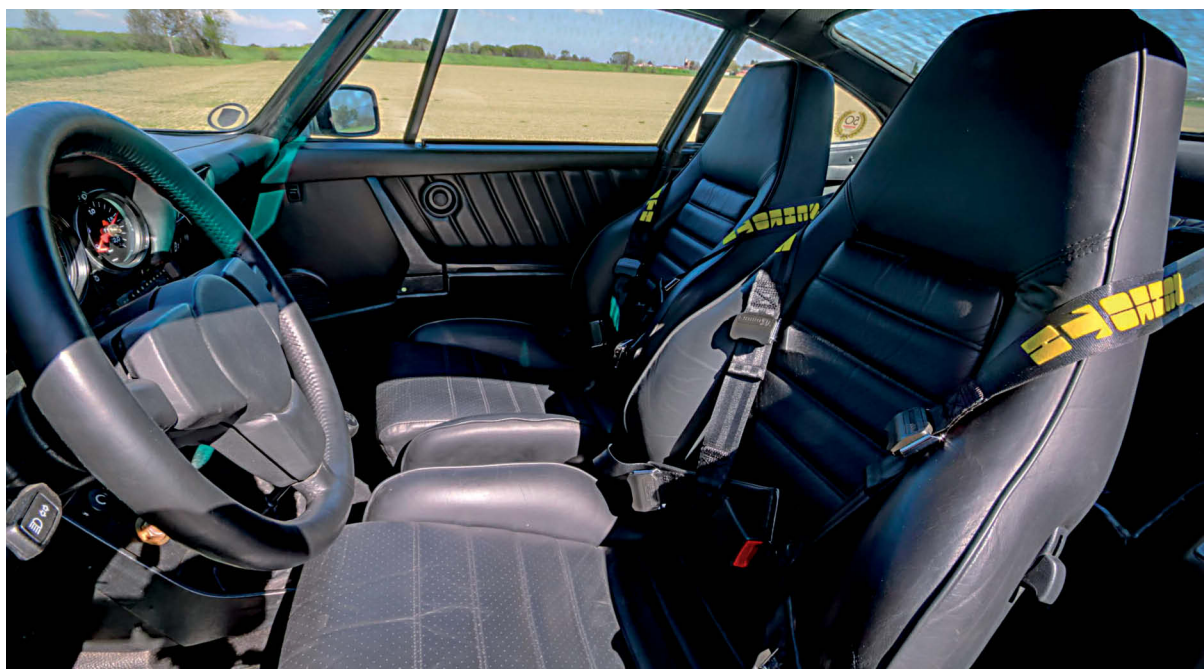
Thicker RUF steering wheel and retrimmed sports seats are complemented by the Schroth full harnesses. No rear seats are fitted due to harness mounting points
