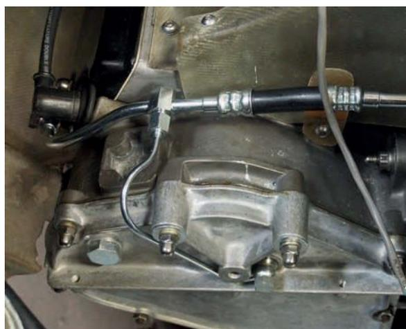
*The longer oil line required for installation on earlier engines fits to the right side – this negates the need to install a later adaptor piece. You'll need to trim the engine tray to clear the oil feed line on the right side, too*
