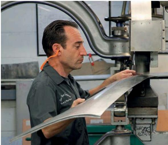
*Planishing hammer and English wheel allow the skilled workforce to recreate virtually any shape of body panel in steel or aluminium*
