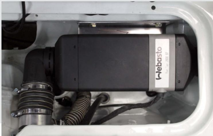
D-P Motorsport has introduced what it refers to as an intuitive controllable heating system for all left-hand-drive Porsche 911s up to 1989 (ie, pre-964 models) which don't have factory air-conditioning fitted.
