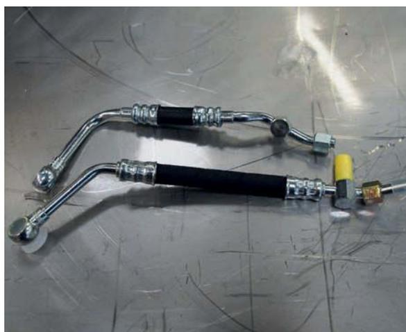
The complete pressure-fed tensioner upgrade kit – you'll need the longer extra oil line if fitting to early engine. Cam chain covers are aluminium, rather than the magnesium used on early engines
