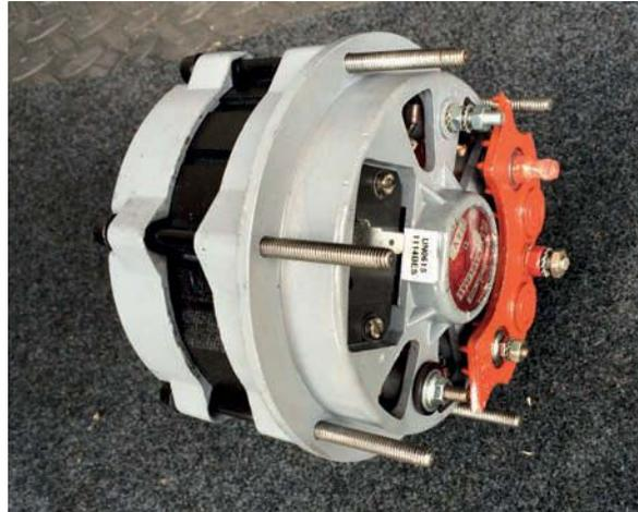
Changing the alternator on a 911 is a fiddly process but it had to be done as the diodes had failed in the original unit. Rebuilt one came via Canford Classics
