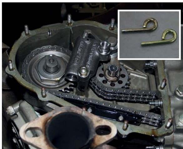
930 cam-chain tensioner is on the left, later Carrera pressure-fed type on the right – the latter is shown fitted in the photo on the right. Don't forget to remove these two retaining pins!
