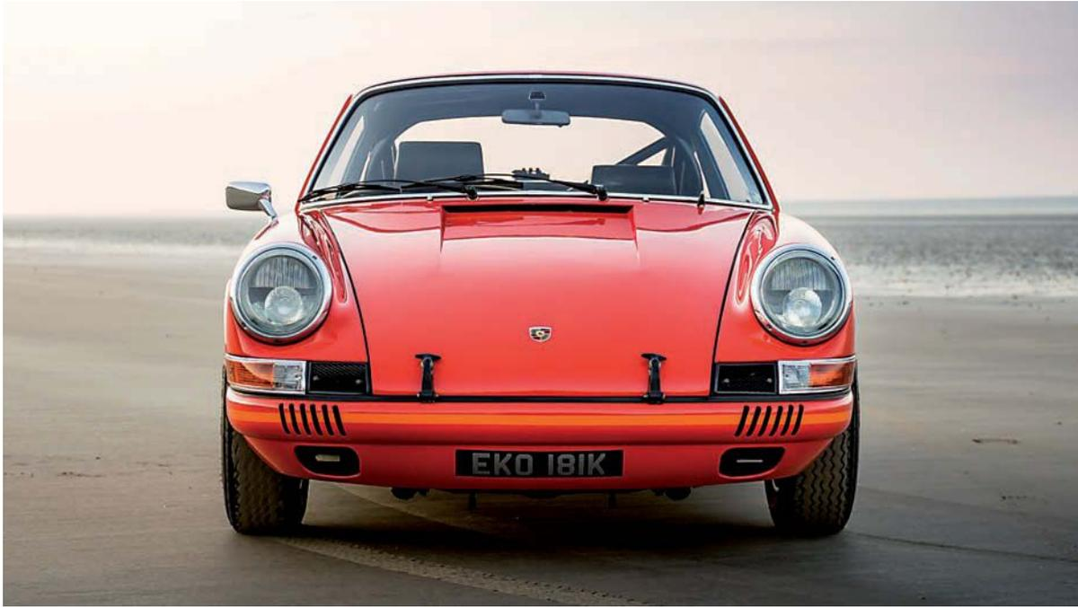
Slots cut into the front bumper are a Darren 'signature touch', allowing air through to the front-mounted oil coolers. Panel fit is exemplary throughout...
