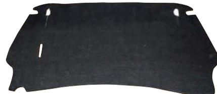
1965 to 1970 Engine sound pad. Tear out that moldy rats nest hanging from your firewall! Correctly dimpled and fire resistant just like OEM.
