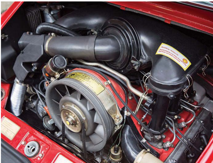
2.7-litre mechanically-injected Carrera engine is the same as that used in the 1973 Carrera RS. Front seats are optional leather, but the remainder of the interior is trimmed in vinyl
