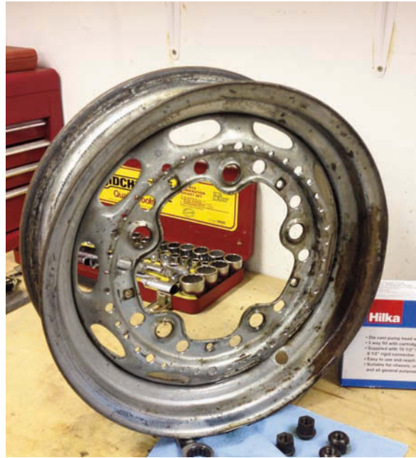
Far left: Drilling the aluminium brake drums was a trick the factory used to reduce unsprung weight – and to aid cooling
