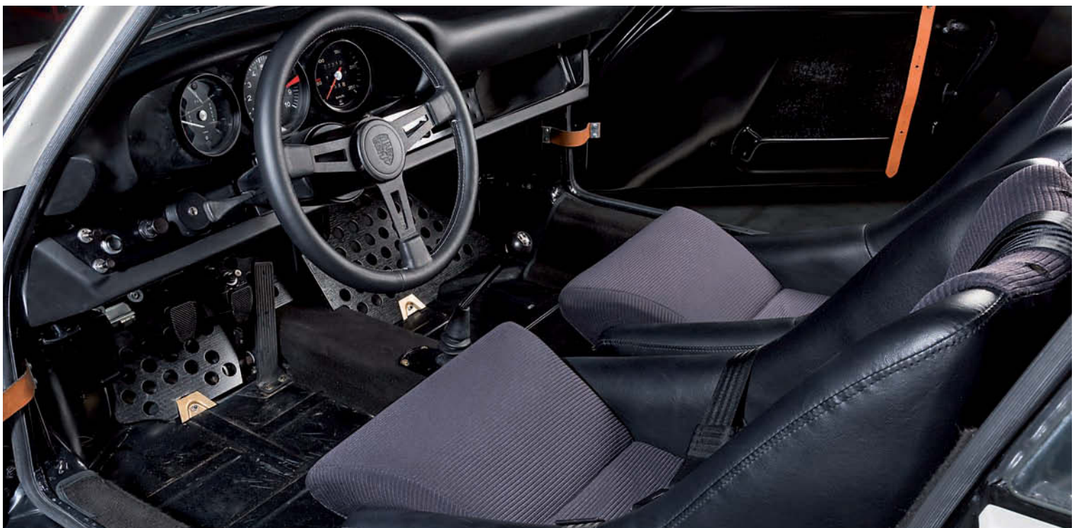
Below: No-frills dashboard means no glove-box lid, no radio and just three gauges. Fuel and oil level gauges are dispensed with, along with the clock
