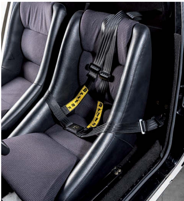
Above left: Scheel seats are used in conjunction with four-point Britax harnesses – you'd never get away with that today, when thicker webbing and five-point are the order of the day
