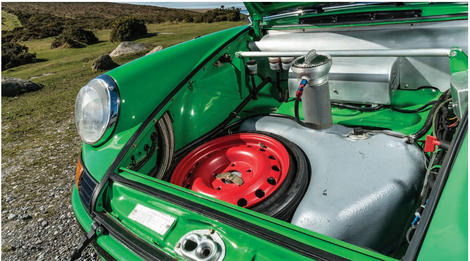
Above: Under the front lid you'll find a through the hood filler conversion, strut brace and that neat aluminium wiring cover. Note oil lines on left, serving the front-mounted cooler
