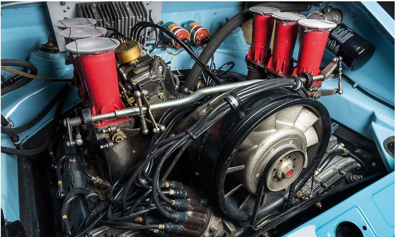
*Above: Dual-plug 2492cc engine is fed by Bosch MFI, and produces around 270bhp at 8000rpm and 191lb ft of torque at 6300rpm*
