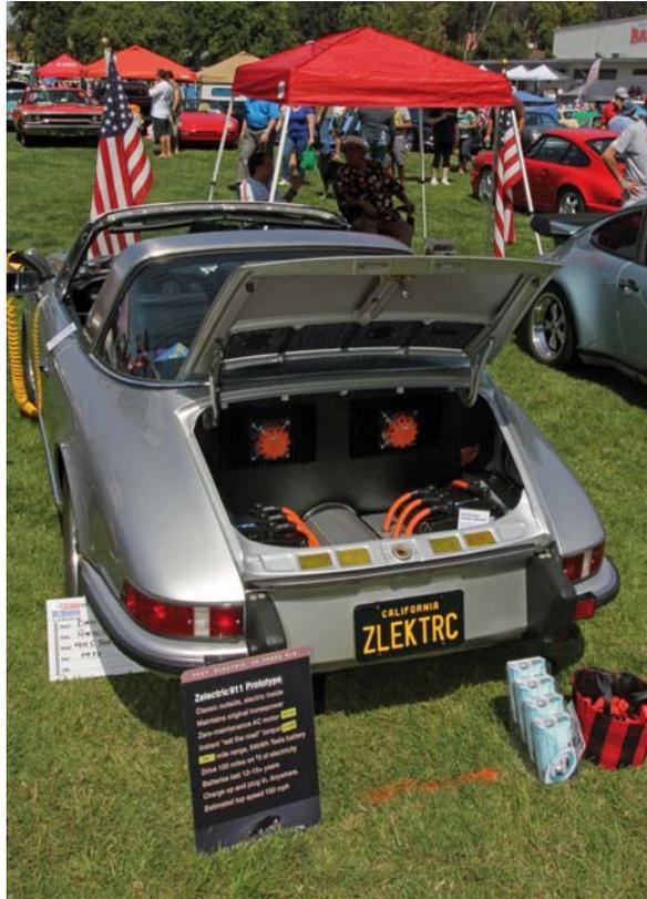
Right: Zelectric's '73 Targa prototype runs a 180hp AC motor and Tesla batteries offering 180 miles range
