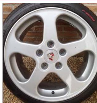
**Genuine Ruf wheel set for Porsche 993**, (complete set of 4) including tyres Pirelli P Zero. Front: wheels 8.5 J x 18 H2 ET58, tyres 225/40 ZR 18 N4 DOT 0910; rear: wheels 10 J x 18 H2 ET66, tyres 285/30 ZR 18 N4 DOT 3607. Wheels are in perfect condition, no damage at all, tyres are perfect with 7mm profile, centre caps not included, fits C2, C4, Targa, S, 4S, RS, Turbo, £2400/€2750. Tel: 32 475 723939. Email: guysteen68@gmail.com (Belgium). C46/019
