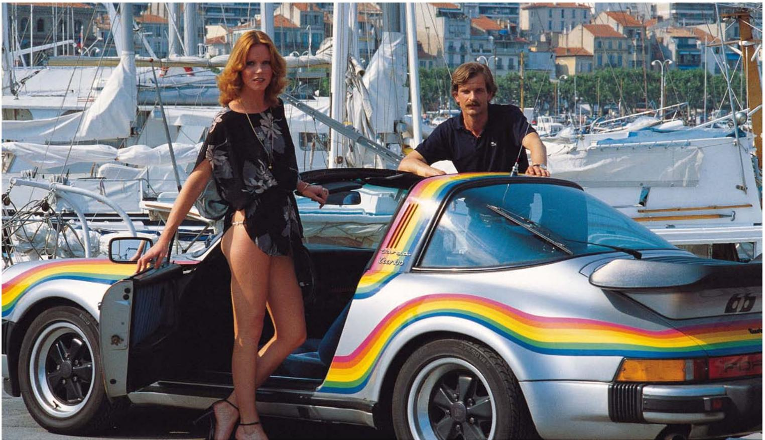
It was based on a 1979 911SC Targa, into which Buchmann installed the drivetrain of a 930 Turbo, adding the widened wings to match, creating a unique Turbo Targa several years ahead of Porsche, who would go on to build fewer than 300 Turbo Targas between 1987 and 1989.
