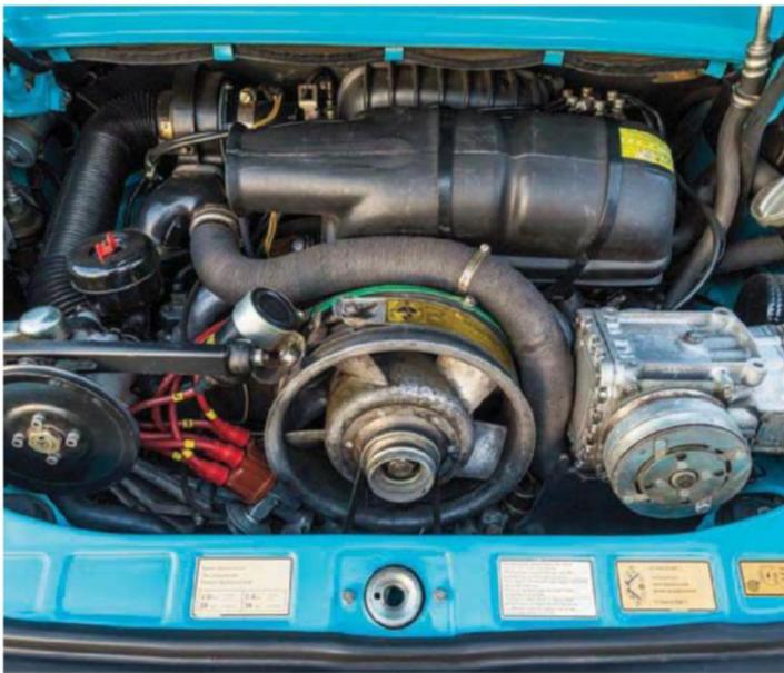
*Above left: Rebuilt 2.7-litre engine produces 180bhp and is less peaky in its power delivery, making the last of the 911Ss the easiest of all to drive*
