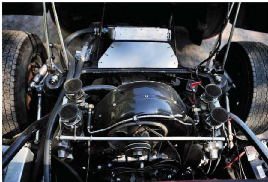
*Below: Clamshell rear bodywork gives excellent access to the engine. There's plenty of space to fit a six-cylinder engine – or one of the F1-spec flat-eights if desired*
