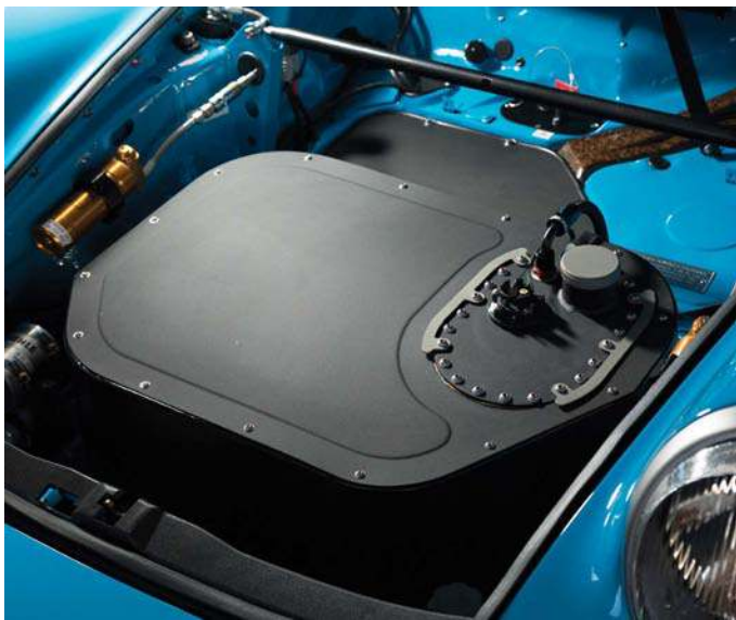
Above left: Fuel cell replaces the stock fuel tank, leaving little room for luggage!
