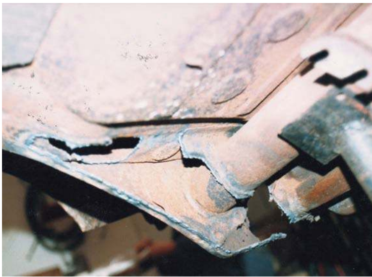
Above left: Rear torsion bar area had suffered from corrosion and required considerable repair work
