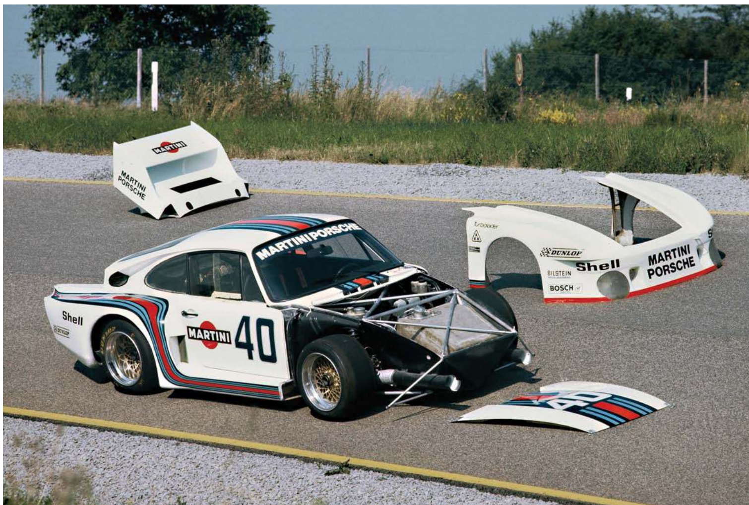
Above: The 935 Baby laid bare. The bodywork in front and behind the cockpit area was cut away to make way for ultra-lightweight aluminium tube subframes
