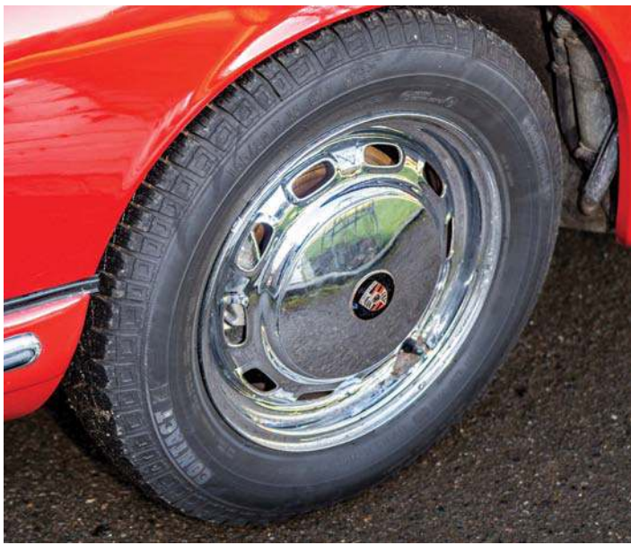
Above left: Steel wheels with flat crested hubcaps conceal the four-wheel disc brakes. Note electric aerial tucked away in the wheel arch
