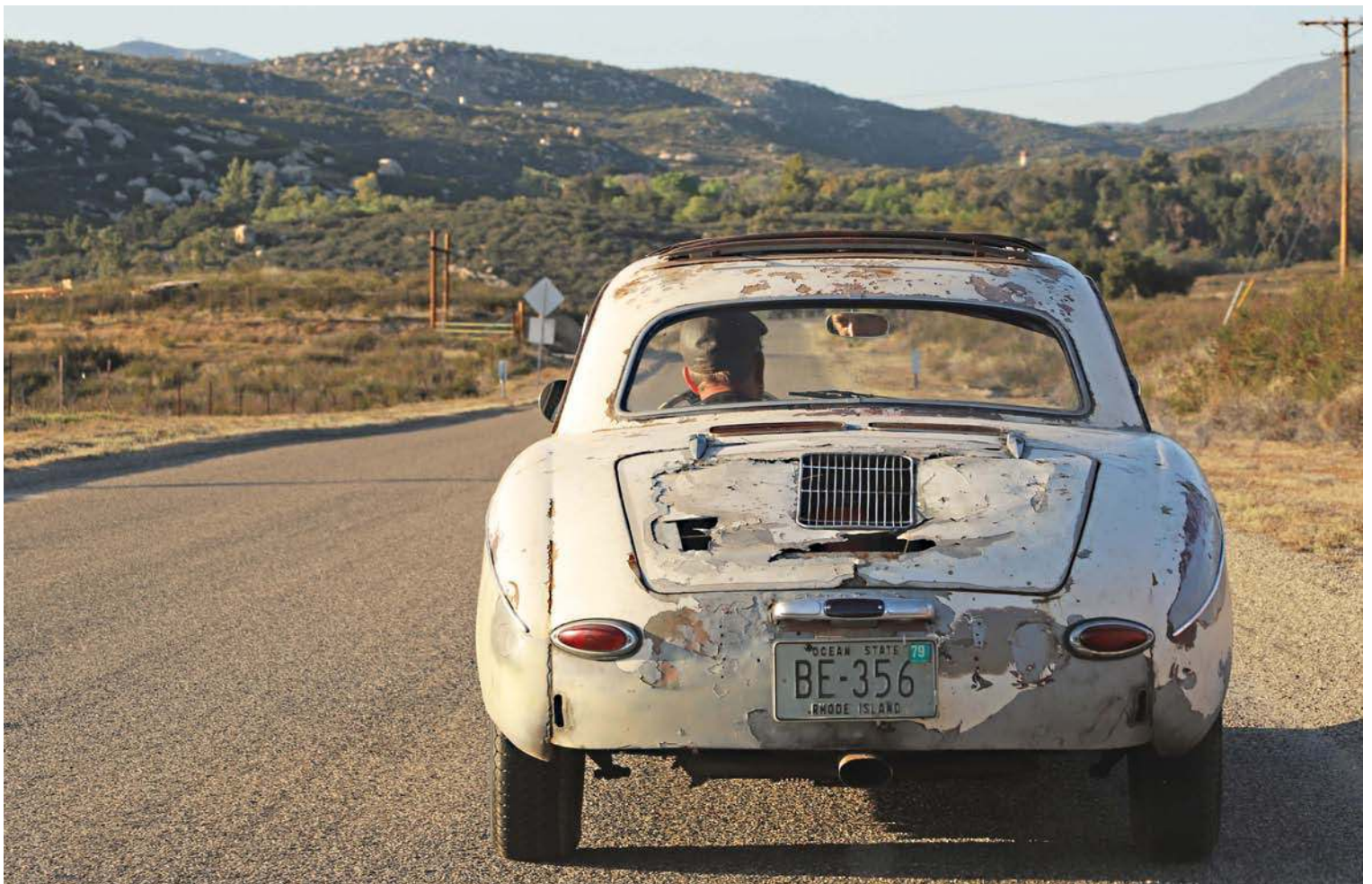
Below: Porsche 356 engine grille allows cooling air into the engine bay, supplemented by a two smaller grilles from the dashboards of a pair of Oval-window Beetles
