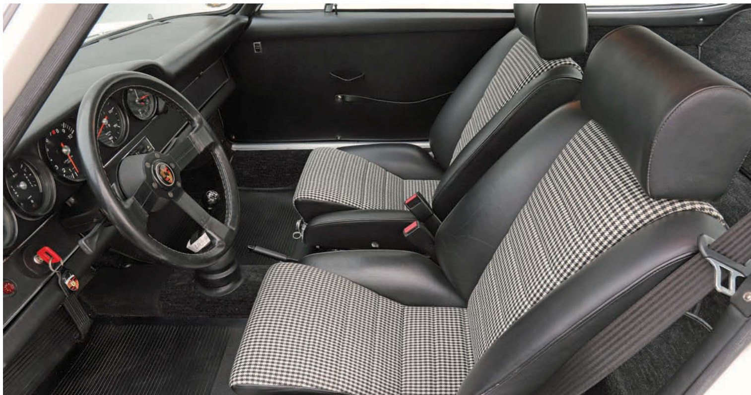
Below: With correct houndstooth material from Eric Linden, the factory sports seats in Dave's 911 were retrimmed by Tony Garcia at Autobahn Interiors
