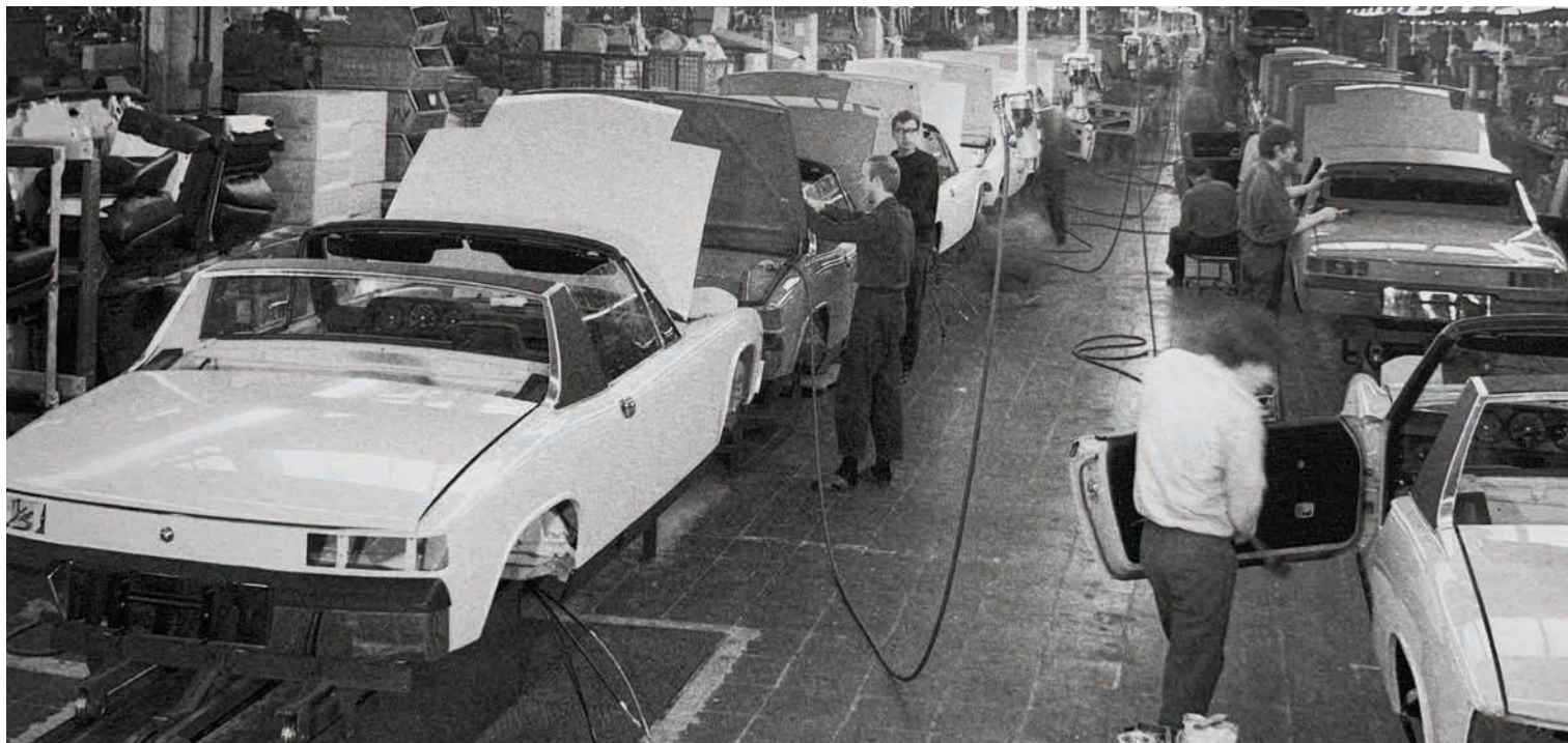
Below: The 914 bodysheells were built by Karmann, who went on to carry out final assembly of all four-cylinder models. The Porsche-powered 914/6 was assembled at Zuffenhausen alongside the 911
