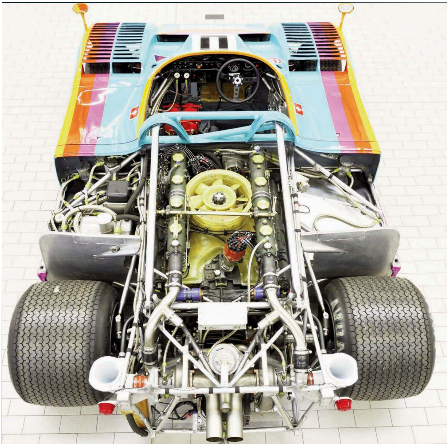
Above: As revised for the 1973 season the 917/30 chassis had a 7.2in-longer wheelbase of 98.4ins, a front track almost two inches wider and rear track nearly three inches narrower
