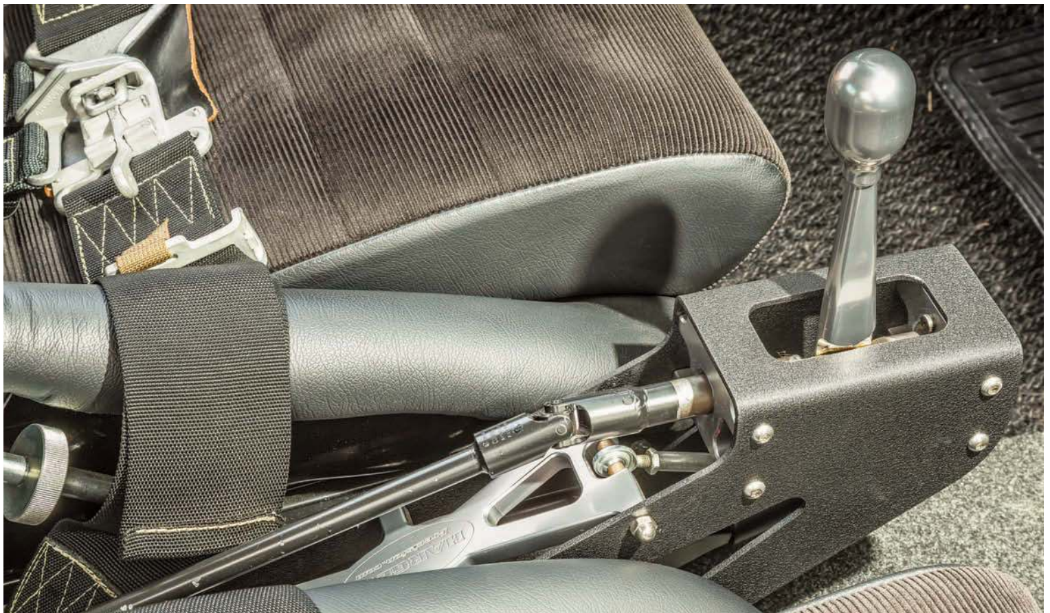
Above: Hargett shifter raises the gear lever, bringing it close to hand. Its rifle-bolt action makes for some slick gear changes
