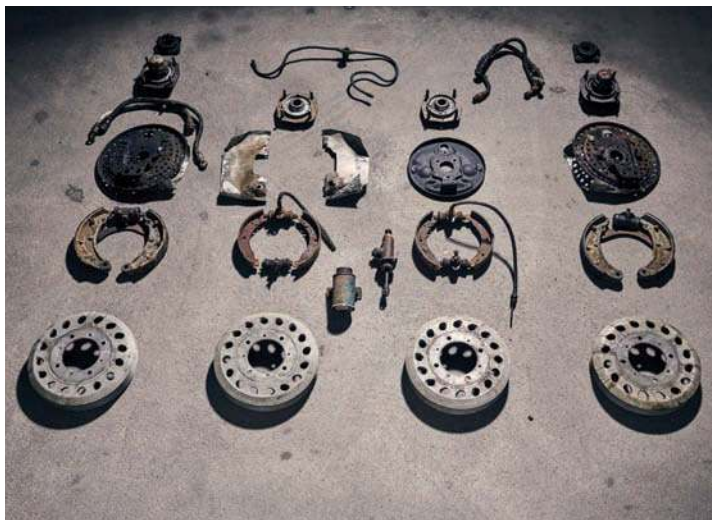
Above left: Ferry Porsche upgraded the brakes sometime in the immediate post-war period. During the 1990s rebuild, the Fiat braking system was replaced with VW components...
