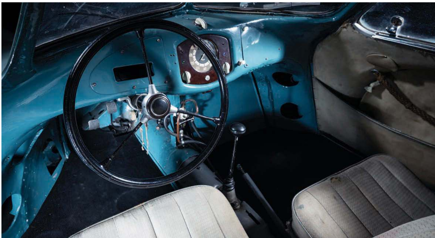
Below: KdF steering wheel, pedals and instrument pod hint at the car's origins. Note the fabric-covered doors to give extra elbow room – and to save weight
