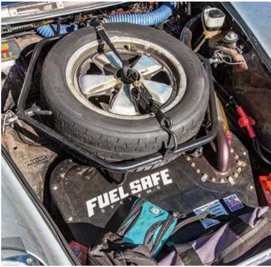
*Above left: Novel strut brace allows installation of spare wheel between strut towers – regular stowage space is taken up by the fuel cell*
