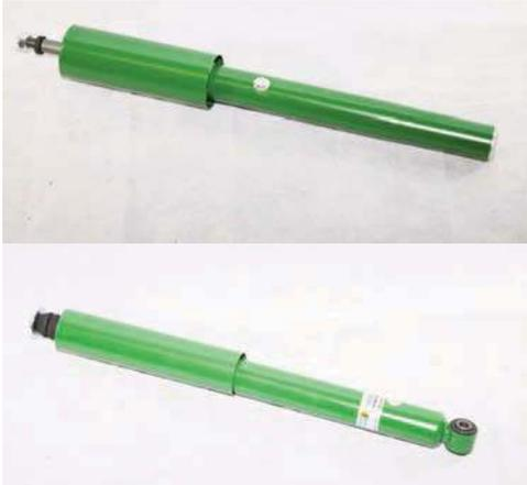
According to Bilstein, a shock absorber reduces and slows down vibrations of a car's springs, which is why it's referred to as a damper. The damper converts the kinetic energy by turning liquid friction into heat energy by slowing down the flow of oil inside the damper through valve passages. Incredibly, the damper can heat up to as much as 100–120°C.
