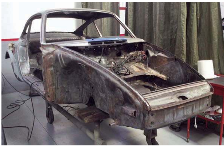
Above left: Once the bodyshell was stripped it was sent off to be acid-dipped
