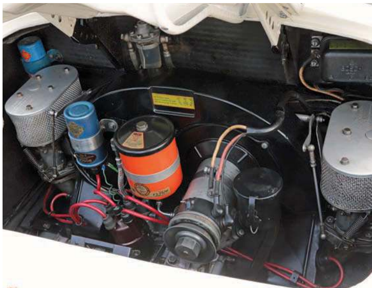
Above: Current engine is a 1500cc pushrod motor, fitted while the four-cam is away for a rebuild after holing number two piston
