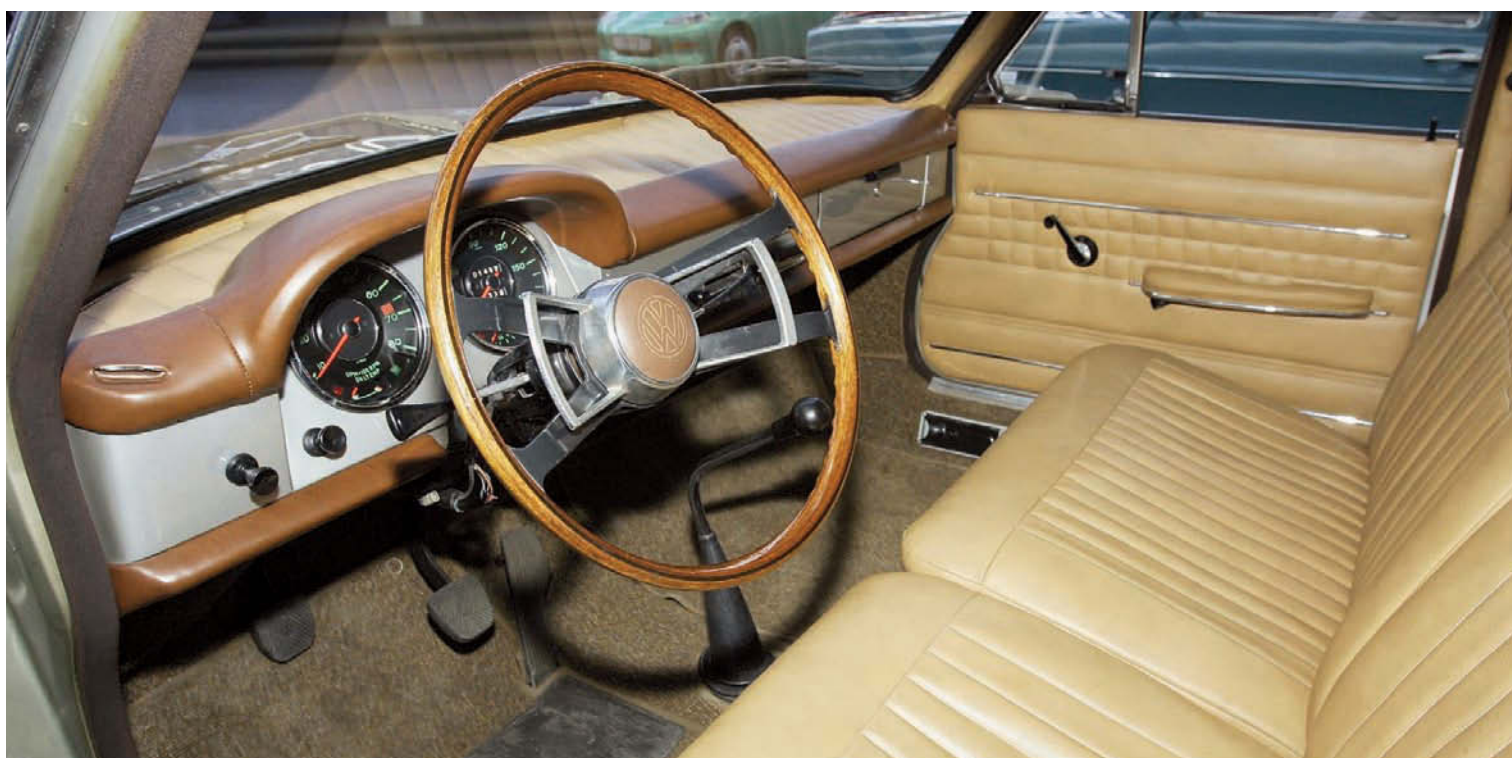
Below: Note the VW-logo'd Porsche steering wheel and the Porsche 911 heater vents in the sills
