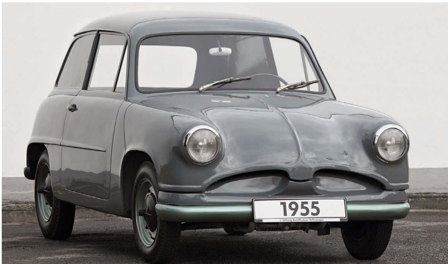
Above: The EA 48 was Volkswagen's first attempt at designing a small car off its own bat. Front-engined and with front-wheel-drive, it was very advanced for the time, but such projects proved time-consuming and were considered detrimental to the company profits
