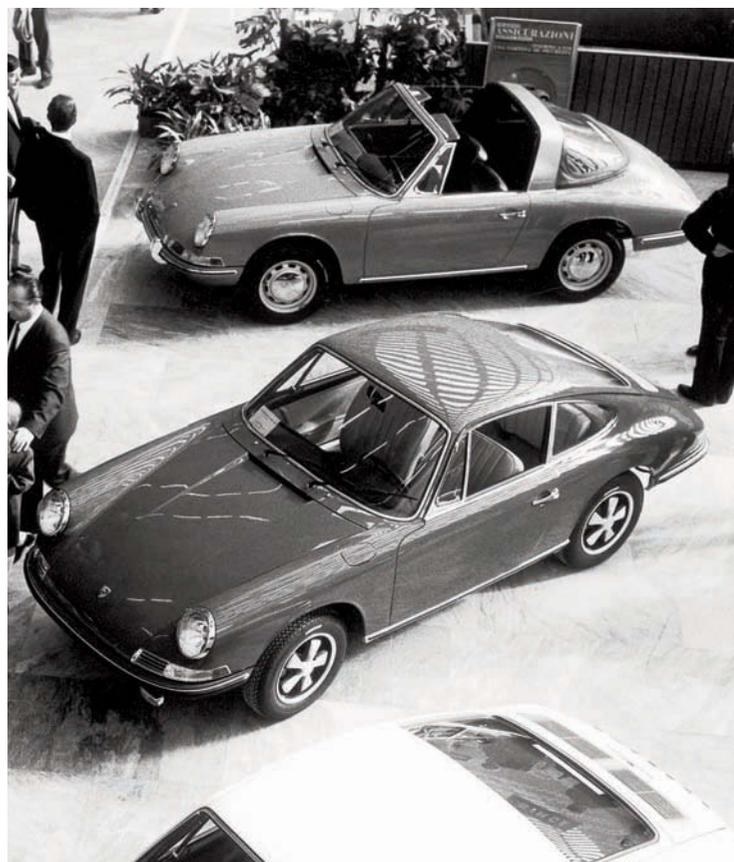
creating a bulge above the driver's head. The solution was to offer a single folding roof section of rubberised fabric, with scissor-action supports which could be clipped into place in the roll-bar and windscreen frame.
