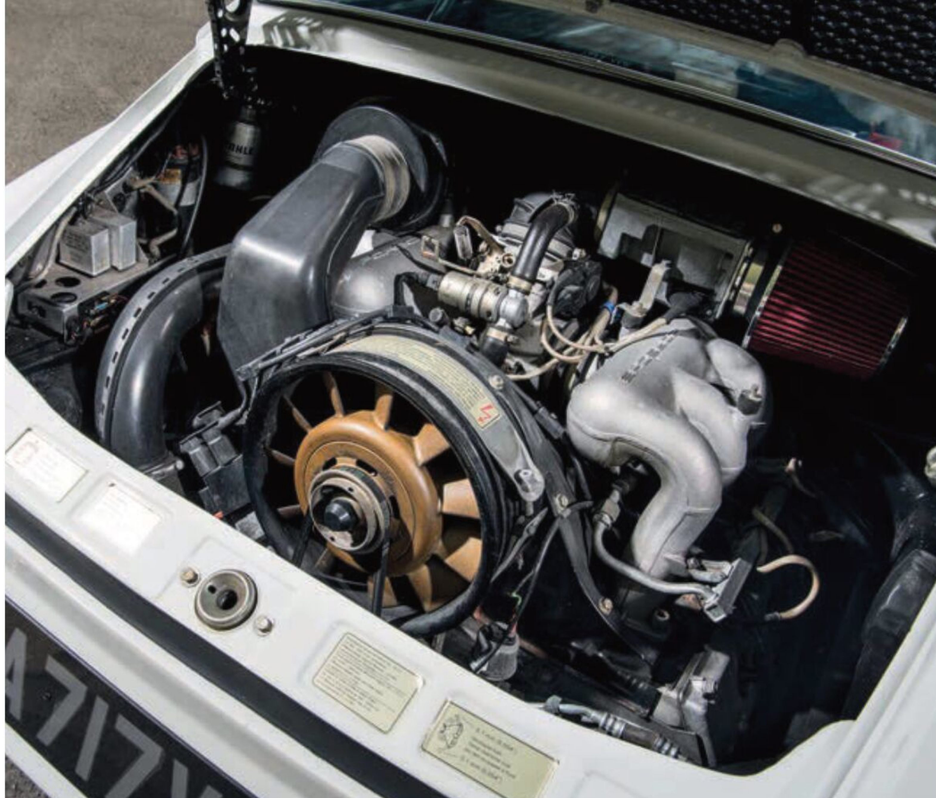
Above Original 3.2-litre lump lives at the car's rear end and delivers close to 240bhp
