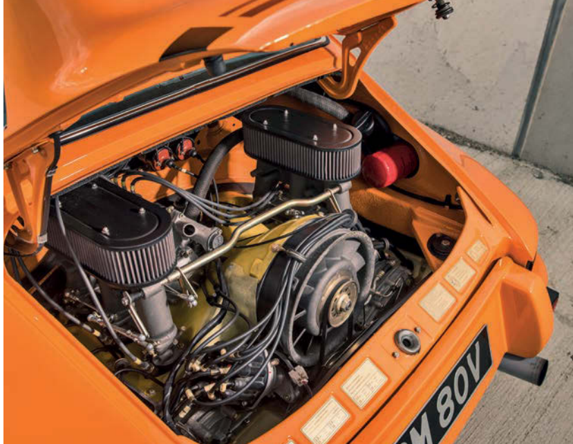
Above Potent 911 flat-six and a rare two-litre 906 engine equipped with fuel injection
